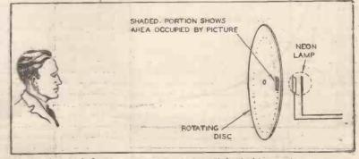
Fig. 9-Principle of simple scanning-disc television receiver
