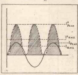
Showing how root-mean-square value of current is derived
