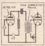
ing. A large self- Fig. 4-Use of transformer for capacity would in- tone correction
