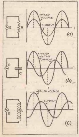
Current through a resistance (a) is in phase with the applied voltage; through a condenser (b) current is 90% ahead of voltage, and through an inductance (c) current lags 90% behind the applied voltage methods can be used, and there must obviously be some relation between the values obtained by the two methods.
