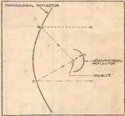
Fig. 2.—Illustrating the effect of the hemispherical reflector
