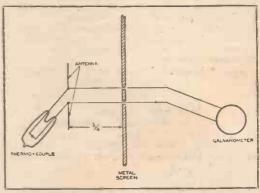
Fig. 3.—The wavemeter employed
