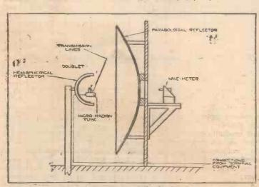
Fig. 1.—Arrangement of the transmitter
