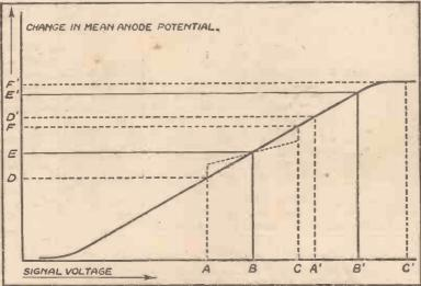
Fig. 2.—Rectification characteristic of a resistance-coupled detector valve
