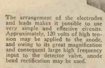
Fil. volts 6.0. Fil. current 0.25. Anode volts 120 max. The magnification factor and impedance vary between wide limits with changes of voltage on the electrodes, but the values under a typical set of conditions are as follows:
