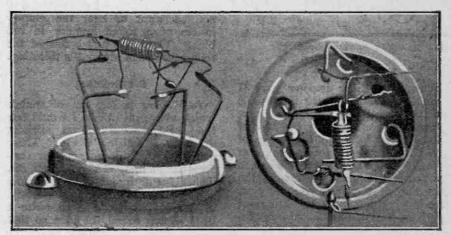
Showing the internal construction of the valve. The electrodes are arranged in the conventional manner.
