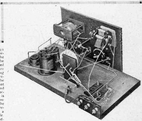
In order that the receiver may operate satisfactorily on short wavelengths the wiring must be well spaced out.
