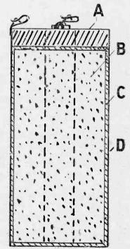
Fig. 2.—A similar type of cell to that shown in Fig. 1, in which C is a wrapping of porous paper.
