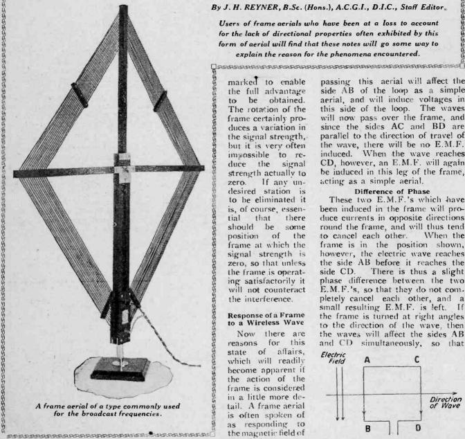
7 1TH the increasing use of super-heterodyne receivers and other forms of portable sets, frame aerials have recently come into prominence for amateur receiving equipment. One of the advantages which is claimed for the use of the frame aerial is that the directional effect may be utilised in reducing interference from unwanted stations.
