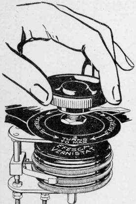
The Efesca Vernistat (Patent) is the most delicate filament control vet invented, and should be used wherever a separate rhetostat is employed for H.F. and detector valves. The Vernistat is smooth and silent in operation, and absolutely safeguards the valves from an accidental burn-out through too rapid switching on, Three complete turns
