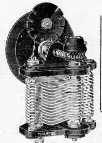
Little experience is necessary upon any such super-sensitive circuits as the short wave side of the Super-Heterodyne or capacity-reaction circuits to self-demonstrate that distant work is an impossible pastime without a mechanical fine tuning device operating on the condenser.
