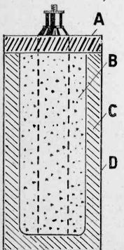
Fig. 1.—Here A is the sealing, B the carbon compound, C plaster of Paris, and D the zinc container.
