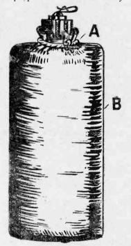
Fig. 3.—Showing how the carbon compound block may be tied up in a piece of cloth.
