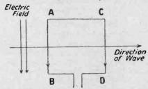
Fig. 1.-When the frame is in the plane of the wave there is a maximum phase difference between the E.M.F.'s in AB and CD.
