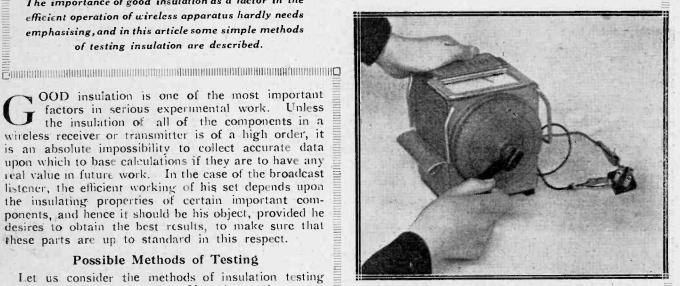
The instrument used by the author in making some of the insulation tests described is of the "Meg" type shown here.
