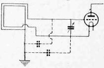
Fig. 4.—Earthing the middle point of the frame eliminates the aerial effect.
