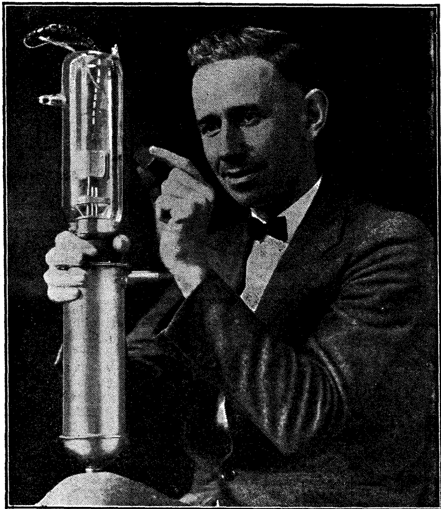
By means of a quartz crystal, shown with a high-power transmitting valve for a comparison of the sizes, the frequency of a transmitting station may be accurately controlled.
