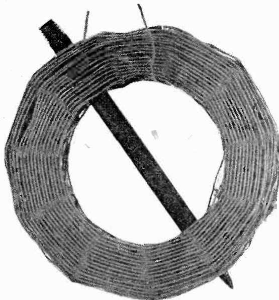
An ebonite rod pushed through the windings of a spider-web coil can be screwed or plugged into a hole in the panel or a conventional plug-in coil mount.
