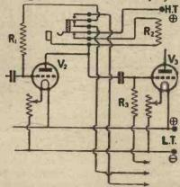
Fig. 2.—Using a jack to change gridbias with H.T. voltage.
