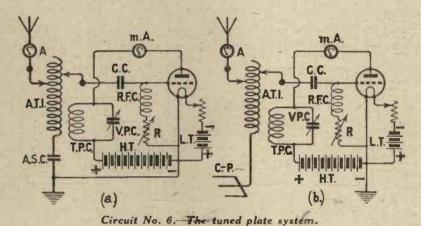
TRANSMITTING CIRCUIT No. 6. Tuned Plate System.
