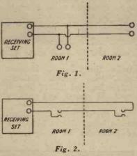
Showing two methods for wiring distant loud-speakers.
