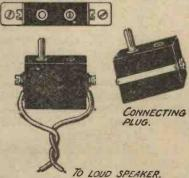
Fig. 3.—A suggested wall plug arrangement.
