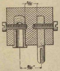
Fig. 1.—A section of a coil socket showing the construction.
