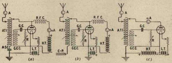
Circuit No. 3.—The magnetic reaction system.
