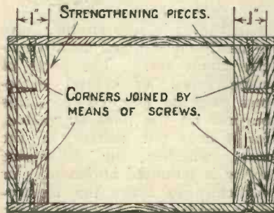
The constructional details of a home-made cabinet.
