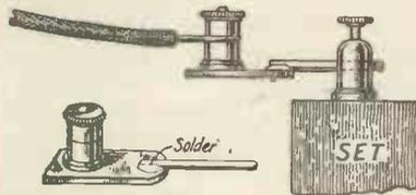
Fig. 3.—An adapter for use with telephone terminals.
