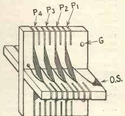
Fig. 4.—The secondary winding completed.
