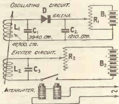
Fig. 4.—Simplified arrangement of the basic circuit developed by Dr. Eccles in 1910.
