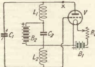
Fig. 30.—A single circuit oscillator using two separate inductances in series.
