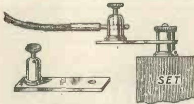
Fig. 2.—A suggested arrangement for screw-down terminals and rod-shaped tags.
