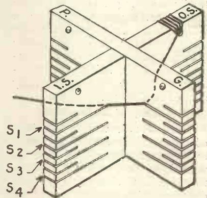
Fig. 3.—Commencing the secondary winding.
