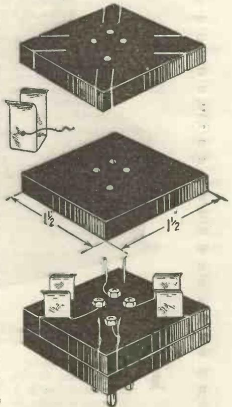
Fig. 6.—The separate parts and assembled adaptor.
