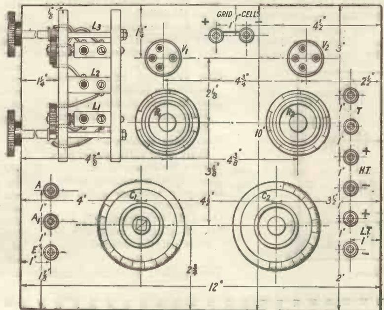
Fig. 4.—The panel layout. Blueprint No. 83a.
