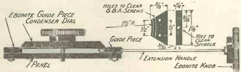
Constructional details of the extension handle and its guides.
