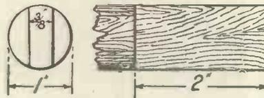
Fig. 9.—Constructional details of the turning handle.
