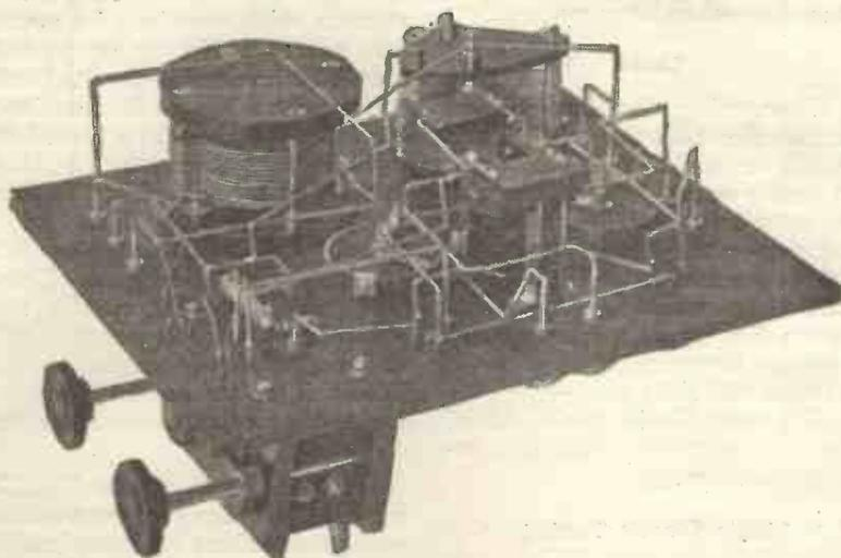
Fig. 7.—The well-spaced wiring of the receiver may be seen from this photograph.
