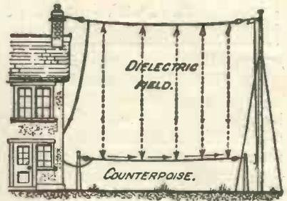
Fig. 2.—The effect of insulated counterpoise.
