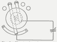
Fig. 3.—Showing how the two arms of the switch are connected.
