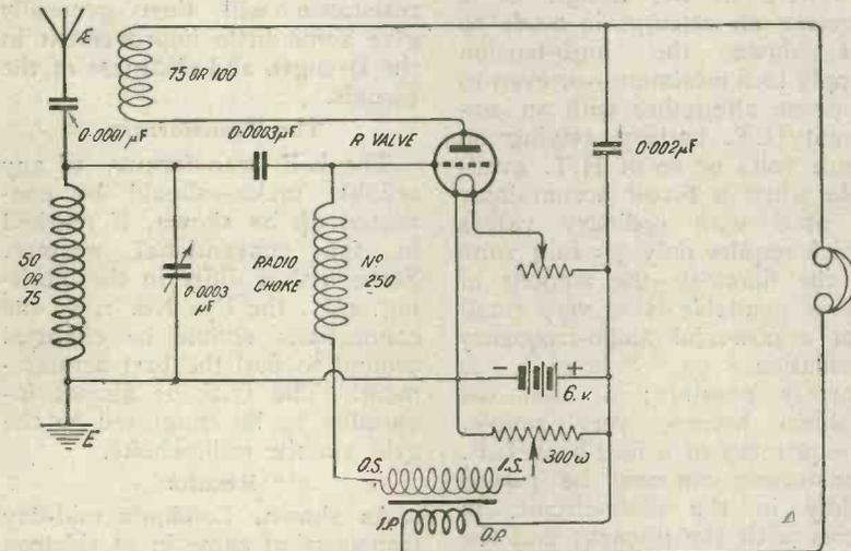
Fig. 1.—The new circuit. It will work just as well with a .06 dull emitter as with an R valve.
