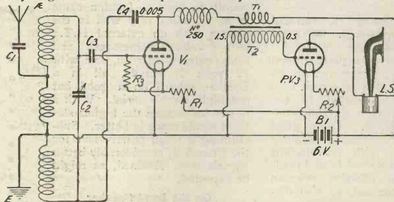
Fig. 6.—With this circuit a loud speaker was operated without H.T. C1 has a value of .00025 μF.
