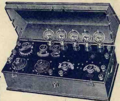
Five valve set in case, with cover not interfering with valves or leads. Wavelength range 300-4,000 metres. PRICE £31:5:0
