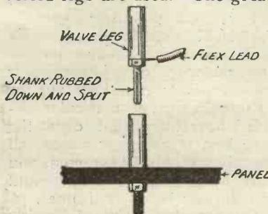
Fig. 1.—A quick method of connecting by means of valve legs.
