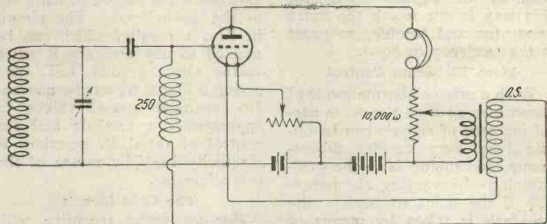
Fig. 2.—The potentiometer method of applying audio-frequency reaction.
