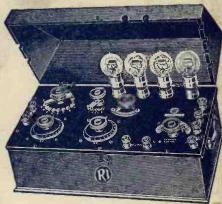
Four valve set in case, with cover not interfering with valves or leads. Wavelength range 300-4,000 metres. PRICE £26:0:0
