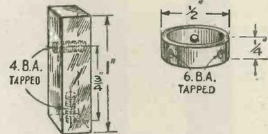
Fig. 3.—Dimensions of crystal holder and shaft support.
