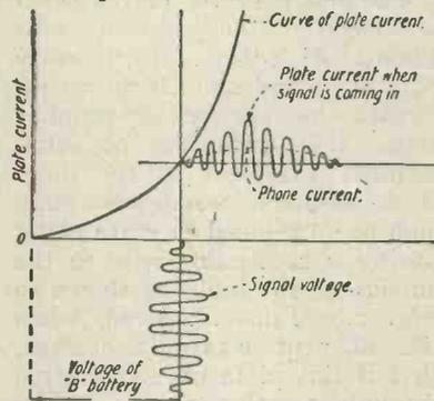
Fig. 5.—Curves illustrating the relation of plate to phone current in the reception of spark signals.
