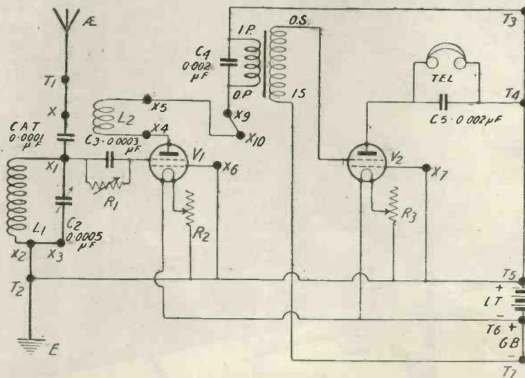
Fig. 4.—Showing the high-tensionless circuit using two valves. Constant aerial tuning is employed.
