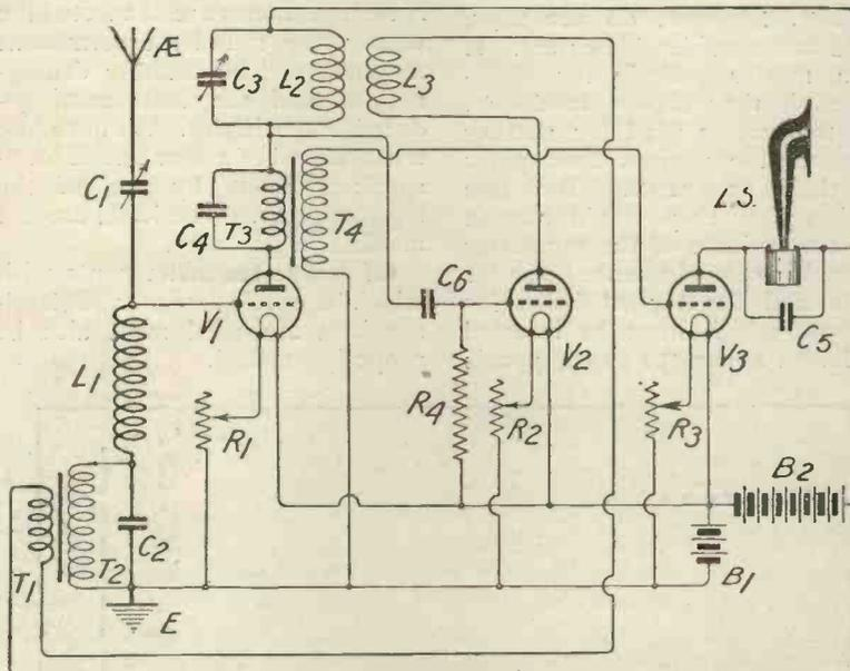
Fig. 1.—The ST76 circuit. The transformer T<sub>3</sub> T<sub>4</sub> is at high-frequency potential to earth.
