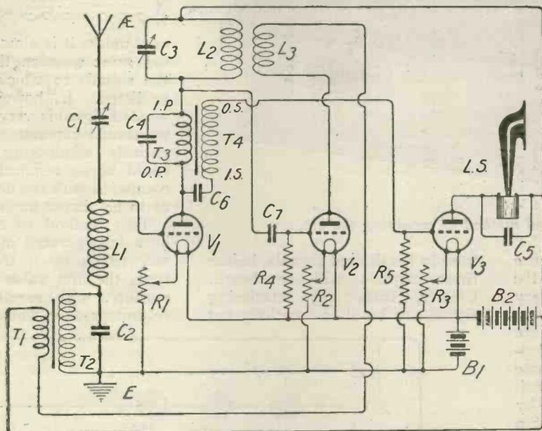
Fig. 3.—The ST76 circuit, with the Simpson connection of the low-frequency transformer incorporated.
