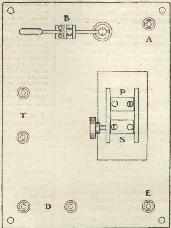
Fig. 2b.—Top-of-panel arrangement of loose-coupled set.
