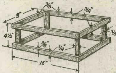
Fig. 9.—Details of the framework.
