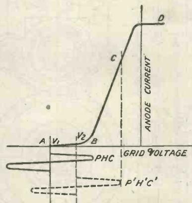
Fig. 49.—A diagram to explain the operation of the Fig. 48 circuit.
