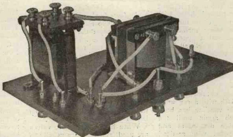
*Fig. 2.—Note that the transformers are arranged at right angles.*
