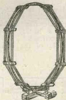
Fig. 4.—The general appearance of the frame aerial.
