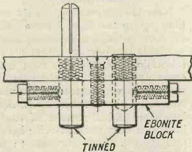
Fig. 1.—A suggested method of mounting coil sockets.
