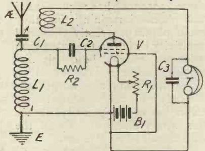
Fig. 3.—A circuit using a double grid valve.
