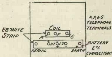
Fig. 2.—Back of cabinet of two-valve receiver used in the test.
