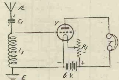
Fig. 4.—The "Sodion" valve circuit.
