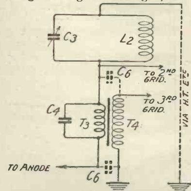
Fig. 2.—Potentials across L<sub>2</sub> C<sub>3</sub> are limited owing to each end of the circuit being at earth potential.
