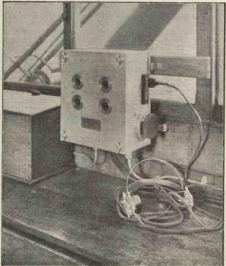
The "Marconi" beam receiver mounted on the bridge of a ship.
