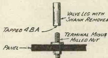
Fig. 2.—Another method, using valve legs and terminals.
