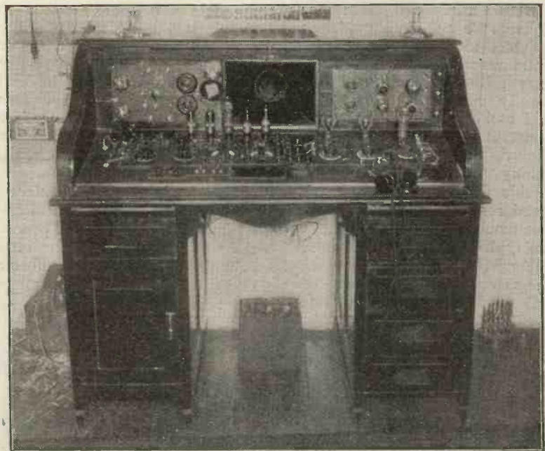
The reader who built this receiver was obviously anxious to have everything to hand. Note the built-in loud speaker. There are twelve valves in sight!
