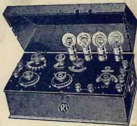
Four valve set in case, with cover not interfering with valves or leads. Wavelength range 300-4,000 metres. PRICE £26:0:0 B.B.C. Tax £1:5:0
