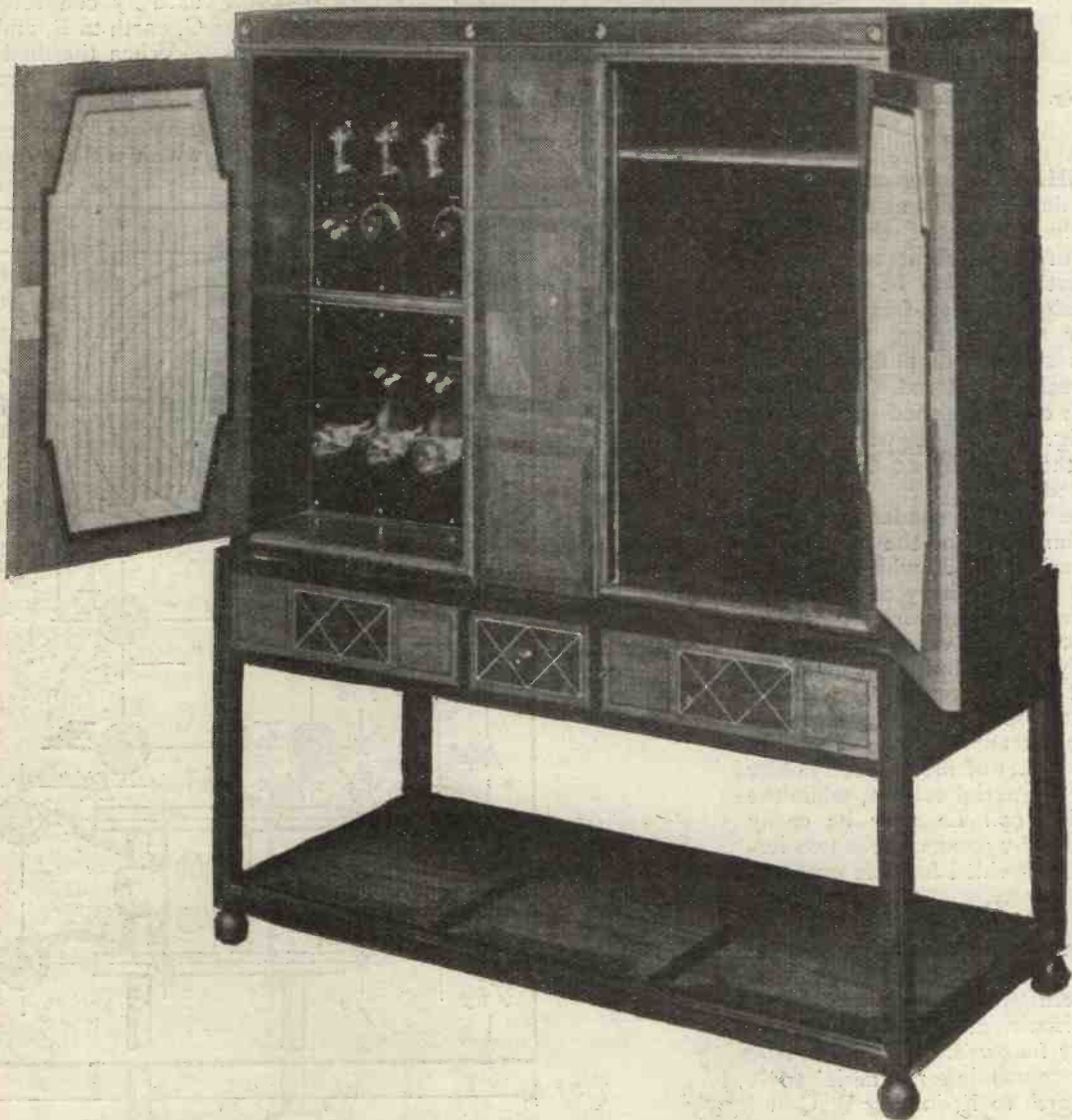
Our photograph shows the cabinet wireless receiver just installed at Buckingham Palace for the use of His Majesty the King. It is self-contained, with batteries, loud speaker, and aerial in one cabinet. Fuller particulars are given on our editorial page.
