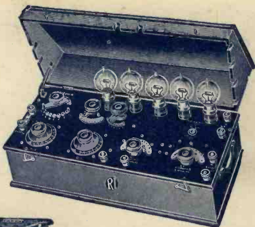
Five valve set in case, with cover not interfering with valves or leads. Wavelength range 300-4,000 metres. PRICE £31:5:0 B.B.C. Tax £1:10:0
