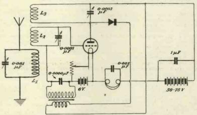
A modified arrangement of the circuit appearing in "Modern Wireless" No. 2, page 88, Fig. 4. L<sub>1</sub> 50 turns, duolateral; L<sub>2</sub> 35 turns, duolateral; L<sub>3</sub> 75 turns, duolateral.
