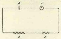
Fig. 2 .- Rough method of measuring a resistance.
