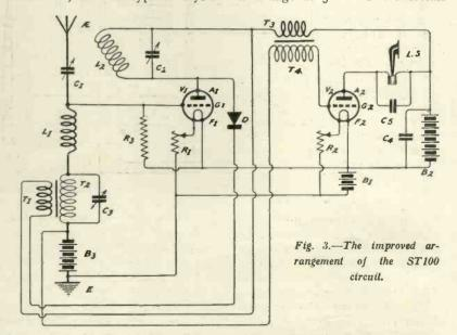
was found to be Galena, with a fine metal point resting on it. The importance of the detector not only lies in its actual rectifying properties, but also on its impedance.
