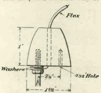
Fig. 8.—Delails for contact pin.
