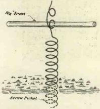
Fig. 11.—Showing the method of using a screw pickel
