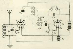
Fig. 2.—The same method of reaction applied to a highfrequency valve.
