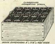
Fig. 9.—The H.T. battery in box with lid removed.
