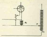
Fig. 2 .- Method showing how the H.T. ballery may be used for providing negative potential to the grid.
