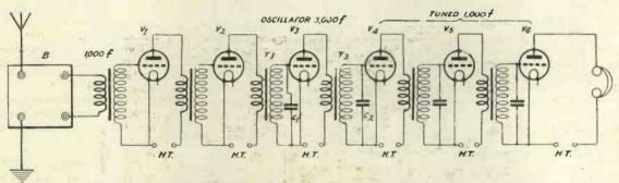
Illustrating the principle of the eliminating circuit; B being the usual receiving apparatus.
