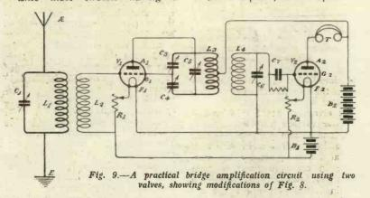
maximum sensitivity and selectivity, those employing this bridge method of amplification are by no means simple to operate. Both manipulative skill and a full knowcoils close together. The best arrangement is to lay them out on a table or on a board.
