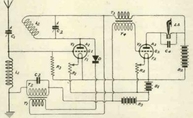
Fig. 1.—The original ST100 circuit with grid cells added at B3.
