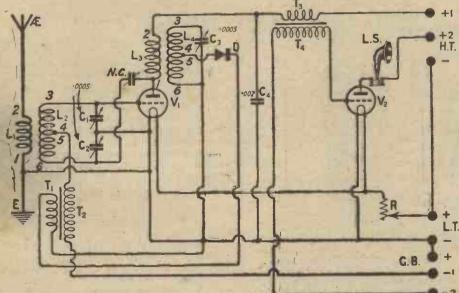
Fig. 3.—The condensers C1 and C2, form the dual condenser and both are operated by one knob.
