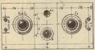
Fig. 1.—Symmetry is the keynote of the panel layout, full dimensions of w ich can be obtained from this diagram. Blue Print No. W2009A.
