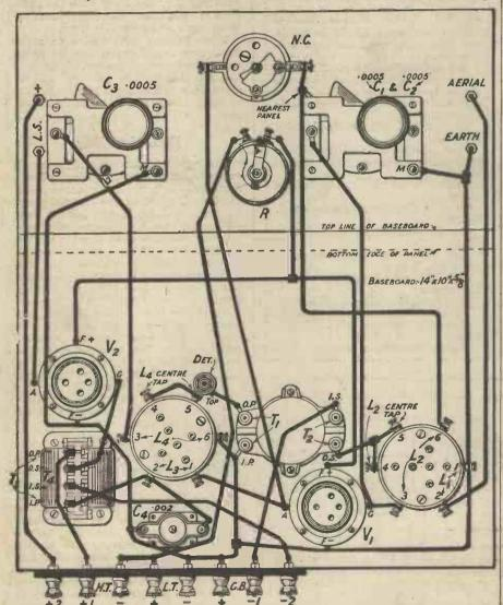
Fig. 2.—The wiring instructions given in the next column should be used in conjunction with this wiring diagram. Free Blue Print W2009B.
