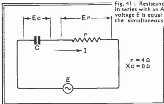
Fig. 41 : Resistance and capacitive reactance in series with an A.C. source. The generator-voltage  $E$  is equal to the total voltage due to the simultaneous presence of  $E_c$  and  $E_r$ . See Fig. 42
