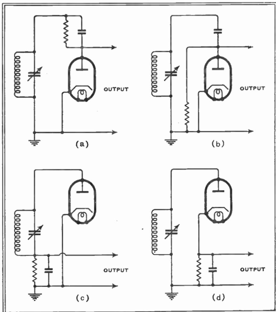
Fig. 85 : Various methods of connecting a diode detector to a tuned circuit
