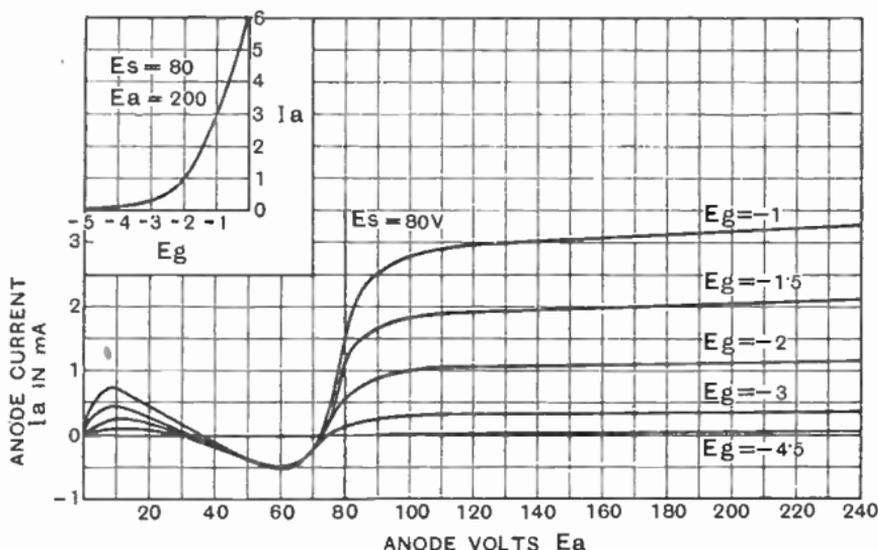
Fig. 105: Characteristic curves of typical screened tetrode. Only the flat parts of the curves to the right of the line  $E_s$  are used for amplification.
