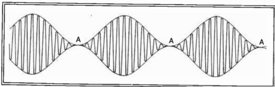
Fig. 73: Carrier-wave modulated to a depth of 100%. At its minima (points A) the R.F. current just drops to zero; any attempt at still deeper modulation results in a series of separate bursts of current, and the envelope no longer has the form of the modulating wave
