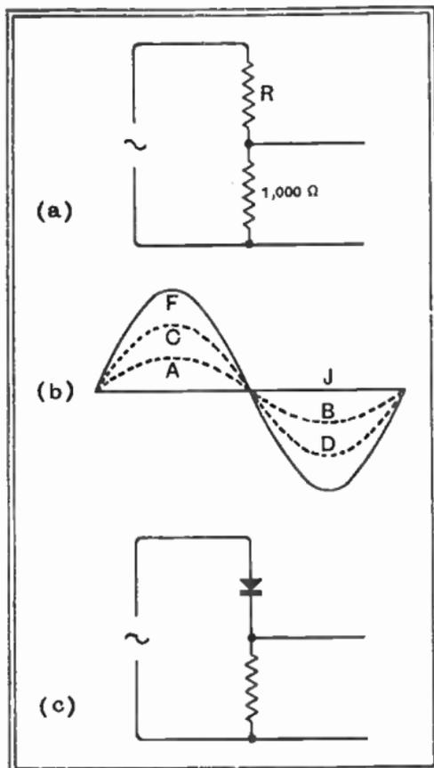
Fig. 77 : The results of applying a sine wave voltage to resistances represented by Fig. 76, in the circuit shown here at a, are indicated by b, which is lettered to correspond with the various characteristics in Fig. 76. When  $R$  is a rectifier, it is represented by the symbol shown in c
