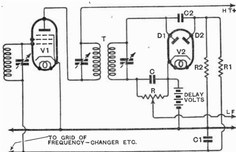
Fig. 149 : Modification of Fig. 147 to produce delayed A.V.C. Until the peak voltage of the signal exceeds the positive bias on the cathode of  $V_2$ , the A.V.C. system does not begin to operate
