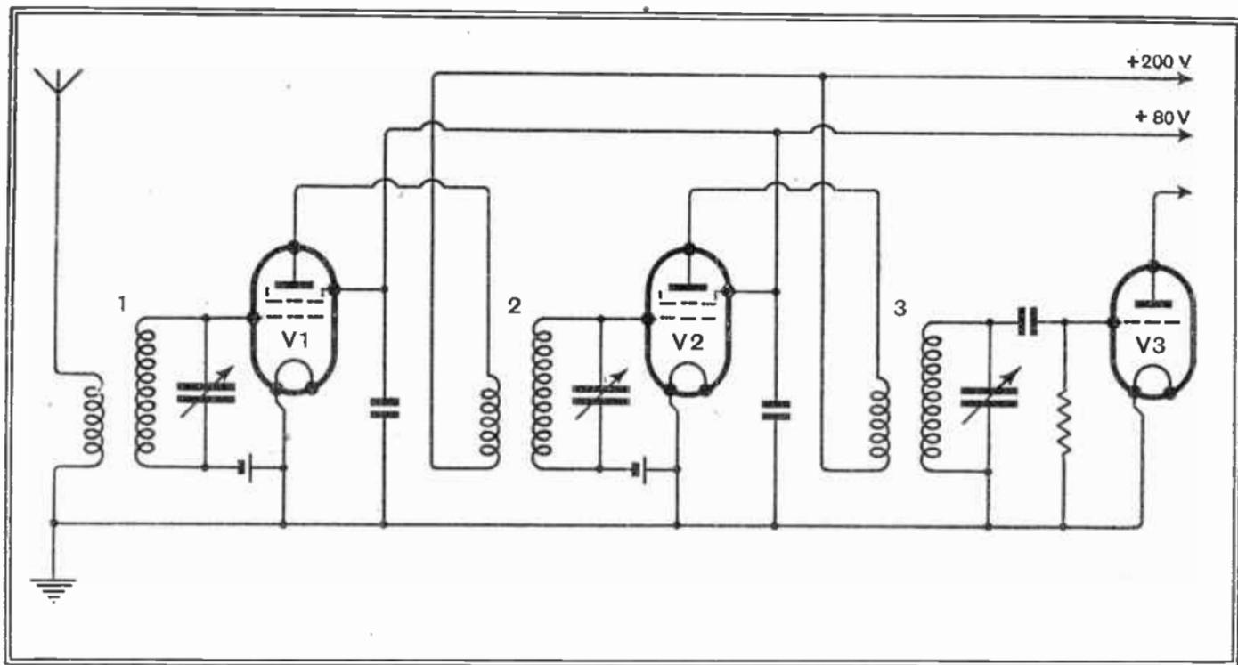
Fig. 108 : Two-stage radio-frequency amplifier, using step-up transformer couplings with screen grid valves. Much more stable than the closely-corresponding circuit of Fig. 107
