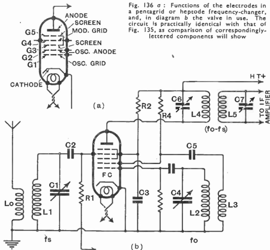
Fig. 136 a : Functions of the electrodes in a pentagrid or heptode frequency-changer, and, in diagram b the valve in use. The circuit is practically identical with that of Fig. 135, as comparison of correspondingly-lettered components will show
