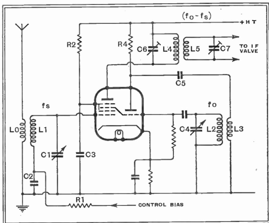
Fig. 137 : Typical triode-hexode frequency-changer circuit, lettered to correspond with Figs. 135 and 136b
