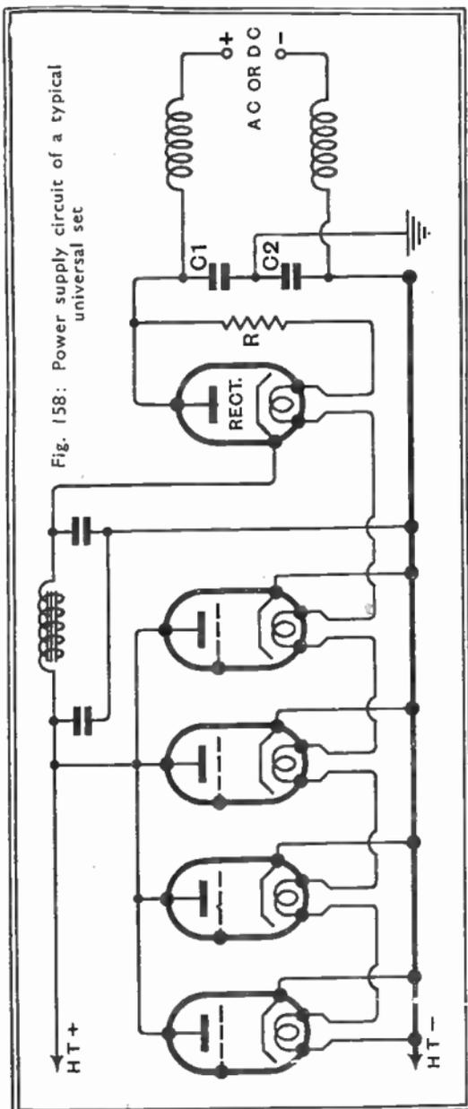
Fig. 158: Power supply circuit of a typical universal set
