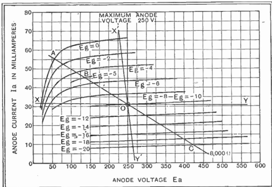
Fig. 123 : Curves of a typical indirectly heated output pentode. The load-line ABOC represents a usual load. Curves taken at  $E_s = 200$
