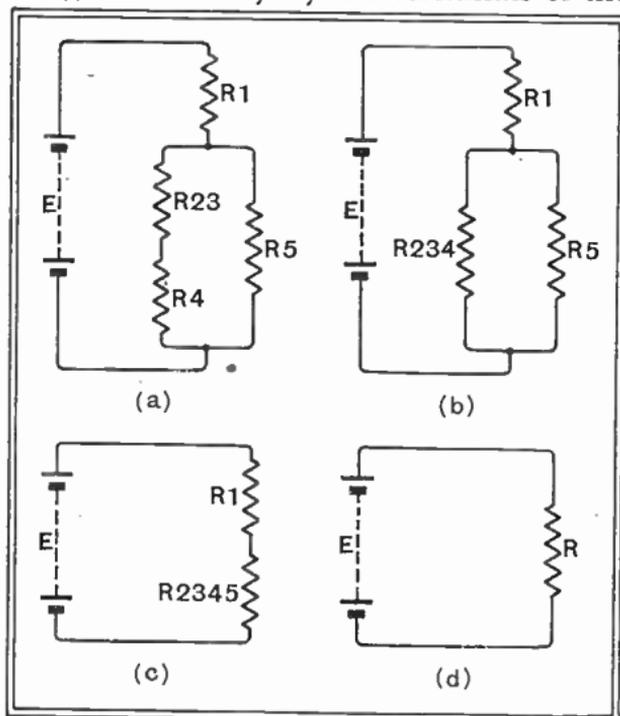
Fig. 11: Successive stages in simplifying the circuit of Fig. 10.  $R_{23}$  stands for the single resistances equivalent to  $R_2$  and  $R_3$ ;  $R_{234}$  to that equivalent to  $R_2$ ,  $R_3$  and  $R_4$ , and so on.  $R$  represents the whole system
