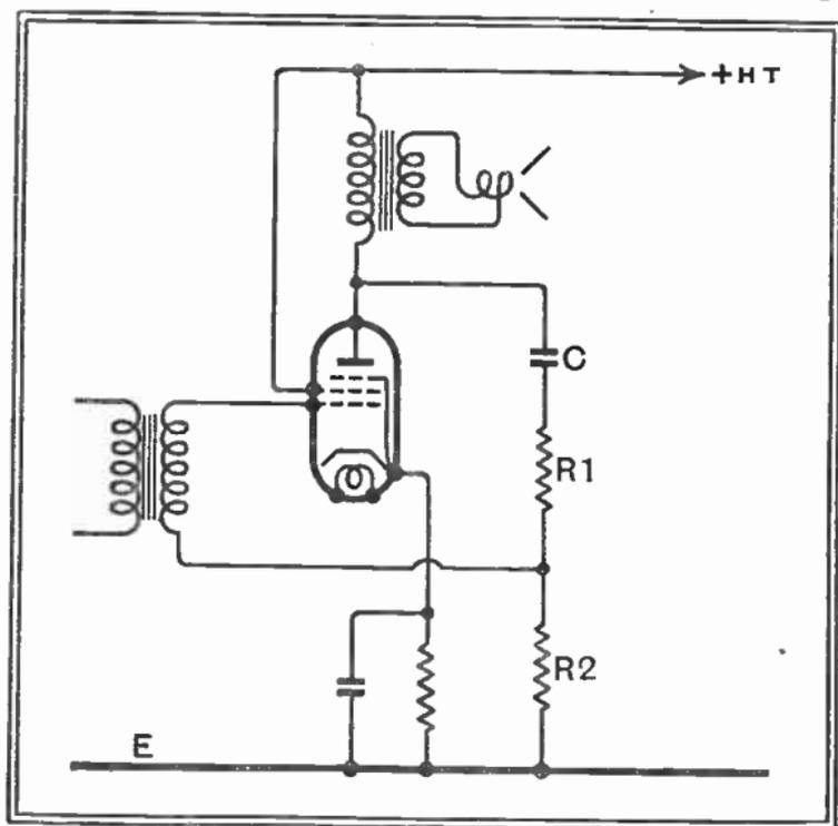
Fig. 128 : Circuit for negative feedback.  $R_1$  and  $R_2$  form a potential divider across the output, the voltage developed across  $R_2$  being fed back into the grid-circuit in series with the transformer secondary.
