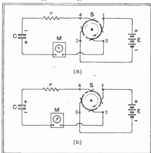
Fig. 30: Condenser and battery, with rotating reversing switch. The behaviour of this circuit leads directly to the properties of capacitance in an A.C. circuit
