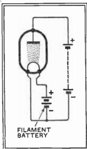
Fig. 59 : A directly heated (battery) diode valve
