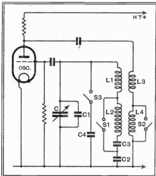
cause the required ratio of maximum to minimum capacitance is different. This difference, however, can readily be adjusted by putting a fixed capacitance either in parallel with the oscillator condenser to increase the minimum capacitance, or in series to
