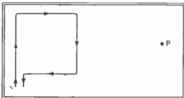
Fig. 161 : From the point of view of the reader, the radiation due to different parts of a turn of wire carrying oscillatory current cancels out. Towards the point P, however, the different distances of the vertical sides of the square result in net radiation
