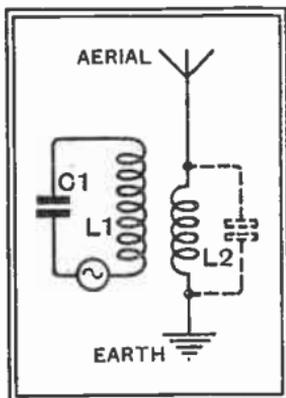
Fig. 70 : Schematic diagram showing how a wireless wave originates at the transmitting station. The coil  $L_1$  is tuned by the capacitance (shown in dotted lines) existing between the aerial wire and the ground beneath it
