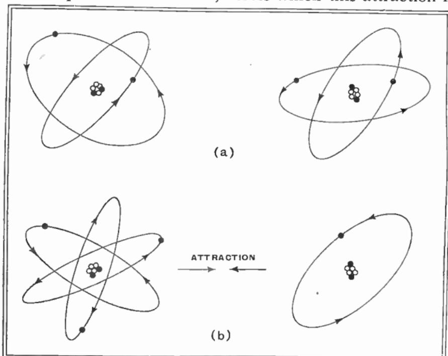
Fig. 5 : Diagram showing (a) imagined structure of two neutral atoms, each containing the same number of protons (white) and electrons (black), which cancel out so far as electrical effects are concerned. (b) shows the same two atoms after one has gained an electron at the expense of the other, and they now show electrical attraction. Two atoms, both with a surplus or a deficiency of electrons, repel one another
