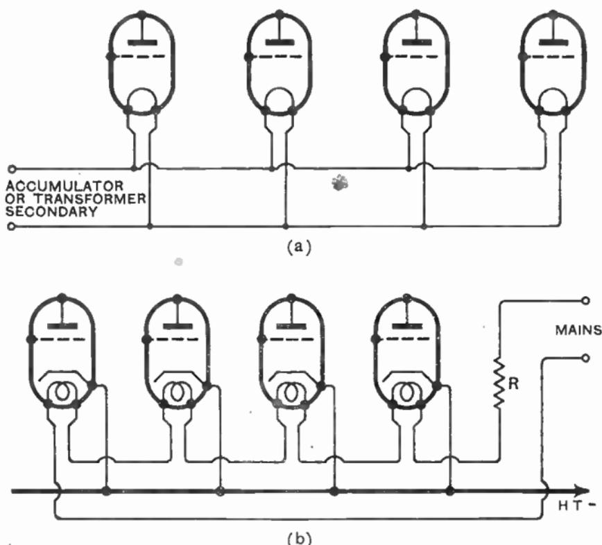
Fig. 153 : Diagram a shows method of heating filaments of battery valves or heaters of A.C. valves in a 4-valve set. All valves require the same voltage. In diagram b, which shows D.C. or universal valves with heaters in series, all take the same current. Note that in spite of different potentials of heaters all cathodes can be joined to H.T. —
