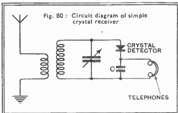
Fig. 80 : Circuit diagram of simple crystal receiver
