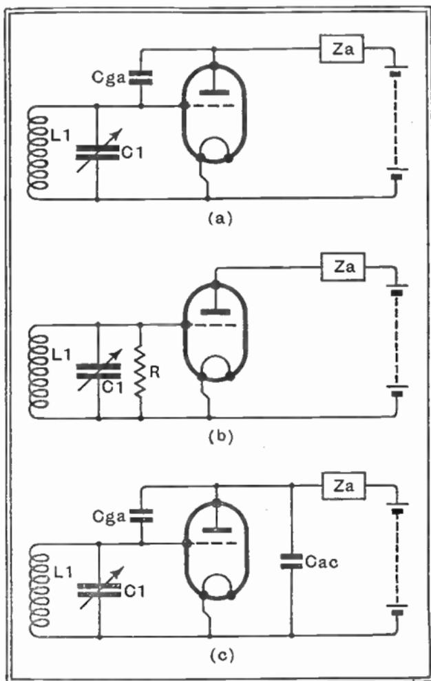
Fig. 95 : Illustrating the Miller Effect. *a* A voltage at the anode of a valve can pass, by way of  $C_{ga}$ , back into the grid circuit. *b* If  $Z_a$  is a capacitance, the anode-grid feed is equivalent to connecting a damping resistance  $R$  across the grid circuit. *c* Owing to the stray capacitances from anode to cathode, any anode-circuit impedance  $Z_a$  is necessarily shunted by  $C_{acc}$
