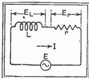
Fig. 43 : Resistance and inductive reactance in series with a source of A.C. voltage. Compare with Fig. 41 and the curve of Fig. 42
