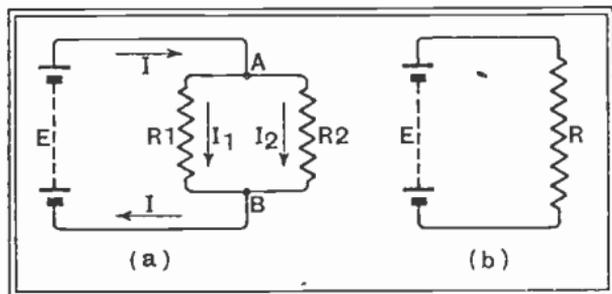
Fig. 9 : Resistances in parallel. The circuit b is equivalent to the circuit a in the sense that both take the same current from the battery E, if  $1/R = 1/R_1 + 1/R_2$ .
