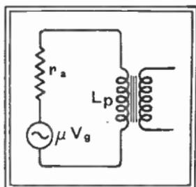
Fig. 120 : Equivalent anode circuit of a transformer-coupled stage
