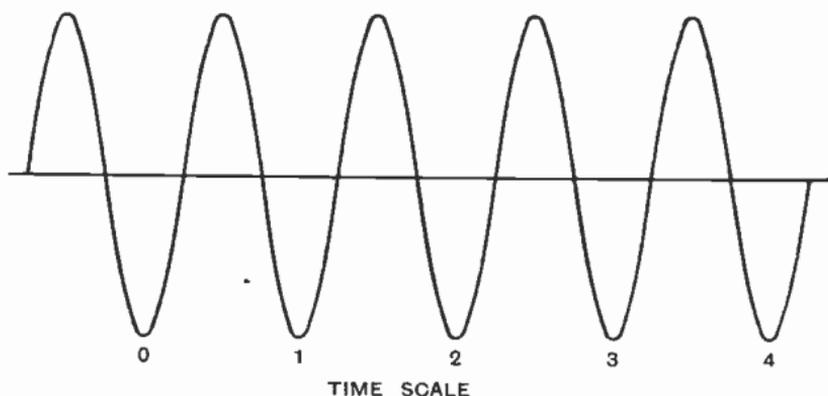
Fig. 71 : Curve representing rise and fall of current in  $L_1, C_1$  (Fig. 70), rise and fall of voltage on aerial, or rise and fall in strength of field due to radiation. If  $f = 1,000$  kc/s ( $\lambda = 300$  m.) the unit of time is one-millionth of a second
