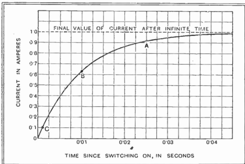
Fig. 35 : Showing slow rise of current in circuit of Fig. 34. Calculated for  $E = 100$  v,  $L = 1.0$  H,  $r = 100 \Omega$ . By sufficiently rapid rotation of the switch, the current could be kept below A ( $1/40$ th sec.), below B ( $1/100$ th sec.), or even below C ( $1/1,000$ th sec.)
