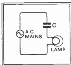
Fig. 32 : If a condenser of large capacitance ( $2 \mu\text{F}$  or more) is placed in series with a lamp lighted from A.C. mains, the lamp will light, though with less than normal brilliance
