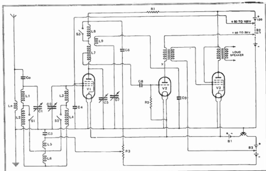
Fig. 132 : Complete circuit of three-valve set to conform with specification laid down in Section 148
