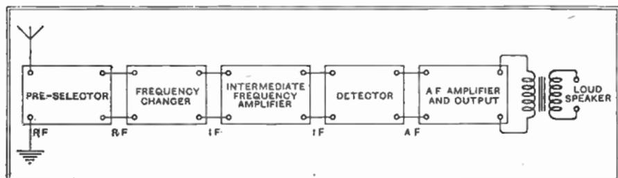
Fig. 133 : Schematic diagram of supersonic heterodyne receiver ("superhet.") showing the functions of the various parts and the changes in the signal in passing through it
