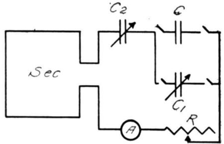
the movable-plate air condenser,  $C_1$ , and vary its capacity until the current,  $A$ , has a maximum value. Also vary the sliding resistance,  $R$ , until the current has the same value it has when the condenser,  $C$ , is used.
