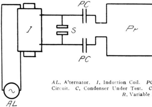
AL, Alternator. I, Induction Coil. PC, Primary Condenser. Pr, Primary Circuit. Sec, Secondary Circuit. C, Condenser Under Test.  $C_2$ , Adjustable Air Condenser.  $C_1$ , Adjustable Air Condenser. R, Variable Resistance. A, Hot Wire Ammeter.
