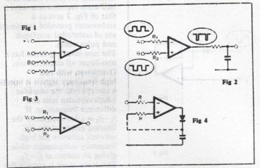
of the peak detector of Fig. 4. The capacitor charges through the diode until it matches the peak value of the input. Another application for the comparator is in coupling signals into and out of
