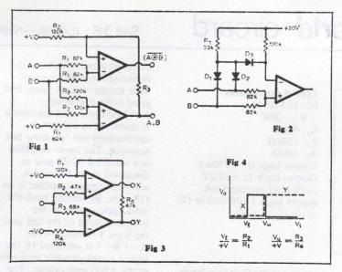
gate to go to logic 1 when both inputs are at logic 1, overriding the normal NOR gate function. The net result is that the output of the NOR gate becomes logic 1 for A=B and the circuit is an equality comparator. The output can also be seen as the negation of the exclusive-OR function.
