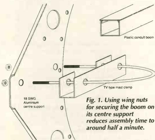
Fig. 1. Using wing nuts for securing the boom on its centre support reduces assembly time to around half a minute.
