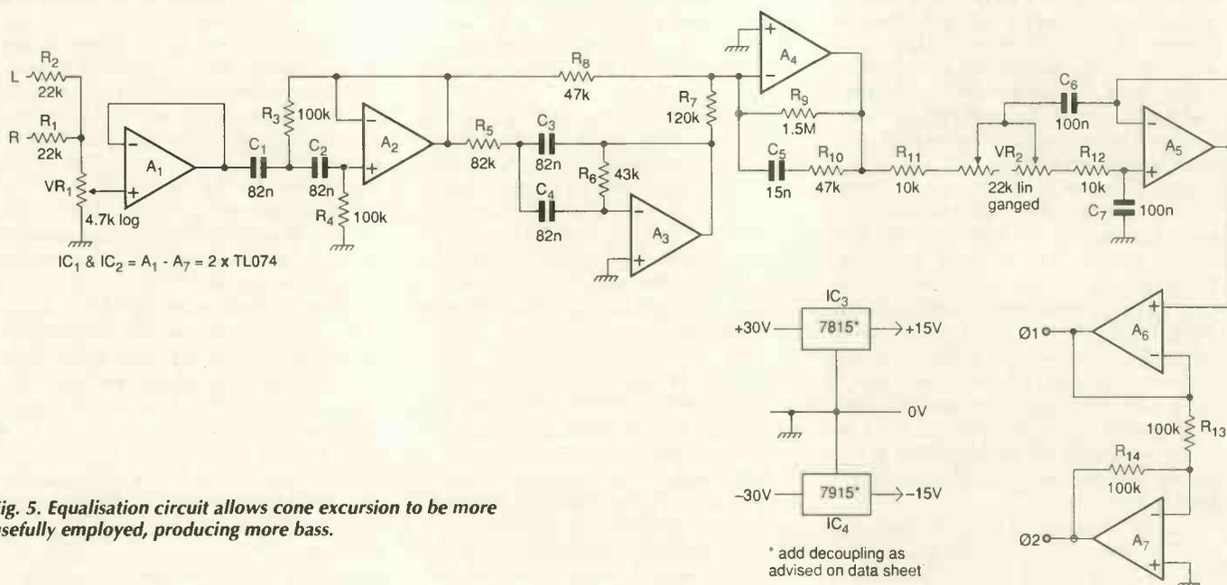
Fig. 5. Equalisation circuit allows cone excursion to be more usefully employed, producing more bass.
