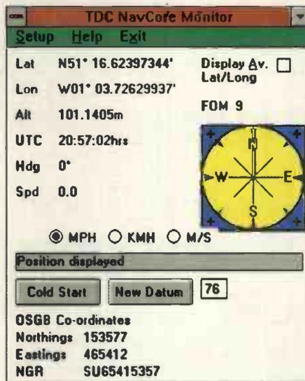
Fig. 3. Screen shot of industry standard NMEA reader program, also included in kit. Displays GPS information on a pc but also shows positions of satellites in the sky and a tracking display showing a history of your position.
