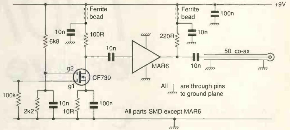
is intended for examining low-level rf signals and can be used with an input capacitor as small as 1pF. This forms a capacitive divider leading to a gain of about two – still useful.
