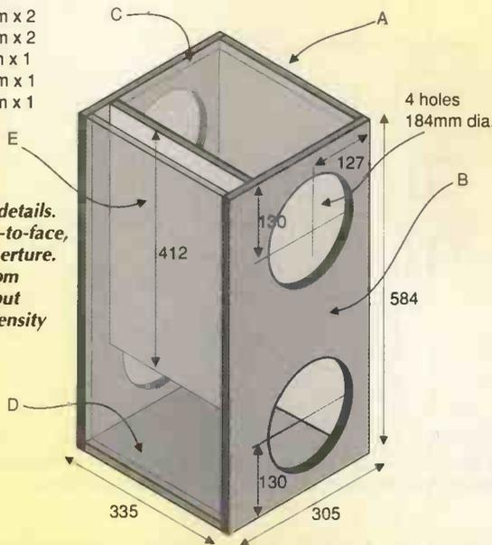
**Fig. 6. Enclosure details.** Two drivers, face-to-face, mount in each aperture. Prototype was from 15mm shelving, but 18mm medium density fibreboard is recommended.
