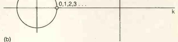
**2d. Complex digital phasor of frequency (pi+delta) radians per sample interval; aliasing due to undersampling.**
