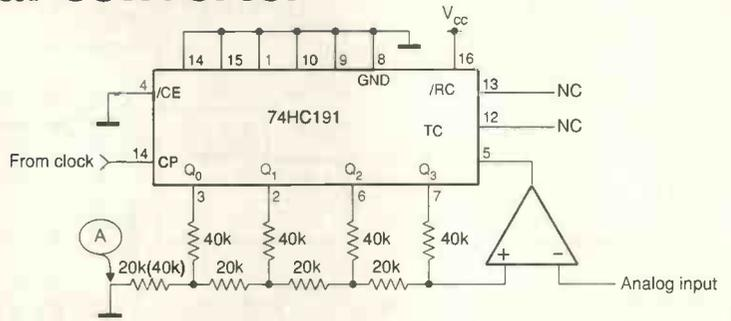
Up/down counter tracks analogue input to give a 4-bit a-to-d converter, convertible to give more bits.
