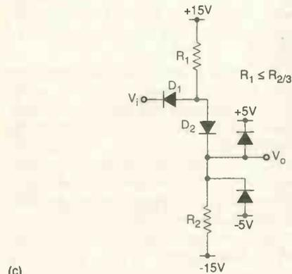
Fig. 2. Diode limiting (a) used in a circuit to measure the settling time of an op-amp. At (b) the LT1194 wideband op-amp circuit with voltage controlled symmetrical clipping level. Reproduced by courtesy of Linear Technology Corporation. Simple bounding circuit in (c) protects following stages from mains inputs.
