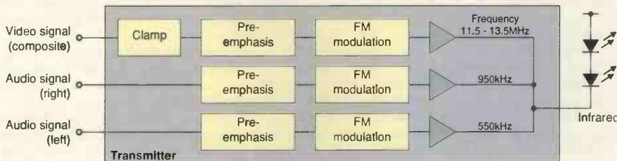
Transmitting and receiving systems of the camcorder one-way optical link. Both audio and video signals are transmitted.
