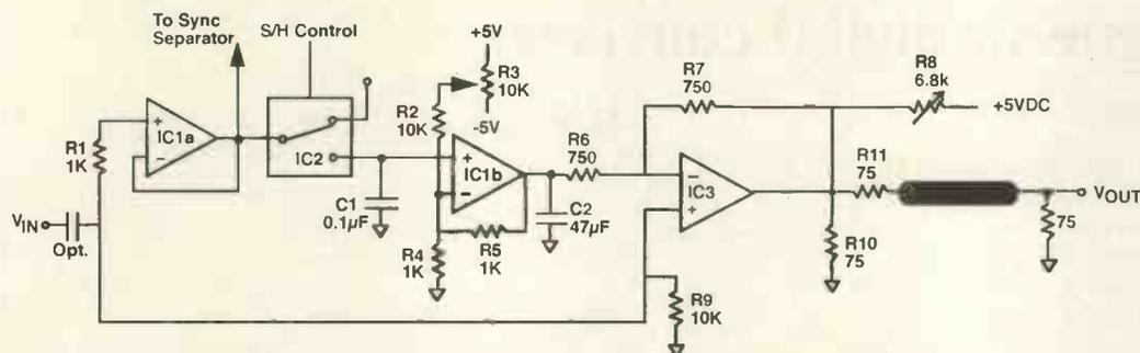
One of the benefits of this circuit is that by stripping off the sync from a video signal and digitising only the active information, better use is made of the a-to-d converter's resolution.
