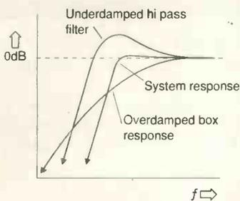
Fig. 2. Sixth-order alignment. System response is extended by an external filter.
