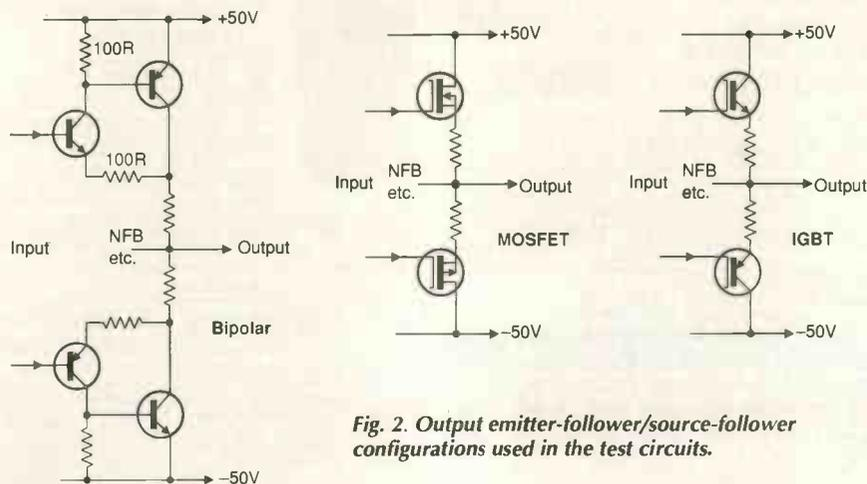
Fig. 2. Output emitter-follower/source-follower configurations used in the test circuits.
