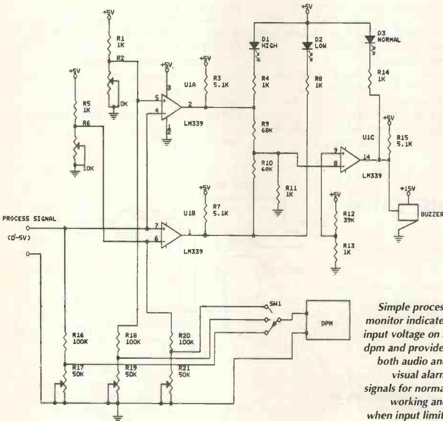
Simple process monitor indicates input voltage on a dpm and provides both audio and visual alarm signals for normal working and when input limits are exceeded.
