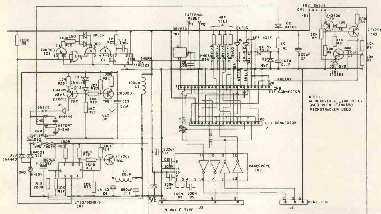
Fig. 1. Circuit diagram of the GPS receiver serial interface board and its power supply.
