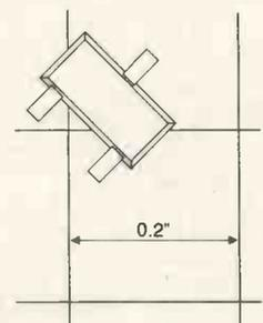
Producing square lands on one side of a double-sided pcb makes an excellent rf prototyping board for surface-mount devices.
