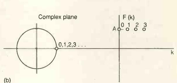
**2c. Complex digital phasor of frequency pi radians per sample, sampling at Nyquist frequency.**
