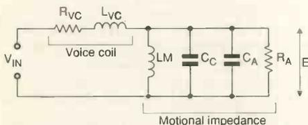
Equivalent circuit to speaker in sealed enclosure.
