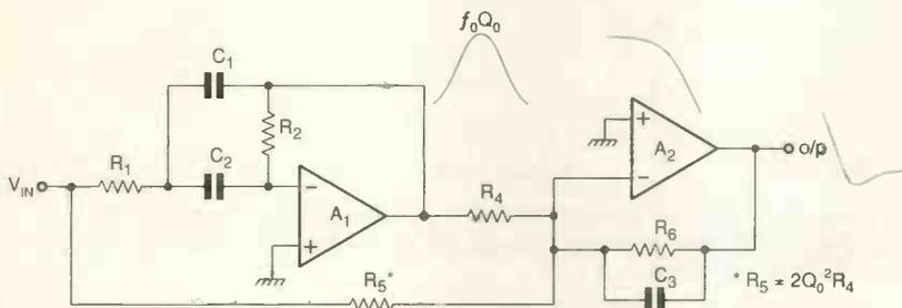
Fig. 3. Amplifier A<sub>1</sub>, with R<sub>1</sub>, R<sub>2</sub>, C<sub>1</sub> and C<sub>2</sub>, forms a bandpass filter with the same turnover frequency and Q as the speaker system. The required bandstop response is obtained by subtracting the bandpass from the input by A<sub>2</sub>. Capacitor C<sub>3</sub> and R<sub>6</sub> produce an integrator response to produce equalisation.
