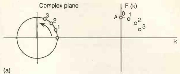
**2b. Complex digital phasor of frequency zero radians per sample interval (dc sampling).**
