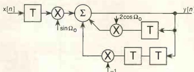
Fig. 4. System diagram of a digital resonator. The frequency of oscillation is controlled by the parameter  $\Omega_0$ .
