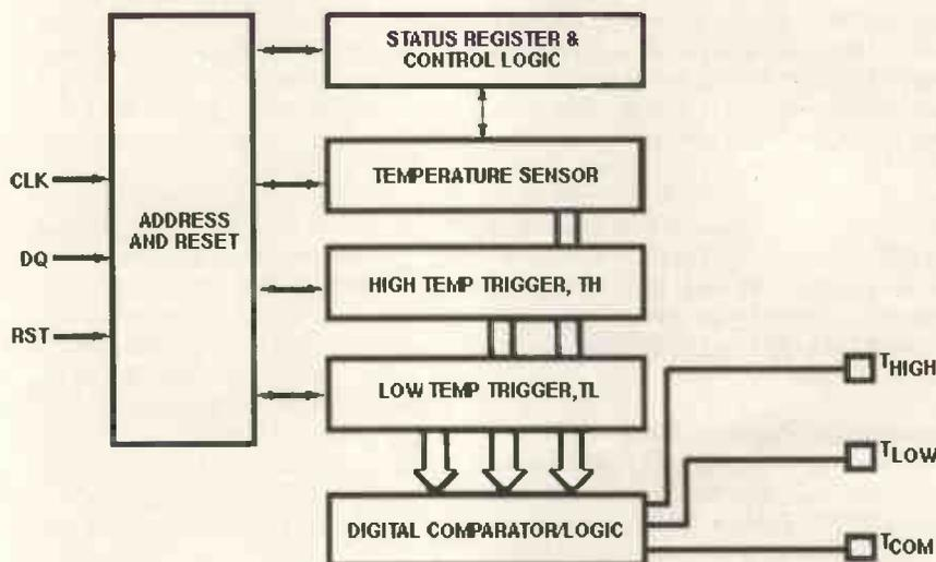
**Fig. 3. Programmable via a simple three-wire interface, the DS1620 registers are used to set temperature thresholds and set the operating mode. Programming is non-volatile so the device can act as a stand-alone controller.**
