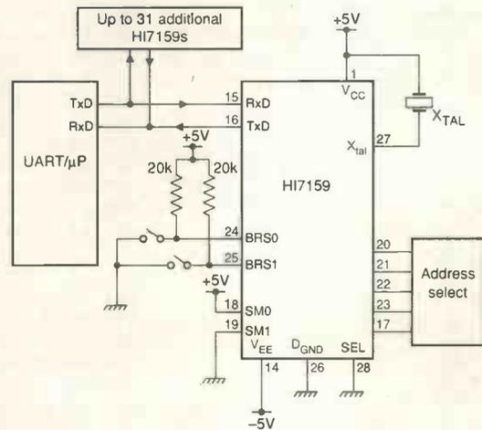
**Fig. 1. Serial-mode 2 allows several  $5\frac{1}{2}$ -digit HI7159 a-to-d converters to be addressed independently.**
