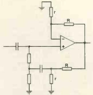
**Possible solution for isolating Self's amplifier's input bootstrapping from its feedback.**
