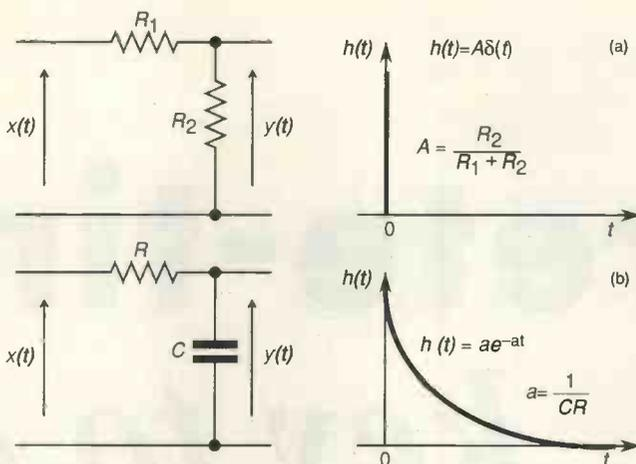
attenuated version of the input, and does not depend on past or future inputs.
