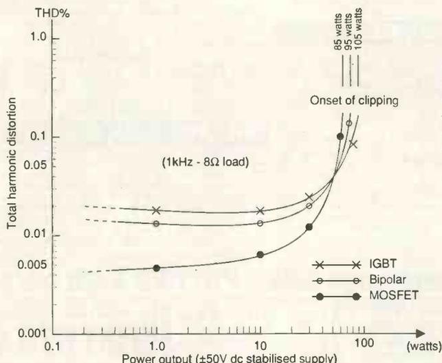
Fig. 3. Relationship between power and total harmonic distortion reveals interesting results.
