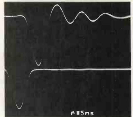
Fig. 1. Multiple reflections caused by a typical probe feeding a 100MHz oscilloscope, upper trace, are almost entirely absent in when the active probe is used, lower trace, in a matched 50 $\Omega$  system.
