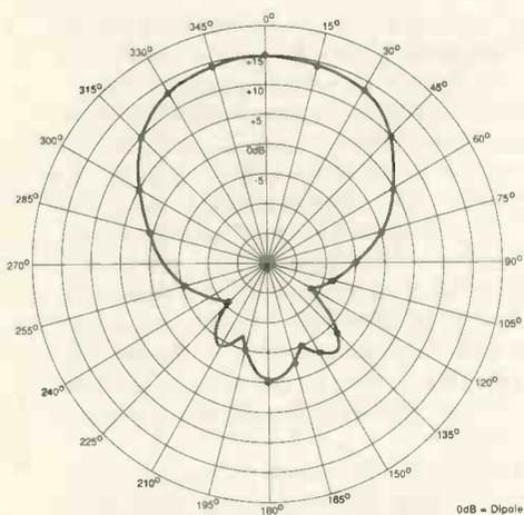
Fig. 2. Horizontal test pattern of the 24cm parabolic antenna. Frequency 1255MHz, swr 1:1.2 and power 1W.
