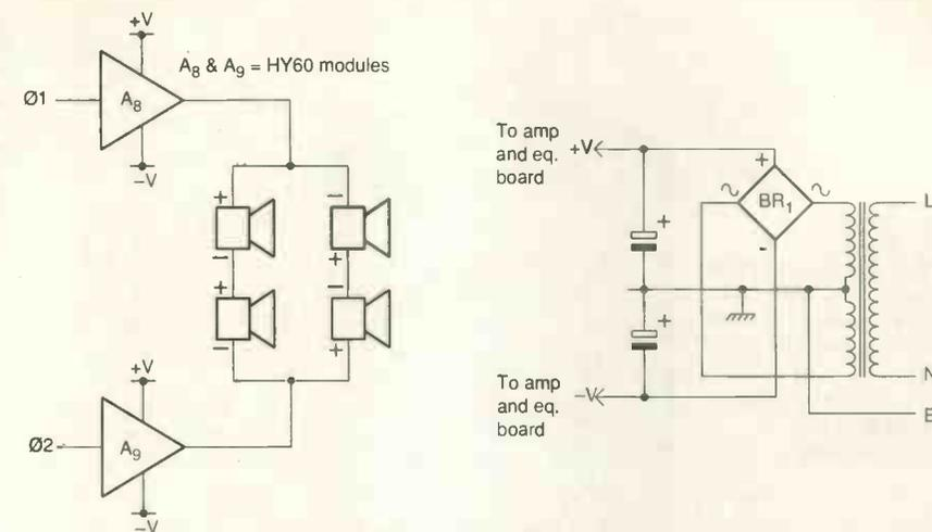
Fig. 4. Wiring the drivers in series/parallel results in an overall impedance of 8Ω from four 8Ω drivers. Pairs of drivers are driven in antiphase and mounted face-to-face.
