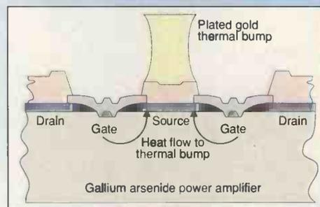
*Profiled bumps could be the answer to heat dissipation problems in GaAs power amplifiers.*
