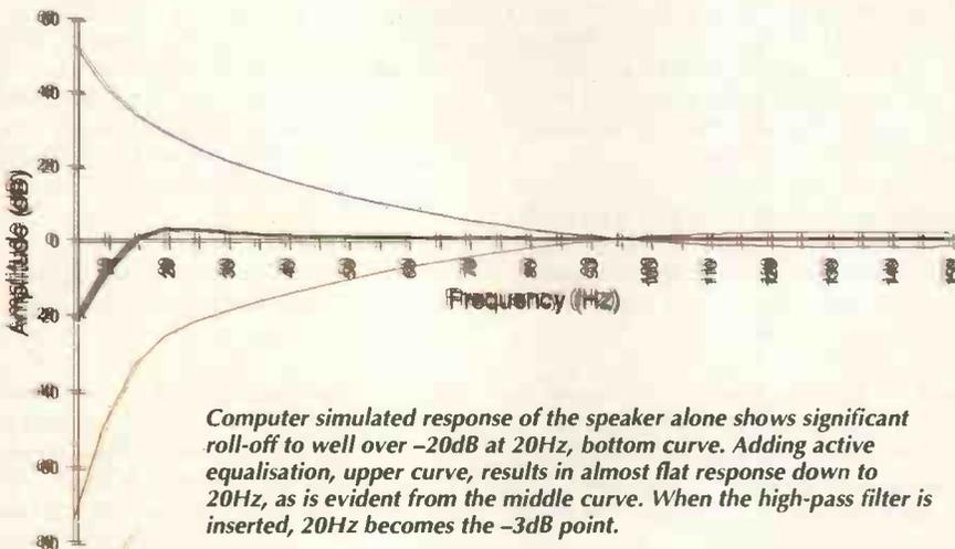
Computer simulated response of the speaker alone shows significant roll-off to well over -20dB at 20Hz, bottom curve. Adding active equalisation, upper curve, results in almost flat response down to 20Hz, as is evident from the middle curve. When the high-pass filter is inserted, 20Hz becomes the -3dB point.
