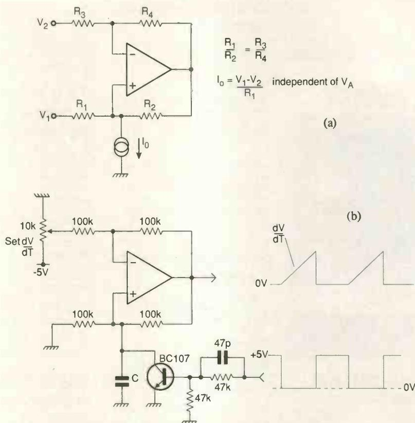
Fig. 7(a). Howland current pump provides an accurate, linear, bipolar, voltage-controlled current source. Non-inverting integrator at (b) is arranged as a linear timebase circuit.
