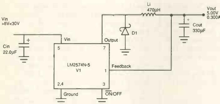
Fig. 7. Switch-mode power supply example incorporating the LM2574 Simple Switcher demonstrates how few external components the device needs.
