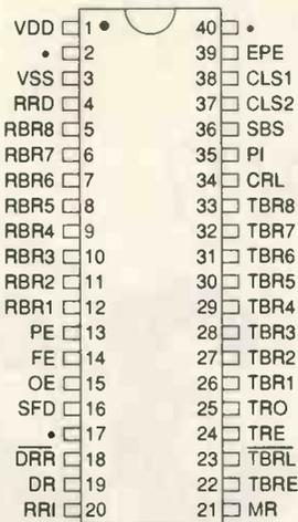
Fig. 2. Conveniently, the 6402 uart has separate eight bit input and output ports.
