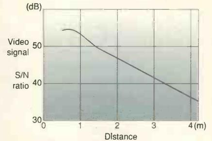
As distance between the optical transmitter increases, so does noise. Past 3m, the s:n ratio falls below 42dB and starts to become a problem.
