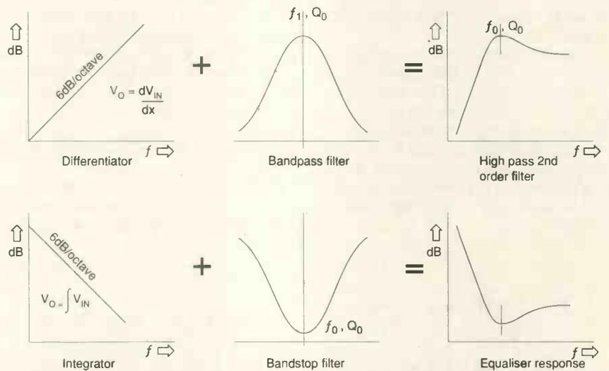
Synthesising a second-order high-pass filter from a differentiator and bandpass filter. For equalisation purposes, an inverse response can be generated by combining a bandstop filter and integrator.
