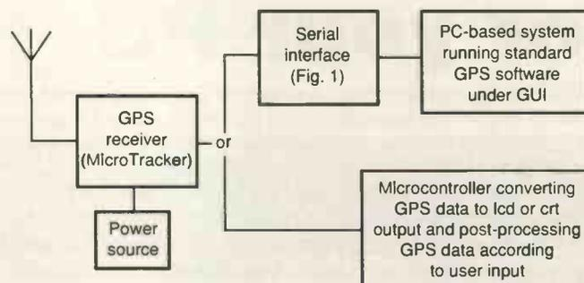
**Complete system for reading and presenting GPS data. The GPS antenna, Microtracker and pc software providing the two displays shown in this article are all part of the designer's kit.**
