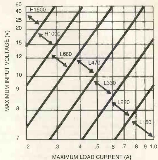
Fig. 4. With the Simple Switcher concept, choosing an inductor is simplified by focussing on a range of readily available standard parts.
