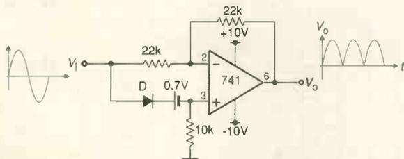
*This full-wave rectifier is unusual in its use of a single op-amp, paying the price for simplicity by its need for a bias voltage.*
