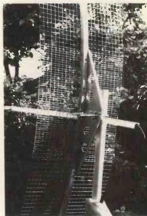
Featuring wide beam, wide bandwidth and useful gain, the 24cm antenna is easily disassembled for transportation.
