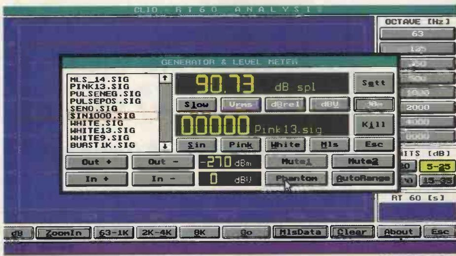
**Fig. 1.** The generator/voltmeter front panel window allows input/output conditions to be set and then dropped down over most instrument displays. The Clio board has two inputs and two outputs, but current software commons both outputs but uses only one input. Being able to use both sets independently would simplify stereo testing.
