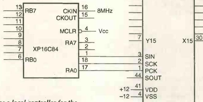
*PIC used as a local controller for the AD75019 cross-point switch allows control by a main processor which is unable to comply with the minimum 20kb/s transfer rate.*
