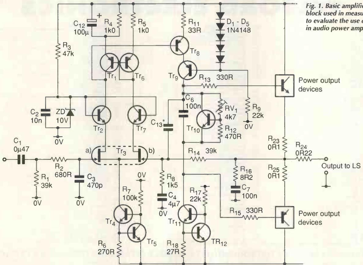
**Fig. 1. Basic amplifier gain block used in measurements to evaluate the use of igbts in audio power amplifiers.**
