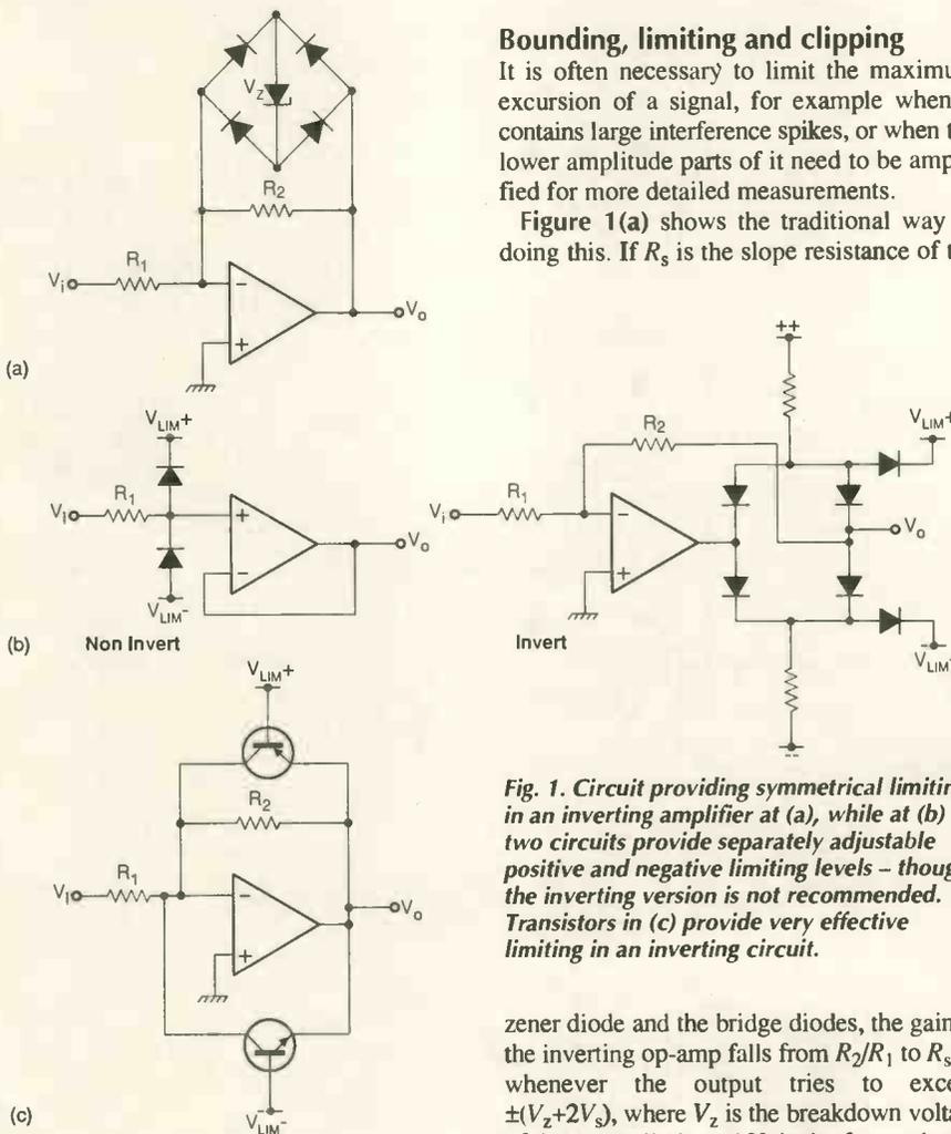
**Fig. 1. Circuit providing symmetrical limiting in an inverting amplifier at (a), while at (b) two circuits provide separately adjustable positive and negative limiting levels – though the inverting version is not recommended. Transistors in (c) provide very effective limiting in an inverting circuit.**
