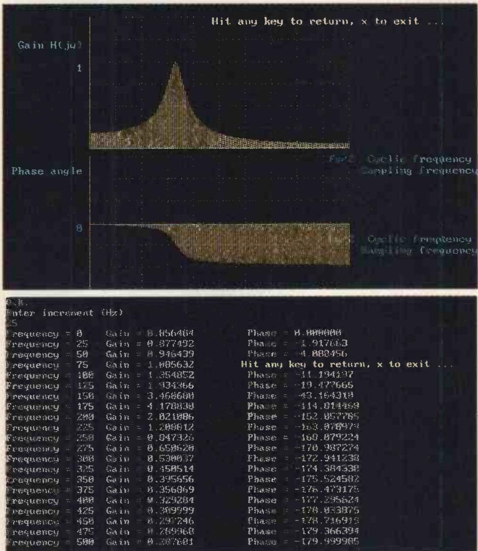
Fig. 7. Variations in the spectral response of  $H(z)$ , obtained by varying the radial position of the poles, graphically demonstrate how the Q-factor or sharpness of the peak in the amplitude ratio is related to the positions of poles relative to the unit circle. Values are  $\Omega_0 = \pi/3$ ,  $a = 0.9$ . The numerical response demonstrates performance for  $F_s = 1000\text{Hz}$ ,  $\delta f = 25\text{Hz}$ .
