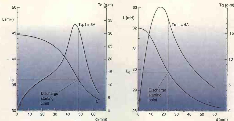
**How inductance of the electromagnet relates to displacement of the core from the electromagnet. Rate of change of the inductance depends on the magnetic fields and is greater in the attracting mode.**
