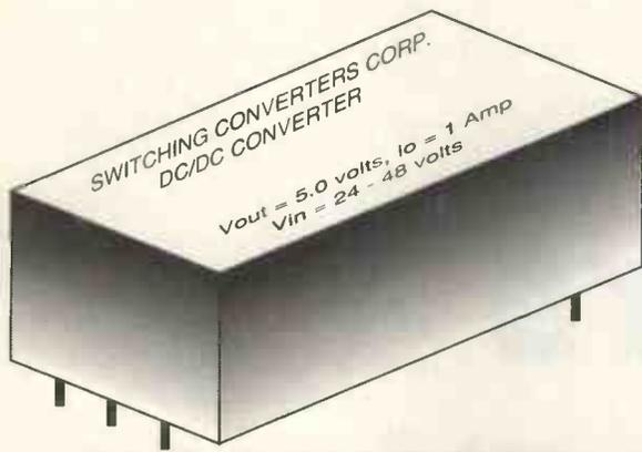
Fig. 2. Allowing designers to reap the benefits of switch-mode power supplies without incurring all of the associated design time and cost penalties, standard modules have become a viable alternative to discrete circuitry.
