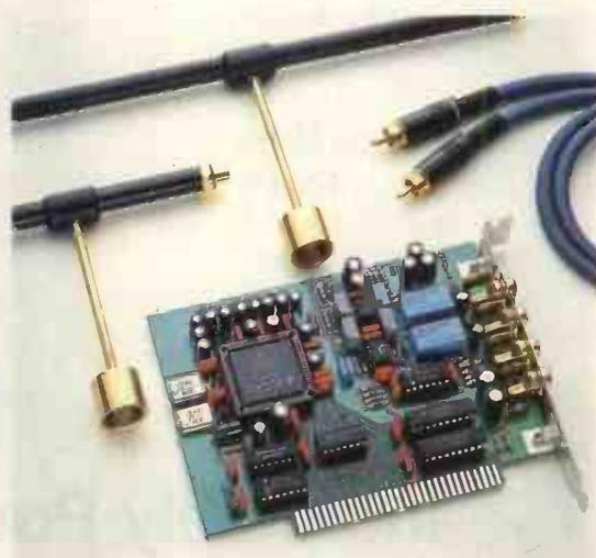
sine frequency response analyser, 10Hz–20kHz storage oscilloscope with 20kHz bandwidth and a fast Fourier transform, FFT, analyser. Spectrum analysis to 20kHz is possible, and the system can measure total harmonic distortion, ac millivolts, Vrms, dBV, dBm and dB relative, fast and slow reading. Sensitivity is up to +30dBV and down to -40dBV. An LC meter is also built in.
