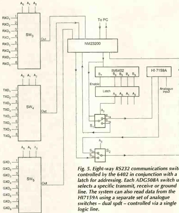
Fig. 5. Eight-way RS232 communications switch controlled by the 6402 in conjunction with a latch for addressing. Each ADG508A switch unit selects a specific transmit, receive or ground line. The system can also read data from the HI7159A using a separate set of analogue switches - dual spdt - controlled via a single logic line.
