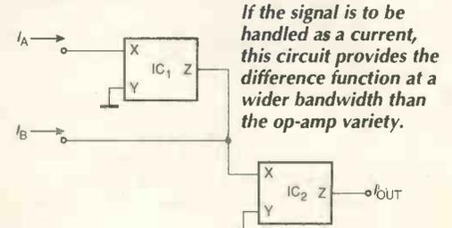
*If the signal is to be handled as a current, this circuit provides the difference function at a wider bandwidth than the op-amp variety.*
