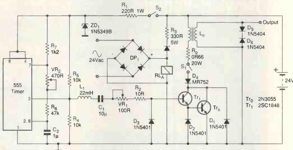
*Simple and efficient inverter provides a backup source for waveform-tolerant equipment and maintains a charge on the battery pack.*
