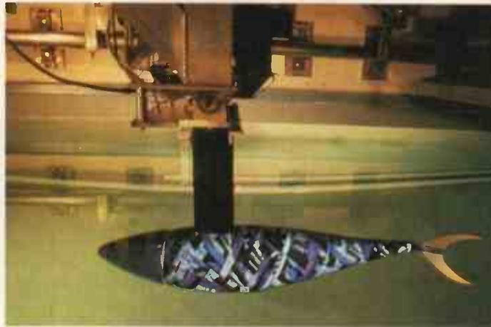
electronic robotuna. The mechanical fish has been built, as far as possible, to resemble a real one and its 2843 parts include over 40 ribs, a set of tendons, a segmented backbone with vertebrae, and a Lycra skin. The robot swims down the tank propelled by a tail that gently swishes back and forth as its flexible body follows suit.
