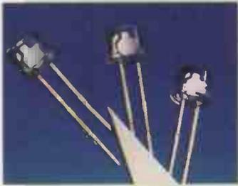
**Laser diode.** Made by EG&G in Canada, the C86137E InGaAs pulsed laser diode uses a multiple quantum well design to give a peak output of 8W at a peak forward current of 25A and 10V; wavelength is 905nm. Price is under £10.00. Pacer Components Ltd. Tel., 01734 845820; fax, 01734 845425.
