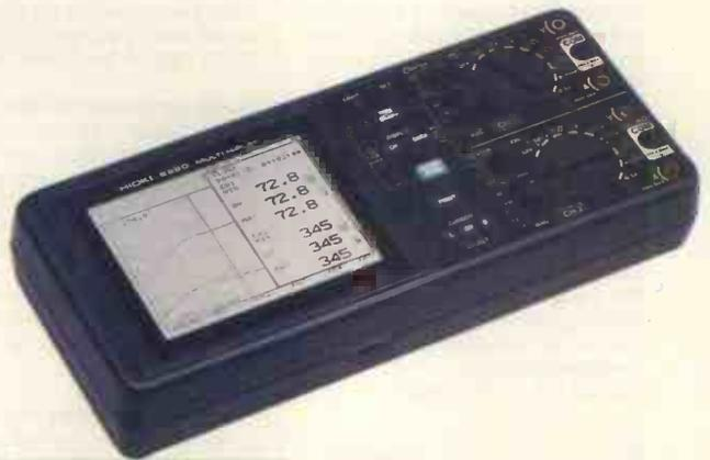
**Multimeter/recorder.** Hioki offers the 8220 Multi HiPlay combined digital multimeter and recording instrument, which presents changes in dual-channel voltage and current readings on an lcd graph. The instrument simultaneously displays on the 5in lcd and stores readings for up to six days, giving a graph of variations over time. A cursor gives a numerical reading of values from the graph, including minimum, maximum and average values, date and time. 01734 786911; fax, 01734
