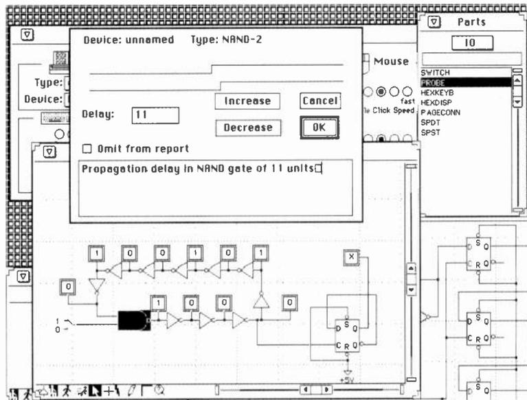
Fig. 4. Propagation delays can be adjusted in highlighted components.
