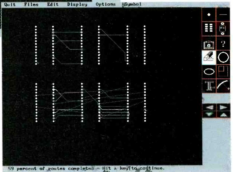
The two silk screen layers and eight copper layers available may be less than that offered by some other packages but they are more than adequate for most applications. The current working layer is displayed on the status bar and layers can be turned on and off in any combination. Solder resist layers are automatically generated from the pad pattern.
