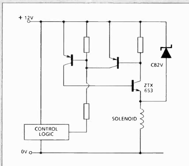
Fig. 3. As a protection against shorts, this circuit imposes a current limit. The zener provides a clamp against transients.
