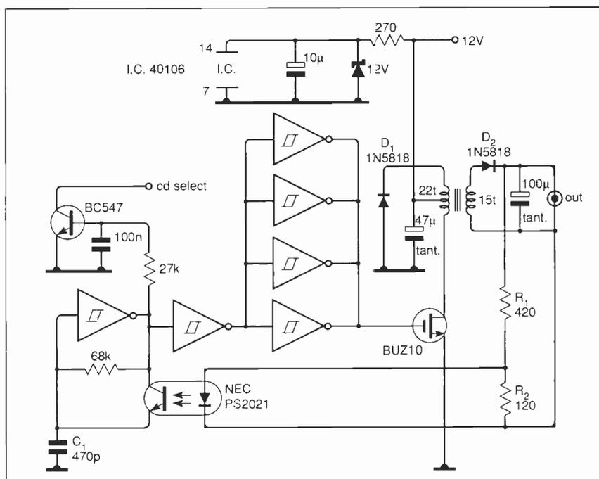
*Flyback converter with opto-coupled feedback gives floating power supply for car audio equipment.*
