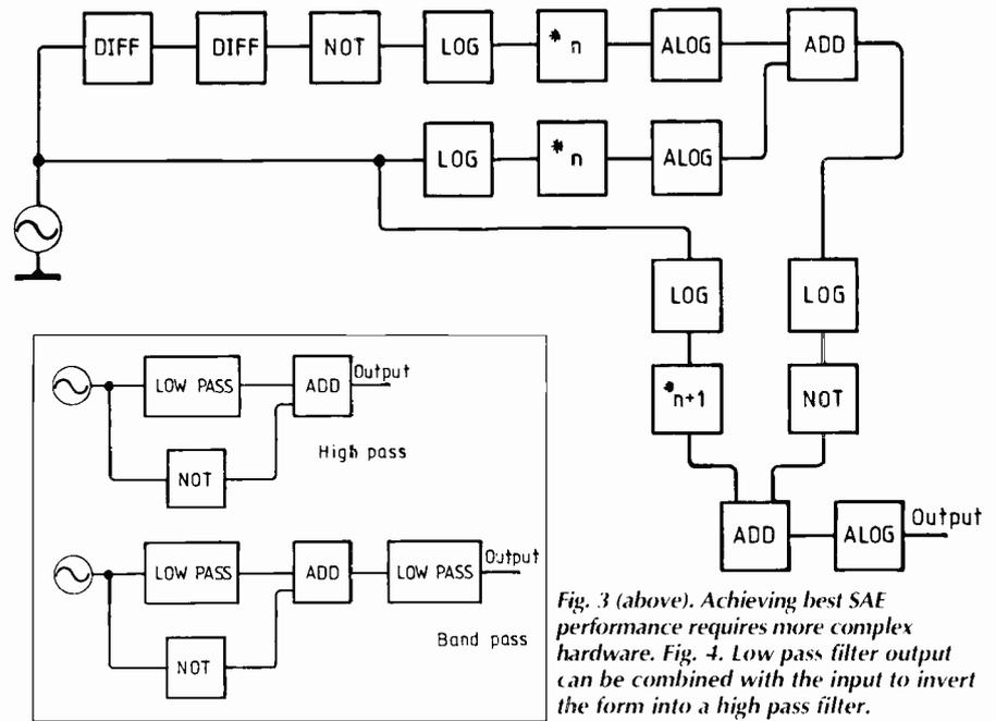
Fig. 3 (above). Achieving best SAE performance requires more complex hardware. Fig. 4. Low pass filter output can be combined with the input to invert the form into a high pass filter.
