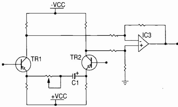
**Fig. 3. In discrete balanced microphone amplifiers the long-tailed-pair works directly into a differential IC or similar arrangement, and emitters cannot be directly coupled. Remove C<sub>1</sub> and replace it with a wire link and each transistor now shares the same resistor path to +Vcc.**
