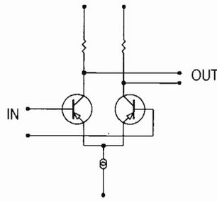
**Fig. 1. The long tailed pair is popular for differential or "balanced" signals.**
