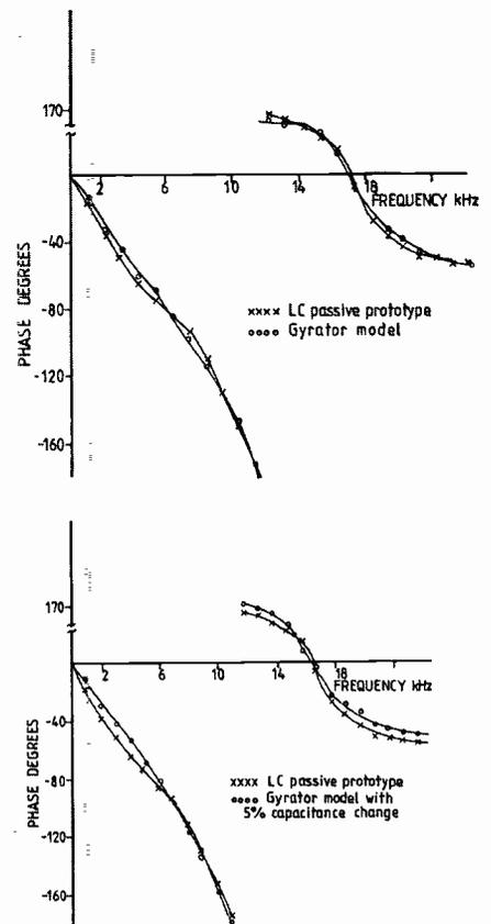
Fig. 9. Phase characteristics of the gyrator filter model compared with the prototype filter when capacitance is changed by 5%.
