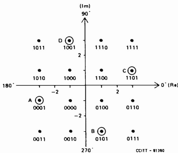
The baseband signal is modulated in both amplitude and phase; specific combinations correspond to the value – either one or zero – of a particular bit in the bitstream. This diagram represents a signal space map of trellis coded modulation at 9600 bits/s, V.32 standard. Derived from a 1200Hz tone, it sounds like a hiss to the ear.
