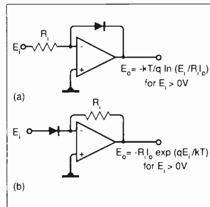
(a) Logarithmic amplifier with junction connected into negative feedback loop; (b) antilog amplifier.
