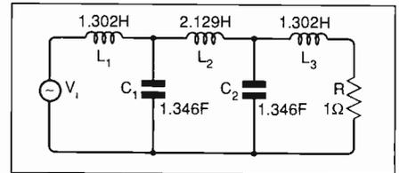
**Fig. 5 Prototype of a five-stage lowpass Tchebycheff filter. The circuit's inductors are floating.**
