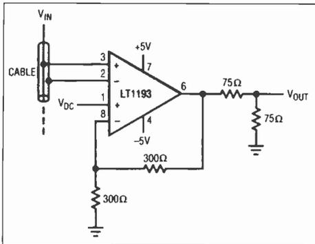
Fig. 3a. Cable sense amplifier for loop through connections with DC adjust.
