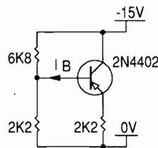
**Fig. 5. Test circuit for the 2N4402.**
