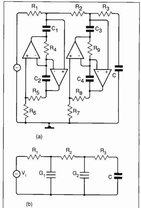
**Fig. 6. Gyrator circuit model derived from the circuit of Fig. 2. Fig.6a is the realisation that results; fig. 6b is the symbolic representation.**
