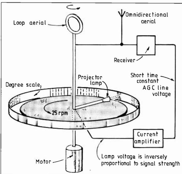
*Elementary scheme of radio navigator, showing one of two turntables. Light bulb flashes once each revolution when signal from aerial is at minimum, indicating direction of transmission on scale.*
