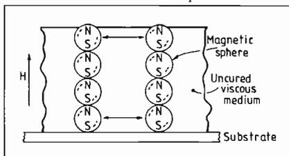
**Structure of the transparent conductor**
