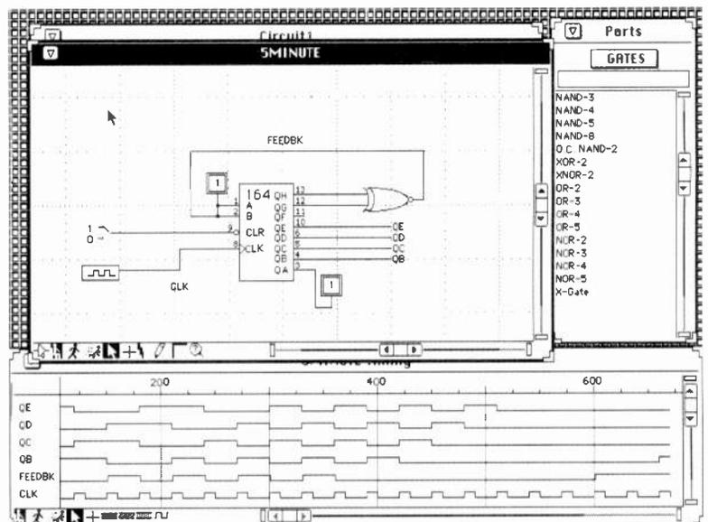
Fig. 5. Simulation diagram showing designer clock skew.
