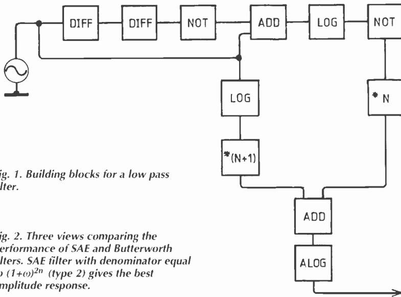
Fig. 1. Building blocks for a low pass filter.
