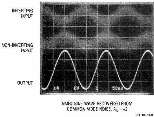
Fig. 3b. Recovered signal from common mode noise.
