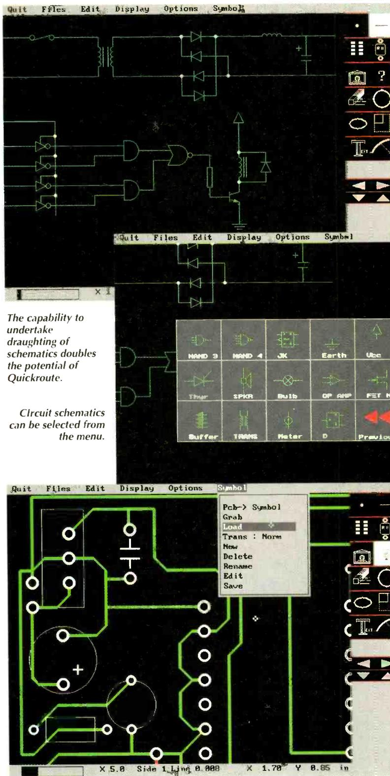
The capability to undertake draughting of schematics doubles the potential of Quickroute.
