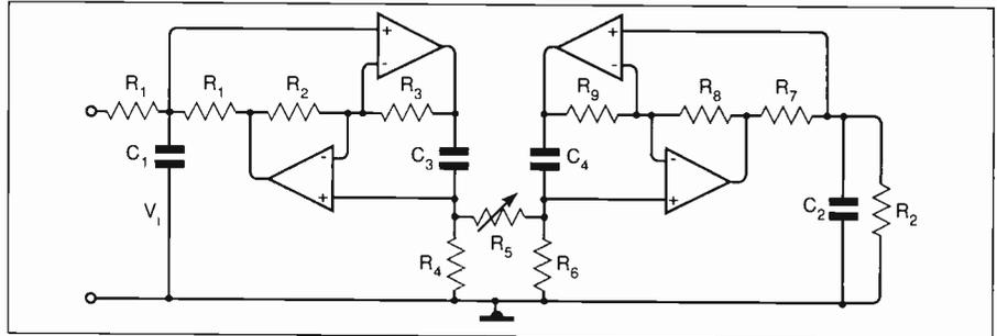
**Fig. 4 Gyrator realisation of bandpass filter from Fig.1b.**
