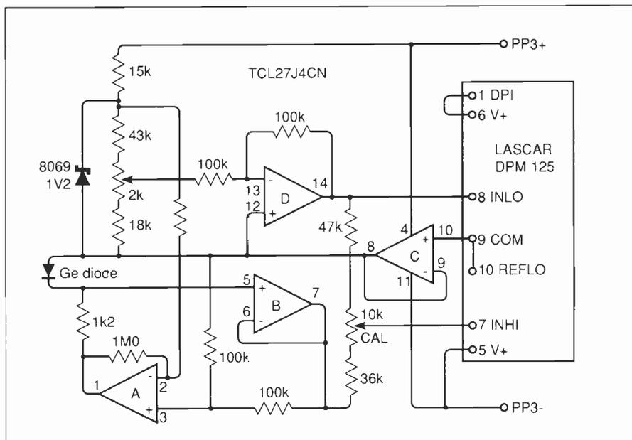
*Diode probe thermometer with digital readout measures from -25°C to 125°C*
