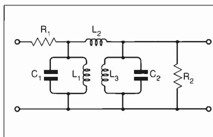
Fig. 3 Prototype of a coupled resonator bandpass filter.
