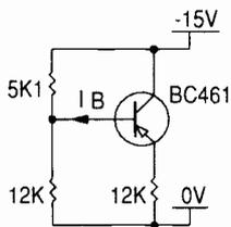
**Fig. 4. Test circuit for the BC461**
