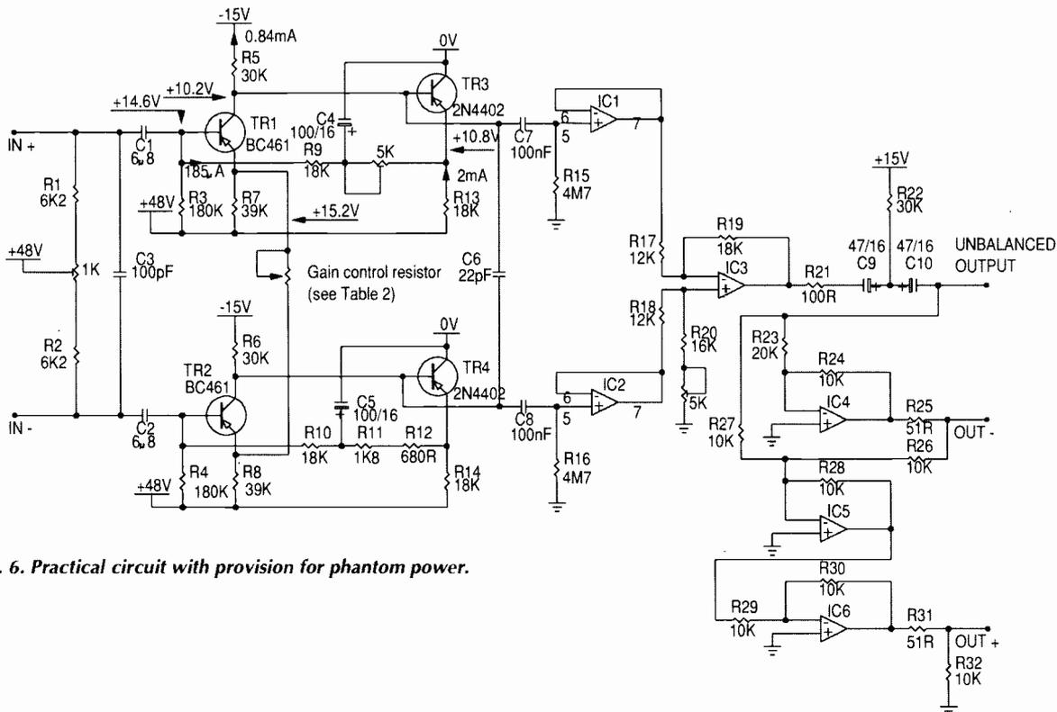
**Fig. 6. Practical circuit with provision for phantom power.**
