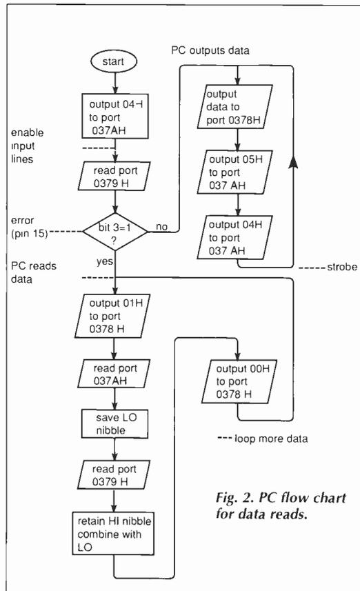
**Fig. 2. PC flow chart for data reads.**
