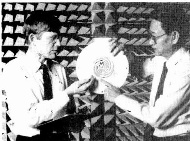
**Georgia Tech researchers Victor Tripp and Johnson Wang examine a new type of microstrip antenna. The spiral flat-plate provides bandwidths of up to 9:1 in the 2-18GHz frequency range. The circular polarisation makes it suitable for applications such as GPS, wireless lans and direct broadcast satellites. The planar nature of the system makes it eminently suitable for vehicle based use as does its small size – typically 5 to 12cm diameter.**
