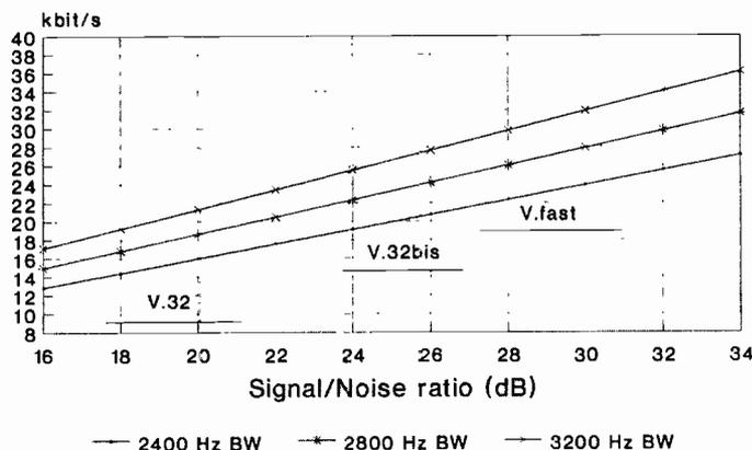
**Absolute channel capacity.** As channel capacity increases, so does the requirement for improved signal to noise ratio. V.fast requires at least 10dB more headroom to operate than circuits using V.32.
