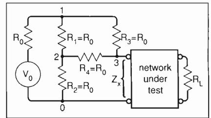
Modelling a return-loss bridge at the relevant port allows plot of insertion loss and, without further plot of computation, return-loss plot simultaneously.
