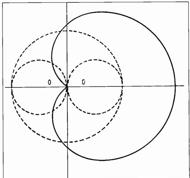
*Combined omni and loop polar diagram, showing heart-shaped field. Cardioid null is not quite as sharp as from loop alone and is usually used merely to show which way to turn loop for correct null. This is unnecessary in Lipschutz's design. Signal from omni must be exactly the same in magnitude and phase as that from the loop.*
