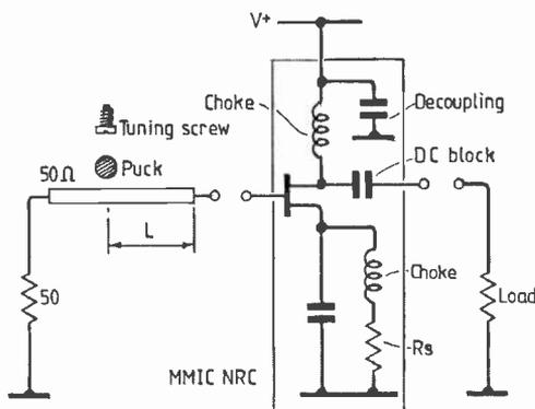
AW Dearn reported an RF-on-wafer MMIC-based dielectric resonator oscillator within a single-chip low-noise downconverter (LNC). Prototype chips have an IF output between 0.95 to 1.3GHz.
