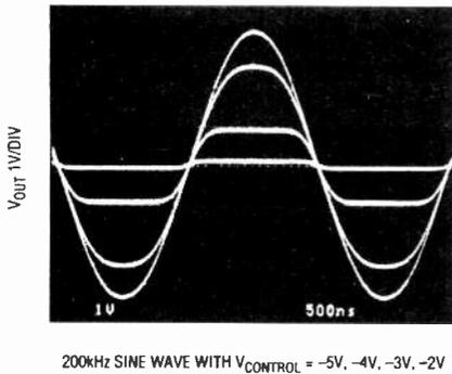
Fig. 3d. Sine wave reduced by limiting the *LT1194*.
