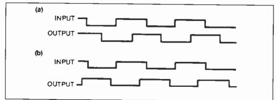
Fig. 2. An input signal of the same frequency (a) as the oscillator's frequency aligns the phase relationships so that the net effect is zero; (b) decreasing the input frequency hinders  $C_F$ 's charging, causing a decrease in the oscillator's frequency.
