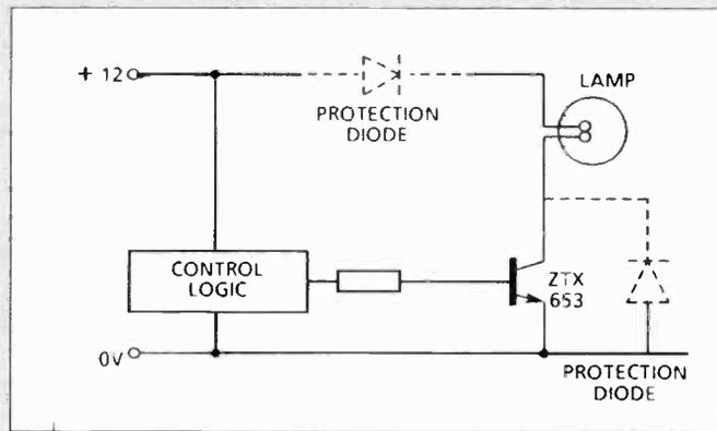
Fig. 1. Two ways of preventing a back-connected battery blowing up the control logic.
