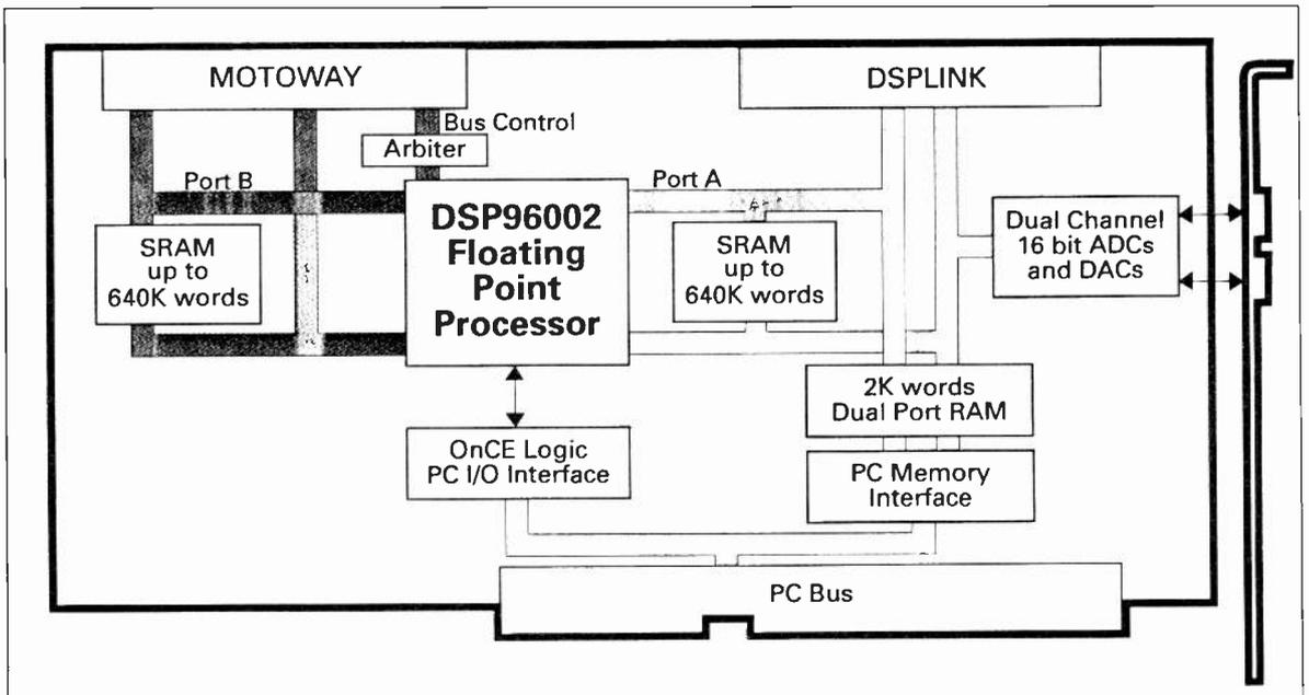
register (OMR) and the port select register (PSR). Sram can be augmented to a maximum of 5Mbyte and for cost consideration purposes wait states can be included in the DSP96002 memory access timing.
