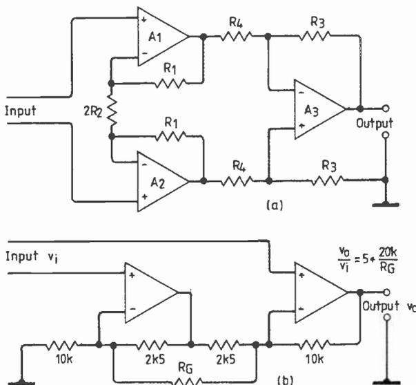
Fig. 1. Instrumentation amplifiers, floating high-impedance input. Circuits using (a) three op-amps or (b) two op amps.
