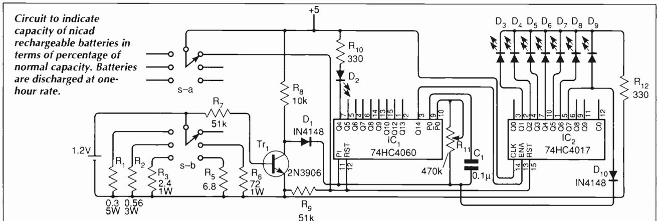
Circuit to indicate capacity of nicad rechargeable batteries in terms of percentage of normal capacity. Batteries are discharged at one-hour rate.
