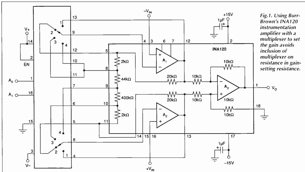
Fig.1. Using Burr-Brown's INA120 instrumentation amplifier with a multiplexer to set the gain avoids inclusion of multiplexer on resistance in gain-setting resistance.
