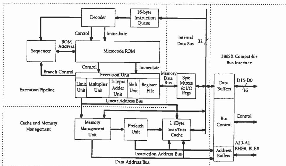
386 pin-compatible Cyrix architecture speeds up a PC by a factor of two over a 386 powered machine run at the same clock speed. Extensive use of pipelining accounts for the boost.
