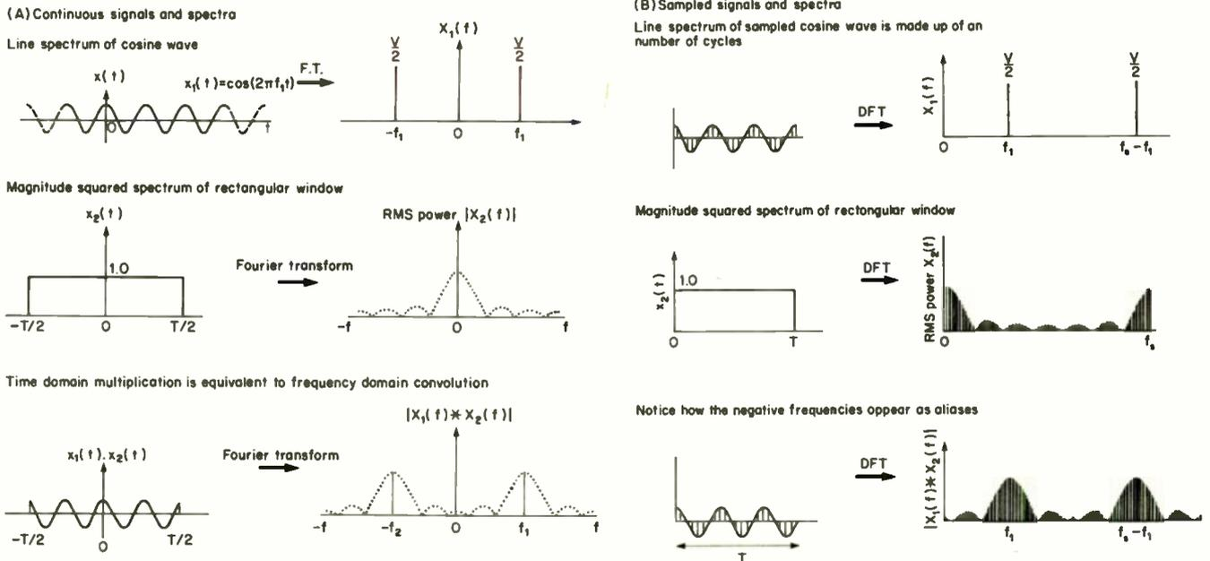
Fig. 6.18. Interpreting analogue and digital frequency spectra.
