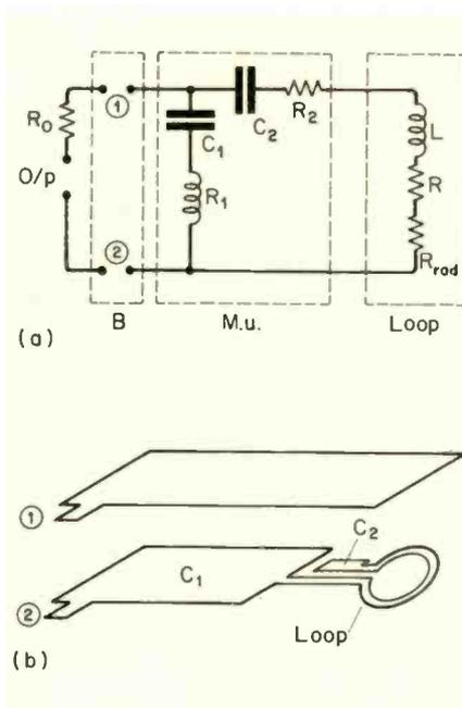
**Experimental 500MHz loop receiving antenna using superconducting capacitor ( $C_2$ ).**
