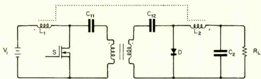
Fig. 4. Dividing the capacitance and the associated inductance allows supply isolation.
