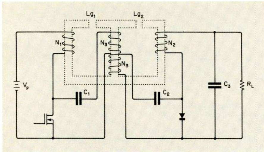
Fig. 5. Cúk converter with all windings integrated into a single magnetic structure. Magnetic balance is critical and leakage inductance may cause problems.
