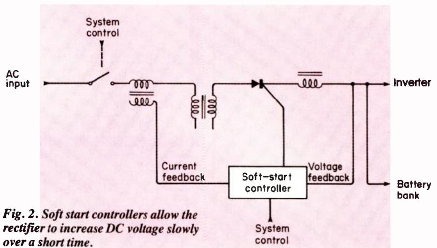
**Fig. 2.** Soft start controllers allow the rectifier to increase DC voltage slowly over a short time.
