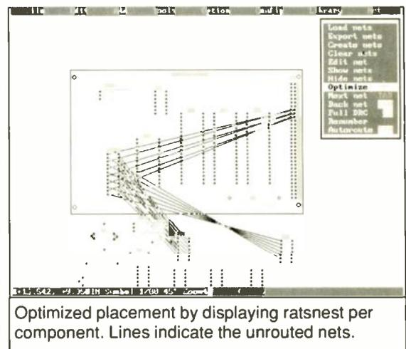
Optimized placement by displaying ratsnest per component. Lines indicate the unrouted nets.
