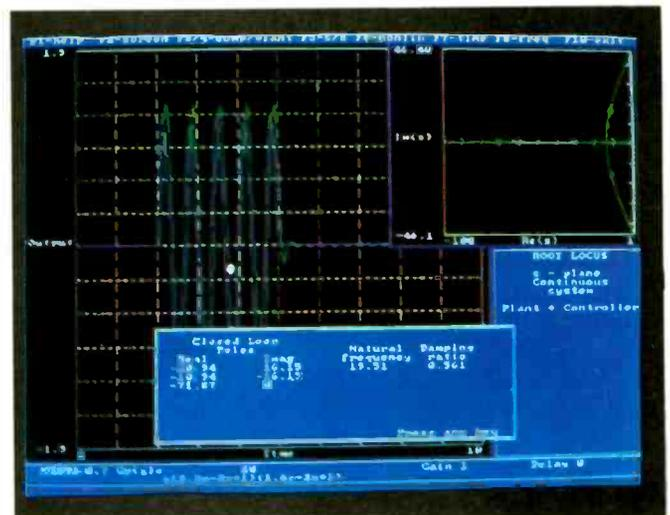
Top left. Root locus. This depicts movement of characteristic equation roots as system gain changes from zero to infinity. Note that their locus intersection of y axis indicates point of system instability. Top right. Nyquist plot for
