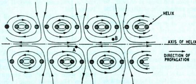
Lines of force of wave travelling along a helix (not to scale).
