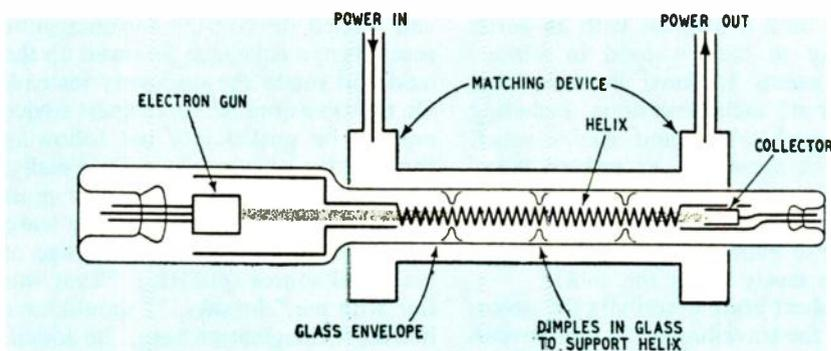
Layout of the travelling-wave amplifying tube.
