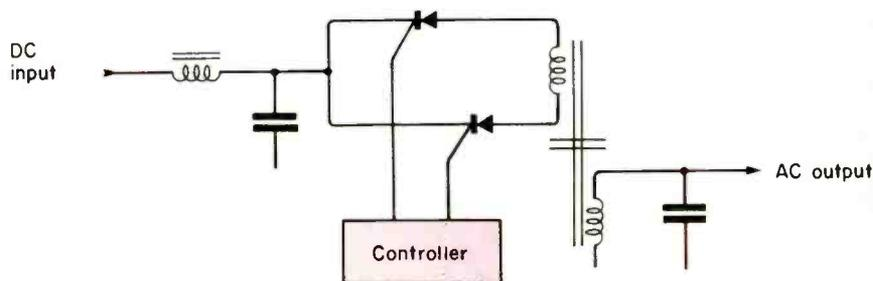
Fig. 3. The ferroresonant inverter is an SCR bridge with a tuned resonant transformer in its output.
