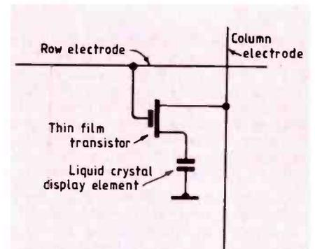
*Active-matrix element. Row and column electrodes are on glass substrates separated by 2 microns, with liquid crystal between them.*
