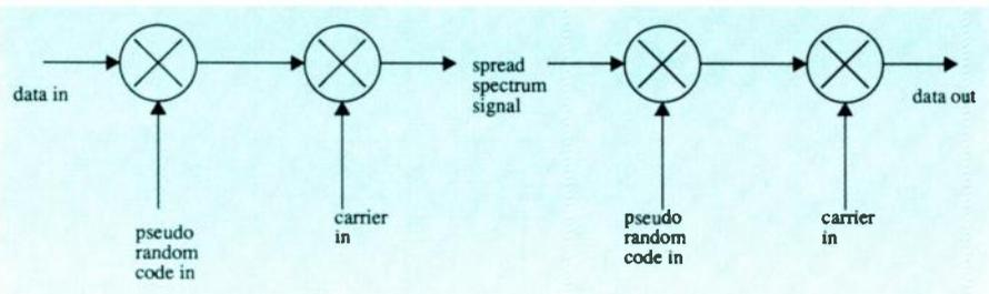
Nearly all the transmitted power is contained within the frequency range  $(f_0 - f_c)$  and  $(f_0 + f_c)$ , where  $f_c = 1/t_c$ . Chip frequencies,  $f_c$ , of between 1 and 10MHz are typical for carriers,  $f_0$ , in the low gigahertz regions.
