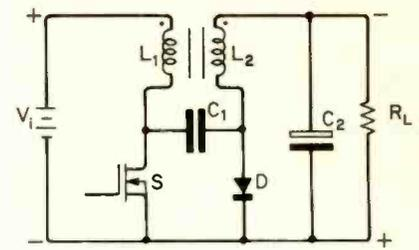
**Fig. 3.** The Cuk circuit allows the integration of separate inductors into a single, close coupled transformer. DC currents in the core cancel out minimising the problems of core saturation.
