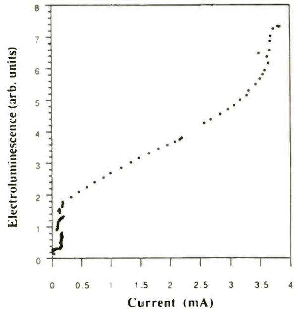
the whole idea is for light to emerge normal to the plane of the device. The graph shows light output characteristics of a polymer led in which PPV is sandwiched between a layer of indium oxide and a layer of aluminium.
