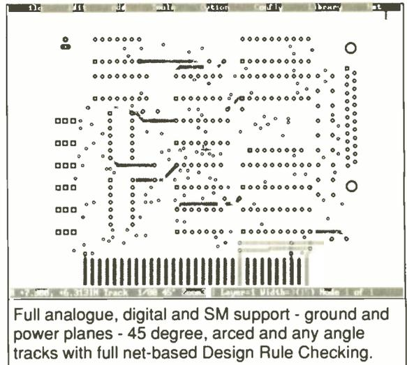
Full analogue, digital and SM support - ground and power planes - 45 degree, arced and any angle tracks with full net-based Design Rule Checking.
