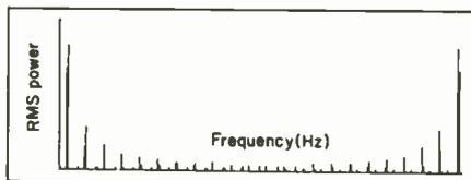
**Fig. 6.16.** Effect of processing real signals using listing 6.13 (FFT with data capture). At (a) is a sine wave of 3Vpk-pk at 5kHz (1024 data points) while (b) shows a 3Vpk-pk square wave 1kHz (512 data points).
