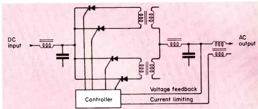
Fig. 4. Quasi-square-wave inverters use an SCR bridge to produce square waves, but regulation is provided electronically rather than magnetically.
