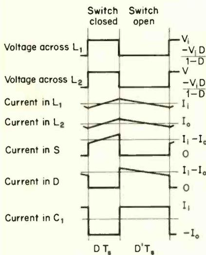
**Fig. 2.** Voltages and currents during the Cuk cycle
