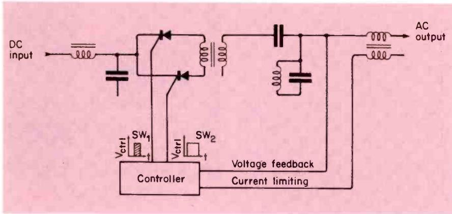
Fig. 5. A pulse width modulated inverter is a higher frequency version of the quasi-square-wave circuit.
