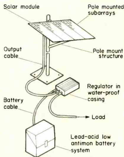
*Typical solar generator system (up to 200w load) as supplied by Solapak Ltd.*
