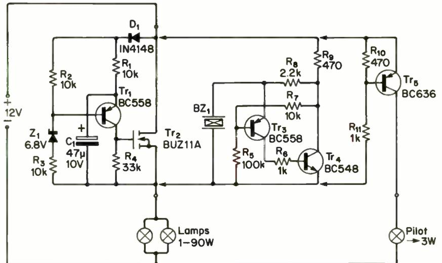
Transistors  $Tr_3$  and  $Tr_4$  act as another multivibrator, using two bipolar types, to provide an audible signal. The piezoelectric buzzer (Murata PZKM 4201 EPP) does not operate at
