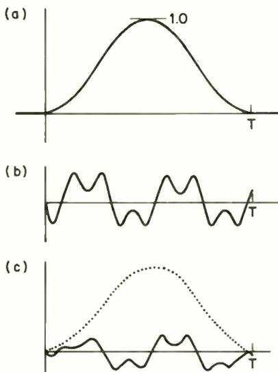
Fig. 6.19. Hanning window. At (a) raised-cosine function is generated using window  $w[z] = 0.5 * (1 - \cos(2 * \pi * z / N))$ , where  $z$  is sample point number and  $N$  number of samples. In (b) is truncated data set to be transformed and (c) shows effect of multiplying data set by Hanning window.
