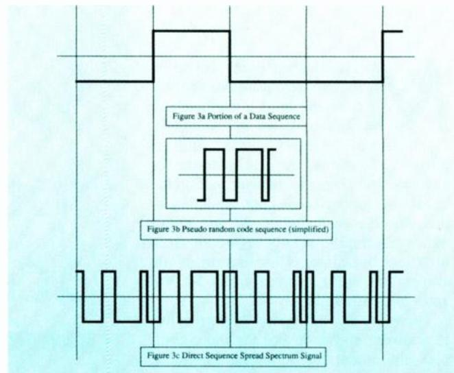
Fig. 3. Generating direct-sequence spread-spectrum signals by modulating the data with a pseudo-random code.
