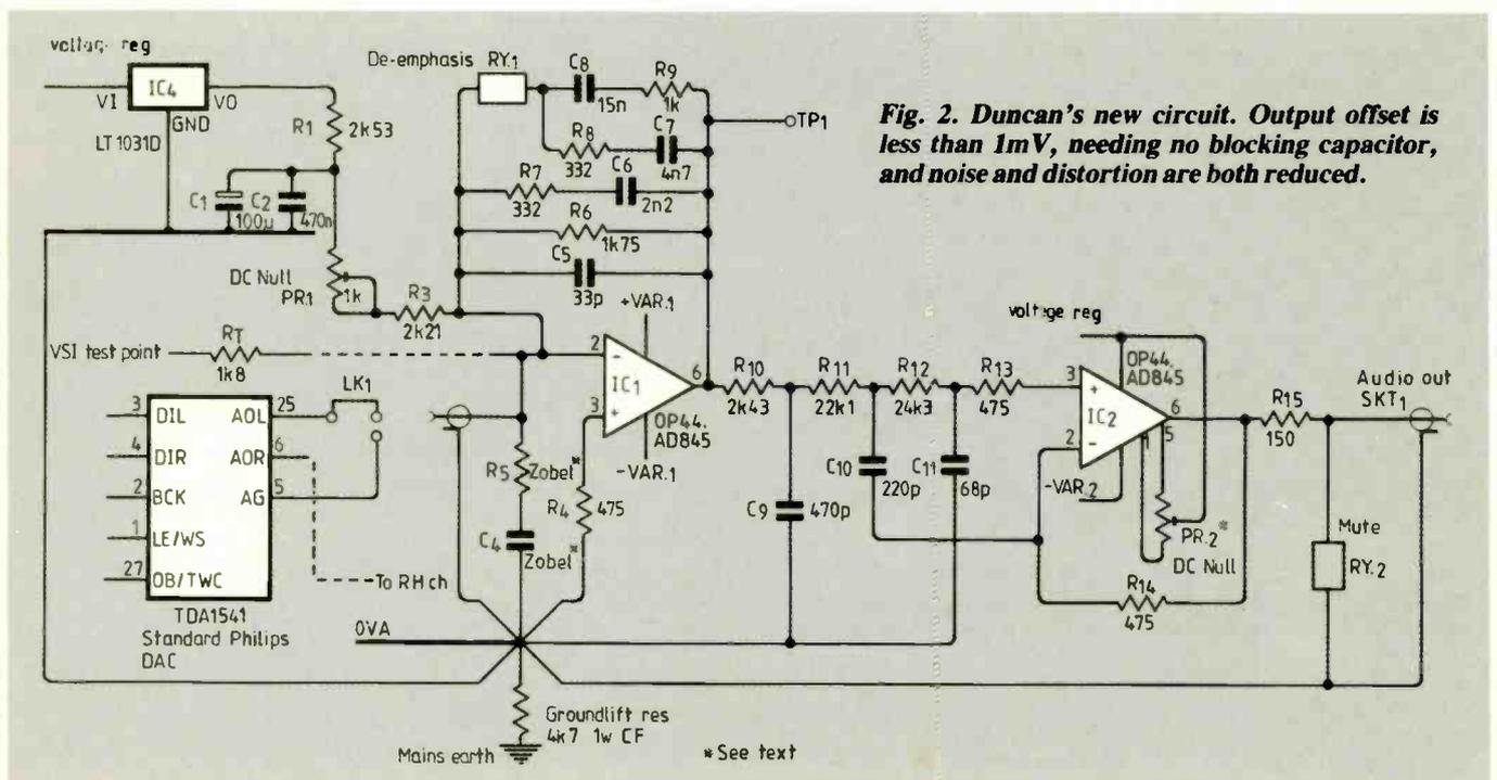
Fig. 2. Duncan's new circuit. Output offset is less than 1mV, needing no blocking capacitor, and noise and distortion are both reduced.
