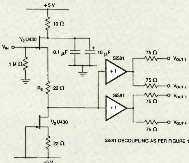
Fig. 3. Multiple-output high-performance buffer
