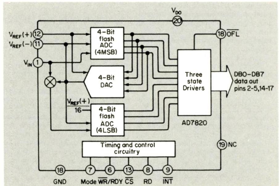
While the output from the A-to-D is latched, the digital signal is reconverted to analogue form for a second conversion with a 1/16 weighted network to make up the least significant bits of the 8-bit output word.
