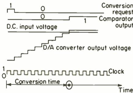
**Fig. 2.2** The conversion time of the counter-ramp A-to-D converter depends upon the amplitude of the input signal
