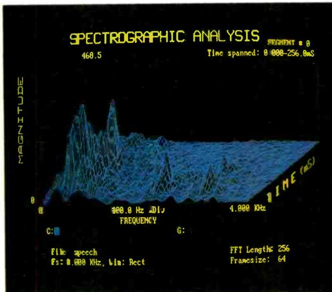
Fig. 3. Three-dimensional spectral display for showing development of a signal.
