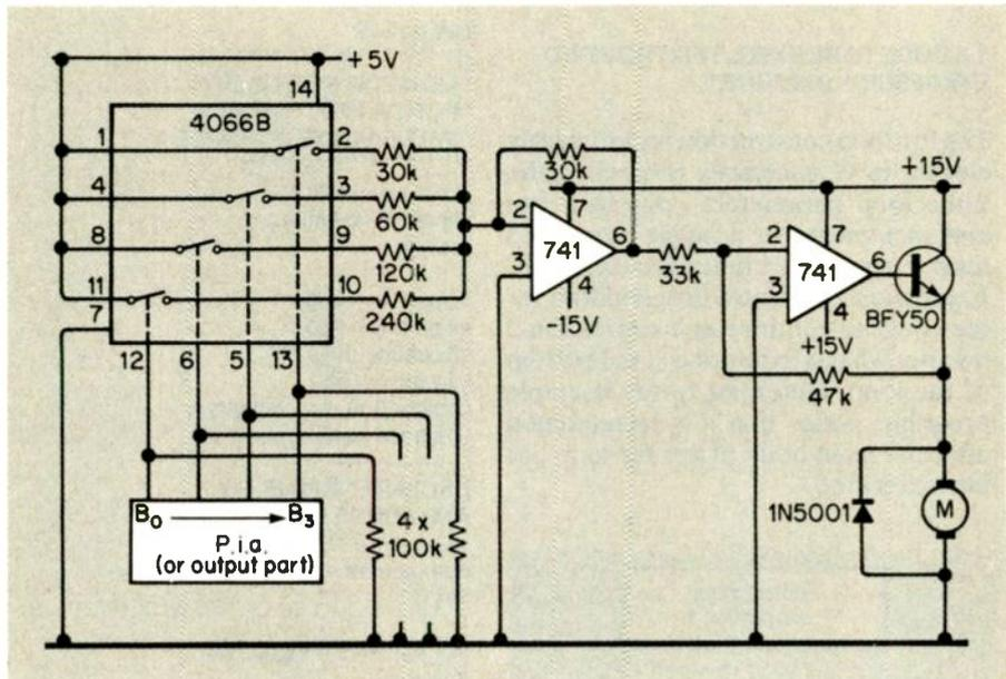
**Fig. 1.9** Hardware for computerised speed control is simple: most of the work is done by software.
