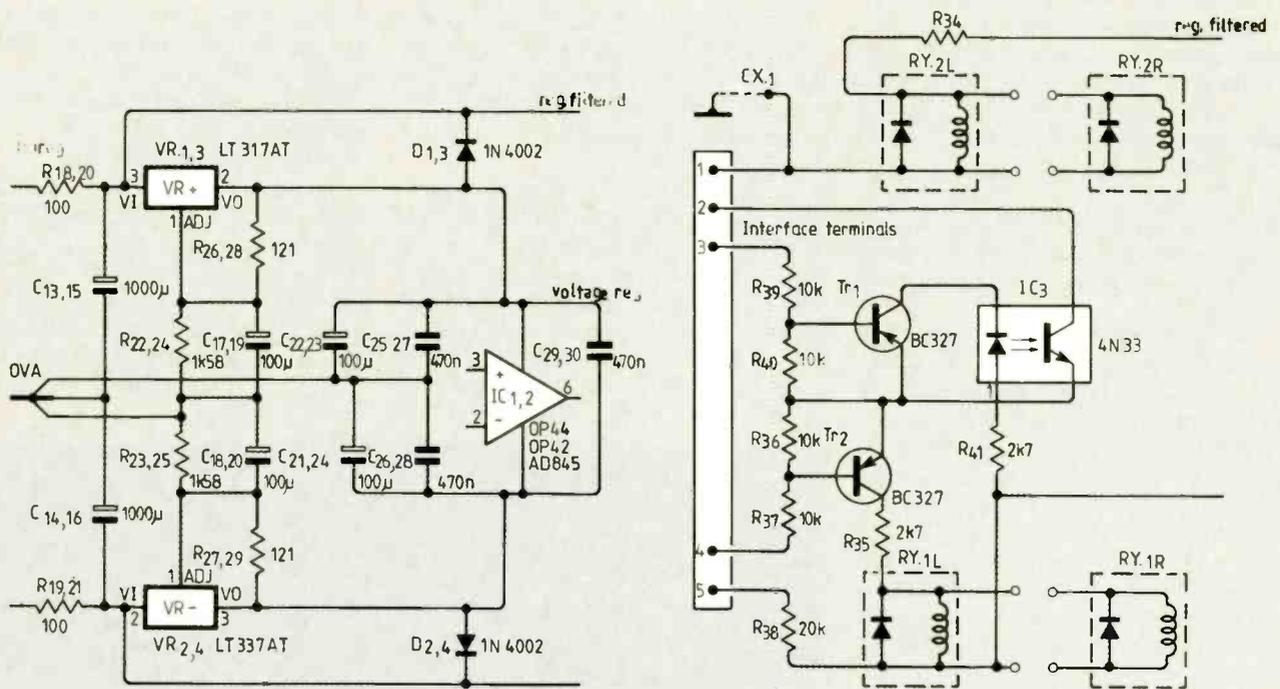
Fig. 3. Power supply and interfacing circuit for muting and de-emphasis relays.
