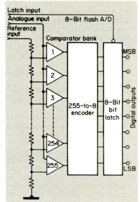
**Fig. 2.5** 8-bit conversion converts in one cycle.
