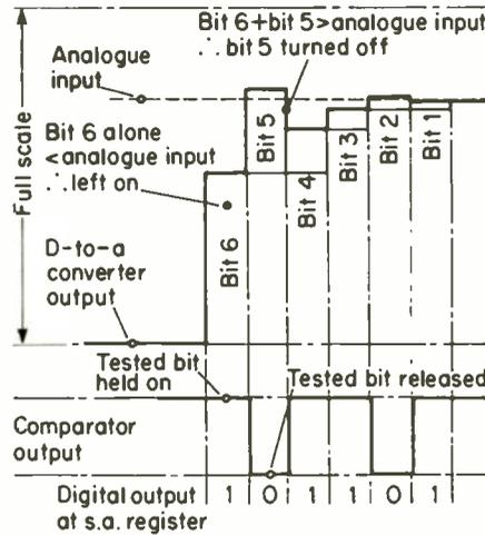
**Fig. 2.4** Successive approximation speeds up conversion time with conversion rates that can stretch from 400ns to 25s. The number of conversion steps required is equal to the number of bits in the data word plus one
