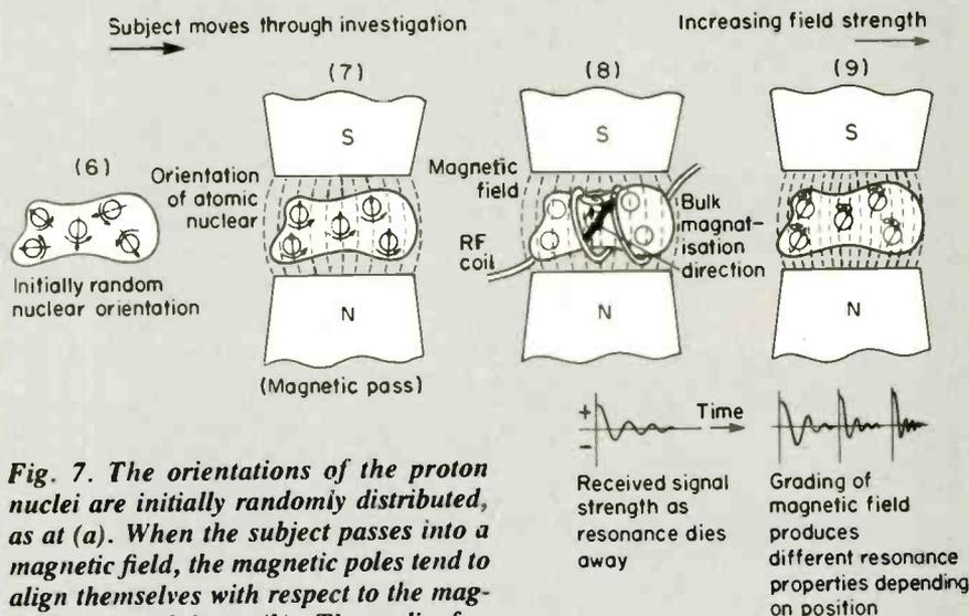
Fig. 7. The orientations of the proton nuclei are initially randomly distributed, as at (a). When the subject passes into a magnetic field, the magnetic poles tend to align themselves with respect to the magnetic lines of force (b). The radio frequency stimulus of the magnetic orientation of the bulk magnetisation direction causes this orientation to precess, as seen at (c). By graduating the strength of the magnetic field, the fre-
