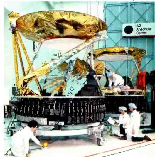
*Building satellites: the communications section of Intelsat VI. The completed satellite, launched on March 14, can carry 120 000 telephone calls and three TV channels. There will be five Intelsat VI spacecraft in orbit by the end of 1991.*
