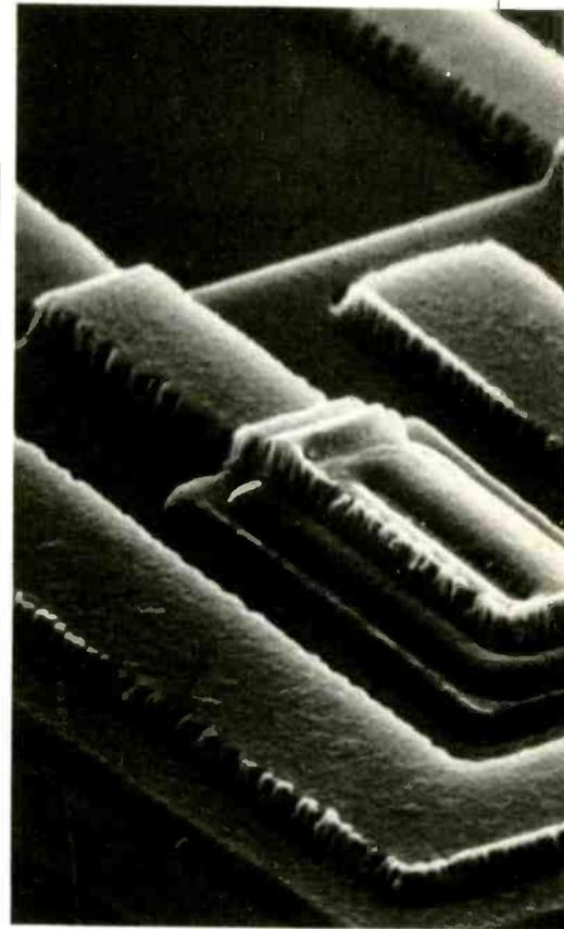
*The world's fastest silicon transistor? IBM researchers claim to have produced a bipolar transistor structure which operates at 75GHz, nearly twice as fast as existing devices.*
