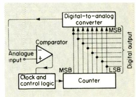
Fig. 2.1 System diagram of a counter-ramp A-to-D converter
