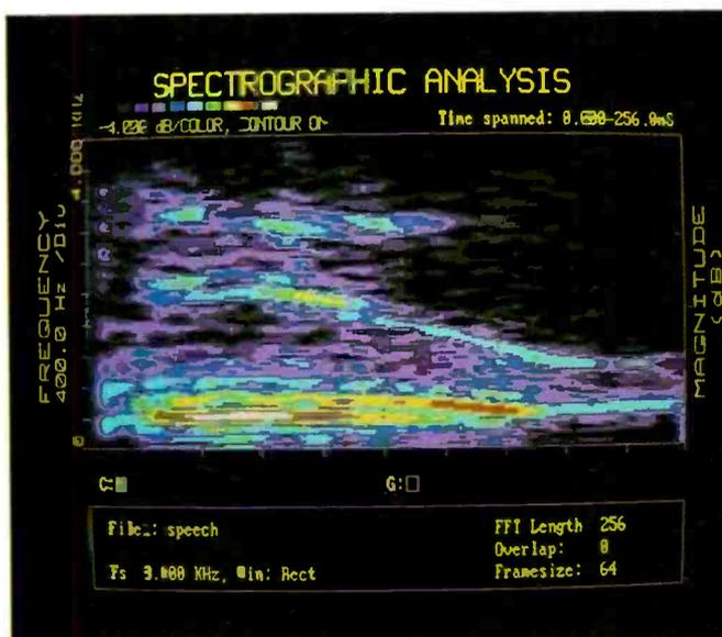
Fig. 4. Spectrographic mode displays a spectrum which changes with time, a facility often used in speech analysis.
