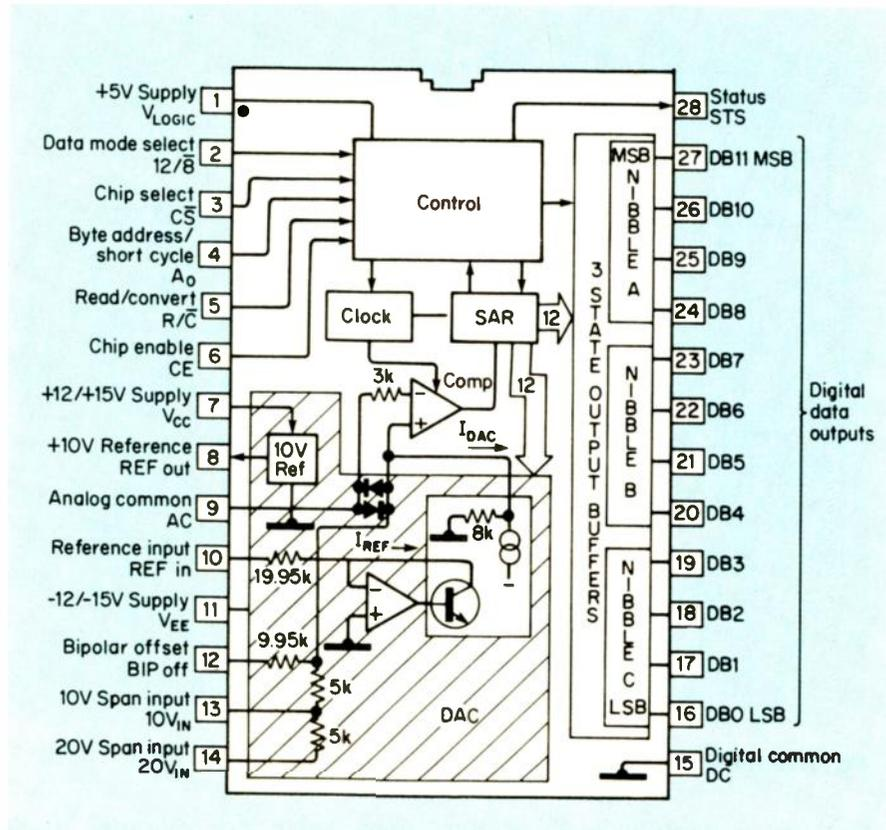
Fig. 2.9 AD574A block diagram and pin configuration
