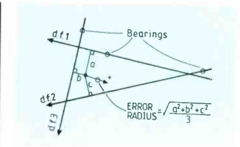
Fig. 3. Derivation of the error radius, where the cross indicates the mean of two station fixes.
