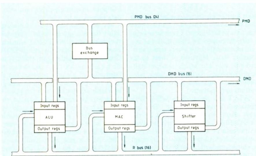
Fig. 4. Analog Devices ADSP2100 has dedicated MAC and straightforward arithmetic section.
