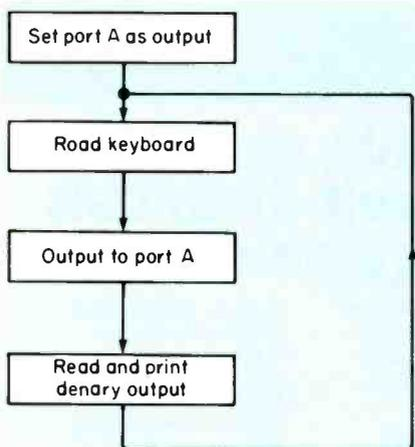
Fig. 1.8 A simple loop mirrored by listing 1.6
