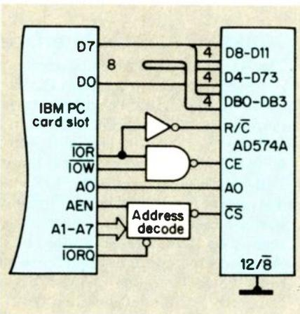
Fig. 2.10 IBM PC - AD574A interface
