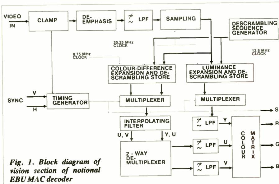
Fig. 1. Block diagram of vision section of notional EBU MAC decoder
