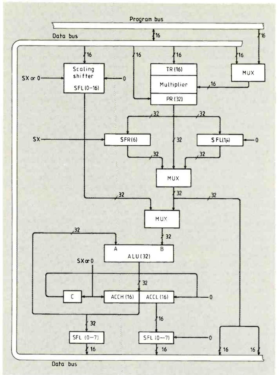
**Fig. 3. TMS32025 arithmetic section. Well established, but suffering from lack of a multiply/accumulator (MAC) and inelegant architecture.**
