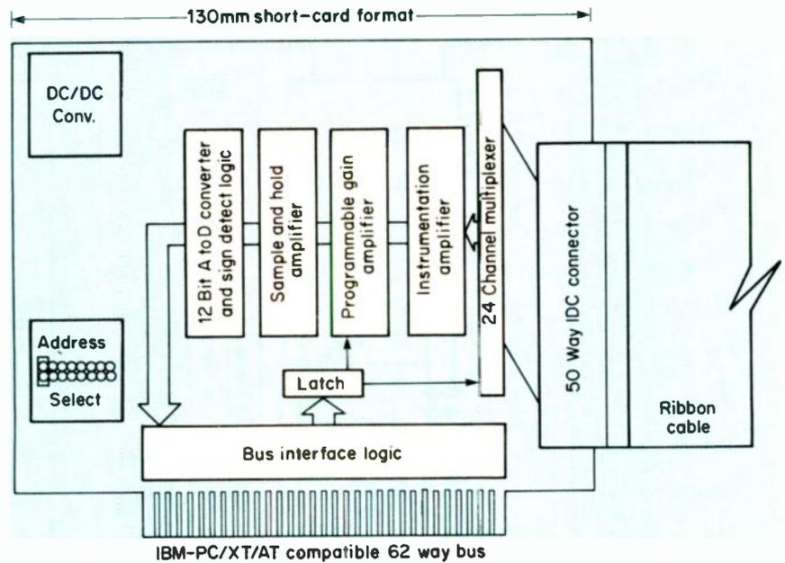
Fig. 2.7 AIP-24 functional block diagram
