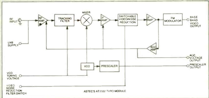
*Satellite mini-receiver. Astec's receive-only module covers 950 to 17750MHz, the downconverted European satellite TV band, and provides positive sync, raw video derived from a demodulated IF of 479.5MHz. Quoted noise figure is 12dB. An internal prescaler can be set to either 256 or 512 for use with an external synthesised tuning system.*
