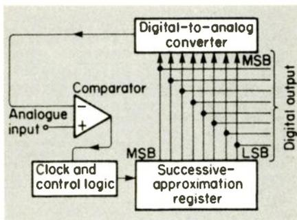
**Fig. 2.3** System diagram of successive approximation A-to-D converter
