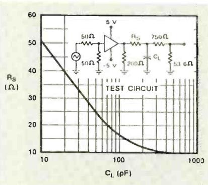
Fig. 2. Series isolating resistor and  $C_{LOAD}$  selection
