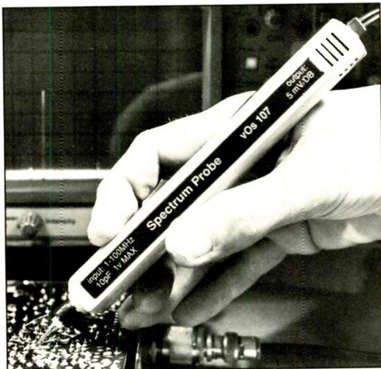
The 107 SPECTRUM PROBE converts a standard 1 MHz scope into c 100 MHz spectrum analyser.
