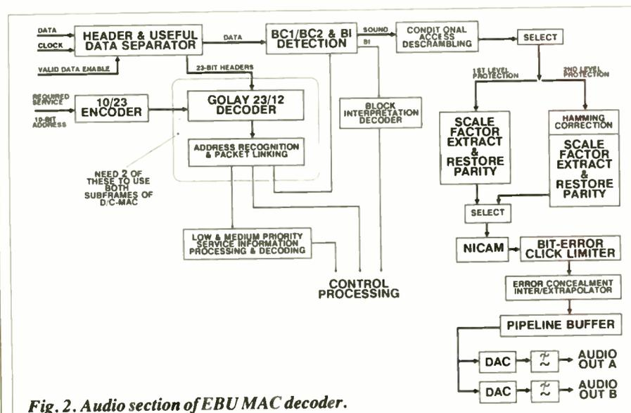
Fig. 2. Audio section of EBU MAC decoder.
