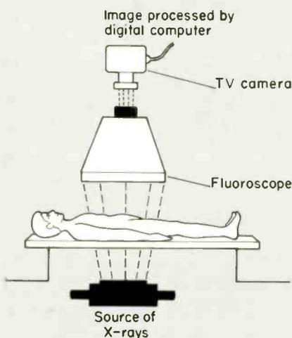
Fig. 8. Digital subtraction angiography images, from an X-ray source and displayed by a fluoroscope, are recorded by a camera, the image from which is processed by a computer
