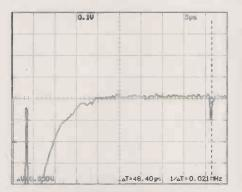
Fig. 8. Cable Talk 4 had the largest eddycurrent loss, the signal taking 25µs to decay into the noise floor.
