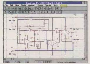
Fig. 1. Typical schematic screen when the parts bin is off, before processing so showing circles at junctions. Note the bubble-type help text on the Vectorise button.
