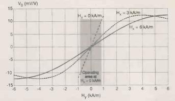
Fig. 7. Sensor output characteristic of ZMY20/ZMZ20. Sensitivity of the sensor can be controlled by applying auxiliary field  $H_x$ . This auxiliary field is necessary for sensor operation in a large field range,  $V_0$ =f( $H_y$ );  $H_x$ -parameter;  $V_b$ =const;  $T_{amb}$  -25°C.
