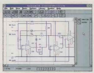
Fig. 2. Same screen with parts bin on, after processing, so many of the circles are now junction dots, indicating net formation. Note area taken up by parts bin.
