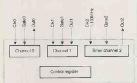
Block diagram of the pc's 8253 programmable universal counter/timer. Timer channel 2 counting is enabled when GATE2 is taken high.
