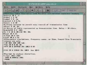
Fig. 5. Basic PSpice Net-List as used for Figs 3 to 7. This can be simulated using the evaluation version of PSpice.
