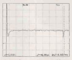
Fig. 16. In the same environment used for Fig. 15, the same length of coaxial cable picks up far less noise.
