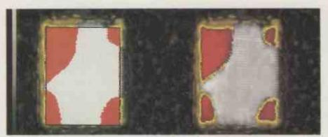
Fig. 2. Digital image analysis of a single UltraBoard image. Original image with 256 grey levels – here in pseudocolor – is reduced to two levels at left for analysis. 'Window' refers to whole area of the chip. 34.6% of whole die attach area is delaminated, as is 75.0% of the upper left quadrant of the chip. 'Large' gives percentage covered by largest delamination in each area; i.e., the large delamination in the top-left quadrant covers 19.5% of chip area.
