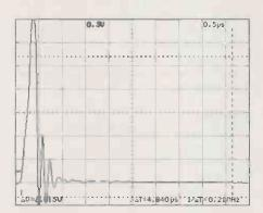
Fig. 13. Performance of a longer length of lawnmower cable -5m – with no damping and a ten times faster time base indicates that the frequencies involved are well outside the audio range.
