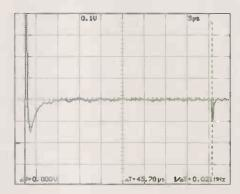
Fig. 5. Jenving Supra Ply 2.0 normally shows a small eddy current decaying within 10µs, but when twisted, the eddy current and time constant increase.
