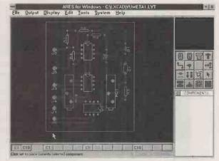
Fig. 11. Results of the Ares autorouter. Note the necked track at U1 putting this autorouter in category B.
