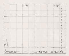
Fig. 11. RG58A/U coaxial cable again, but tested for series inductance. Compare this with Fig. 12.
