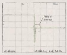
Fig. 1. Output from the 709 op-amp resulting from a test on a 1m length of mains cable. There is an initial positive excursion, followed by a short negative saturation period caused by the cable's reverse emf. This negative transition is the area of interest.
