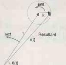
Fig. 4. Unmodulated carrier ωc rad/sec plus interfering carrier ωn rad/sec.
