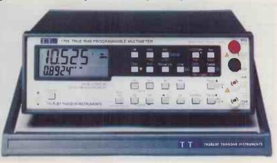
This high-performance bench multimeter could be yours in exchange for a good idea. Featuring a dual display, the 4.5-digit 1705 multimeter resolves down to  $10\mu V$ ,  $10m\Omega$  and  $0.1\mu A$  and has a basic dc accuracy of 0.04%. Frequency measured is 10Hzto 120kHz with an accuracy of 0.01% and resolution to 0.01Hz. Capacitor and true rms measurements are also featured.
