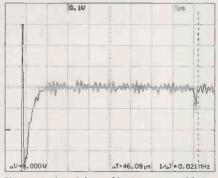
Fig. 15. Noise pickup of lawnmower cable in a noisy environment, length 5m.
