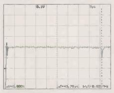
Fig. 2. Reference waveform. The nearer the cable test comes to this shape, the lower the inductance, capacitance and cross-sectional eddy currents.
