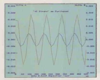
Fig. 1. Measured result of 42-strand as-purchased cable tested via a Douglas Self 50W amplifier.
