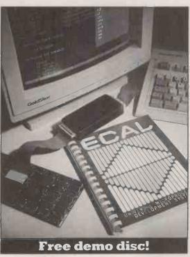
The PC based ECAL hardware emulator is fully integrated with the assembler. Connection is made to the target through the eprom socket so a **single** pod
