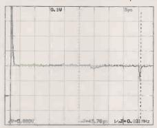
Fig. 7. Eddy currents are not a problem here, but Heywire gave the highest series inductance. Overshoot decay was short though, at 4µs.
