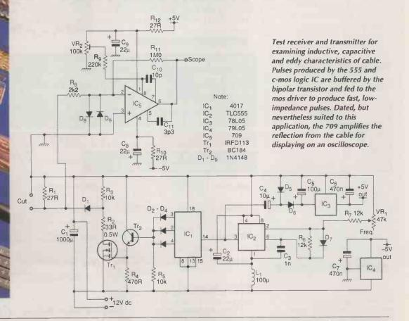
At the termination of the current pulse a wide band op.amp. amplifies any low level decay effects due to induced eddy currents in the wire cross section or to polarisation signals in the insulating material – if they occur.
