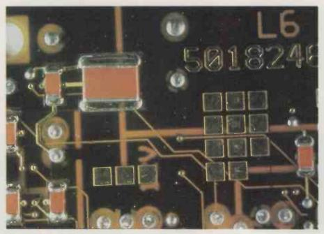
Fig. 3. Optical photograph of ceramic chip capacitor mounted on board.
