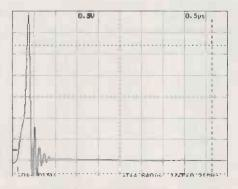
Fig. 14. RG58 coaxial cable performance for a 5m length with damping removed.
