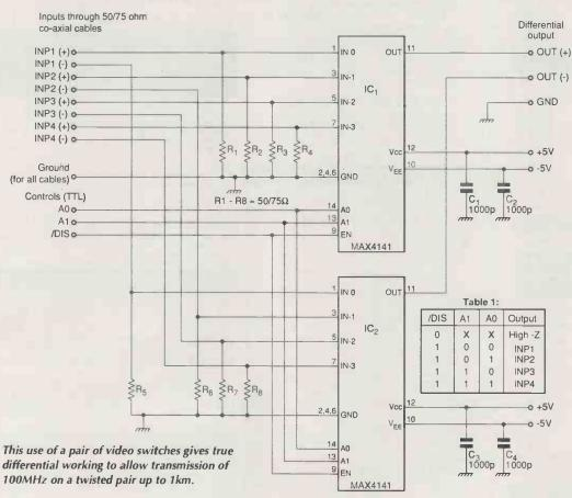
his four-channel, differential input/output video switch was built for a computer-controlled security system, in which one of the 100MHz video signals had to be selected
