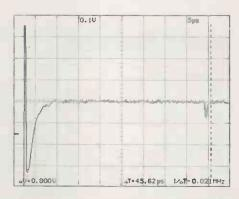
Fig. 17. Some hi-fi enthusiasts advocate the use of oxygen-free copper in audio cables. Here, lawnmower cable was injected with salt water, left for three days and tested again. No change is apparent in these tests.
