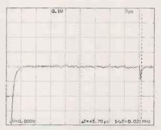
Fig. 10. Cleanest of all – plain and simple RG58 coaxial cable. There is no overshoot and eddy currents in the braid decayed within 7µs.
