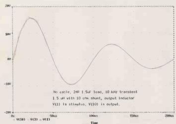
Fig. 3. Simulated behaviour of typical amplifier output configuration when driving into a capacitive and shunt resistor load. Voltage V(1) is taken as the location of the feedback connection.
