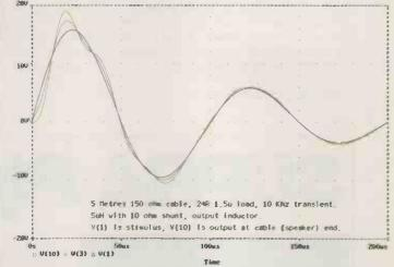
Fig. 6 Simulation of Identical configuration as Fig. 3, except for increased value of amplifier output inductor to  $5\mu$ H. This distortion should be clearly audible on transients.
