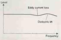
Fig. 3. Frequency response of a solid-core cable with plastic sheath. In listening tests the response dip is audible.
