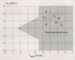
Fig. 6. Safe operating area of ZMY20/ZMZ20 magnetoresistive sensors.  $H_{x(tot)}$  is  $H_x+H_{d'}$  ambient temperature is -25°C and  $H_d$  is the disturbing field.
