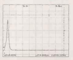
Fig. 12. Inductive spike resulting from Heywire shows that it performs less well relative to coaxial cable in this test.
