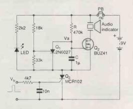
Simple alarm circuit for both visual and audible output.
