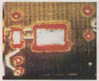
Fig. 4. Effect of electronic gating to limit internal level being imaged: when gating is near top surface, multilayer ceramic chip capacitor shown in Fig. 2 displays only merest suggestion of an internal crack at its lower edge.
