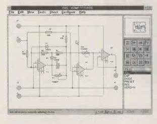
here are two parts to Propak, which are There are two parts to require windows. Isis Illustrator+ is the schematic drawing and capture part of this program. It runs on a 386 pc running Windows 3.1 with 2Mbyte of ram, but more memory than this is recommended in the manual. It was not satisfactory on a 286 with 2Mbyte of ram.
