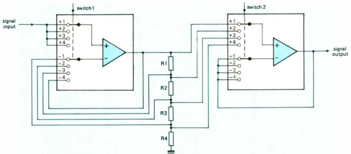
Fig.2. If independently-controlled, four-position switches are introduced at the op-amp inputs, the gains of the left-hand and right-hand op-amps can be independently set to one of four values.
