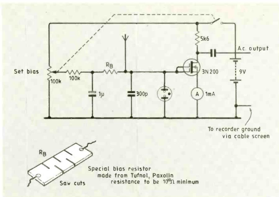
Fig.4. Simple portable electrometer. The bias adjustment is necessary to compensate for atmospheric changes.
