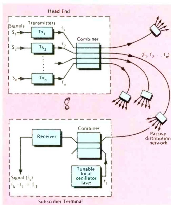
**Fig.7 (left).** Illustration of the functional requirements of a coherent fibre-optic link using the heterodyning principle.
