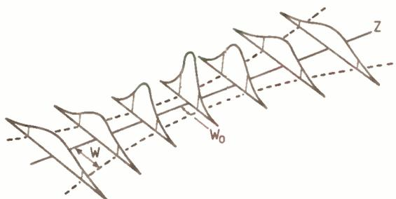
Fig.1: Propagation through a waist of a fundamental mode Gaussian beam. The intensity distribution along any cut perpendicular to the propagation axis is a Gaussian function of the distance from the axis (Adapted from Fig. 2 of reference 3).
