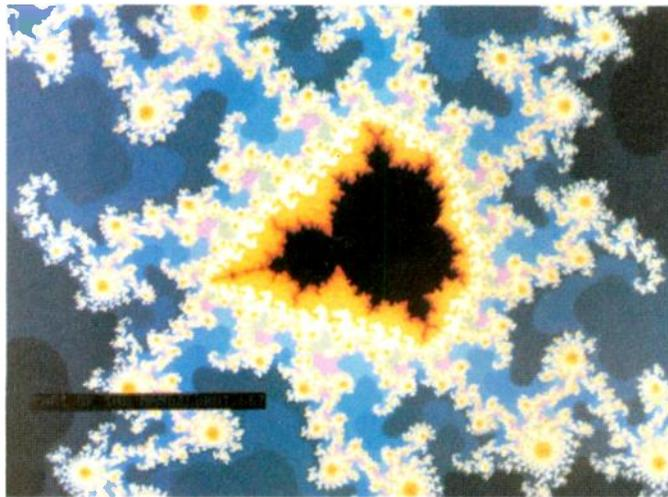
**A Video Graphics Array 16-colour display. Although only 16 are available, they can be chosen from 262144 and subtle effects are possible. The resolution is 640 horizontally by 480 vertically, and this is the only display mode available having equal pixel "size" both ways.**
