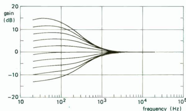
Fig.4. Example frequency response characteristic. Gain control range is +15dB to -12dB in 3dB steps.
