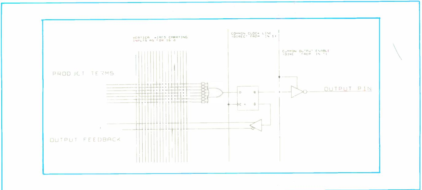
Fig.9. One output of the 16R8 pal.
