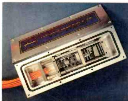
**Fig.5. Packaged 16-channel single-mode fibre WDM component. The device features a grating as wavelength dispersive element and a lithium-niobate concentrator.**
