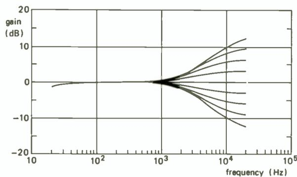
**Fig.6.** Example frequency response. Gain control range is +12dB to -12dB in 3dB steps.
