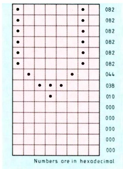
**Fig.1. An 8x14 character array such as that supplied with the EGA. 9-pixel wide arrays are specified by the same byte, the video display circuits provide the extra pixel. MDA characters occupy the top 11 rows of 14, leaving row 13 for underline. The position of the underline is programmable and can also be displayed by the EGA in graphics mode.**
