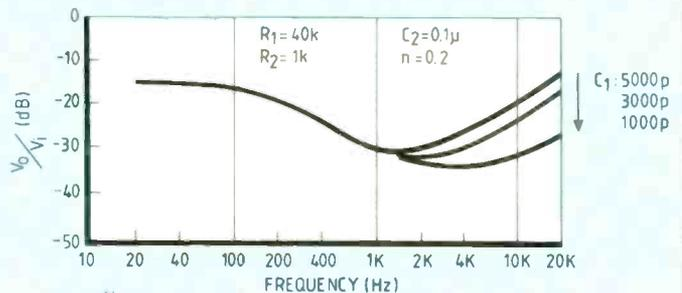
a.  $V_o/V_i$  - f curves for different values of  $C_1$
