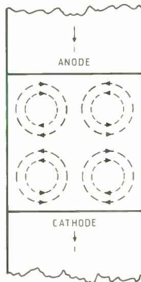
Fig.3. Circulation in liquid metal cell.
