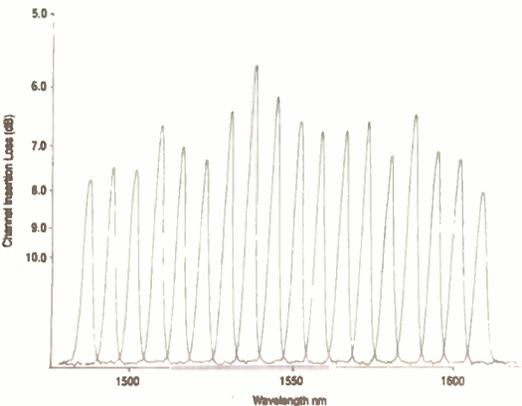
Fig.6. Passband characteristics for 18 channels of the component shown in Fig.5.
