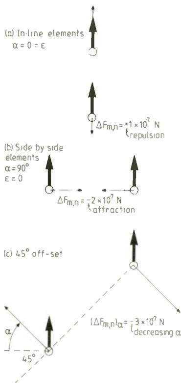
Fig.2. Principal Ampere forces between a pair of current elements.
