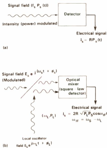
**Fig.1. Principle of direct-detection optical communications (a) and principle of coherent optical detection (b).**
