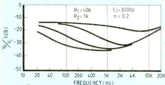
b.  $V_o/V_i$  - f curves for different values of  $C_2$
