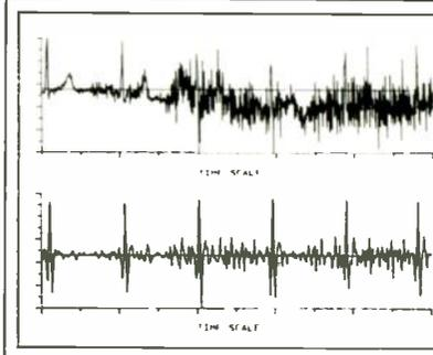
One of the best ways of looking at stress in pilots is to monitor the electrical signals that control the heart beat. While the pilot is not moving the signals are easy to measure but as soon as any movement is made, the signals going to the large muscles in the upper body swamp those detected from the heart.
