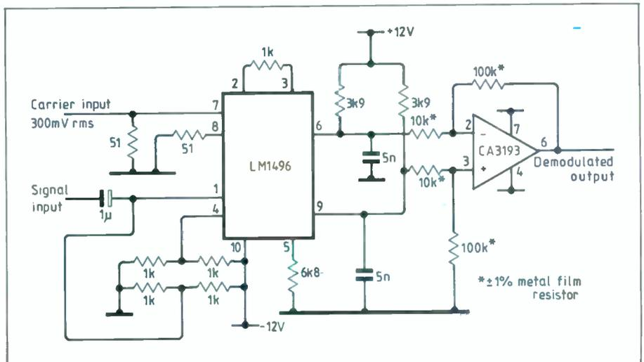
Attenuation of  $2f_c + 2f_s$  products is greater than 60dB. As shown, the circuit is suitable only for low frequencies but if the op-amp is replaced by a CA3450 for example, bandwidth is greatly increased; note that the 3450 and 1496 in this case would both be powered
