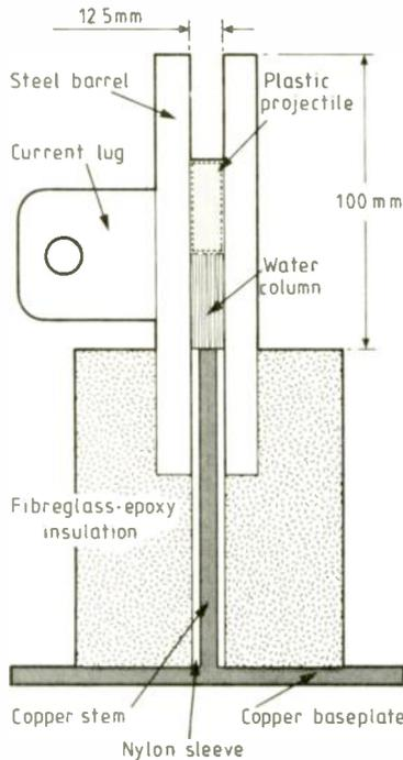
Fig.6. Miniature coaxial water-arc gun.
