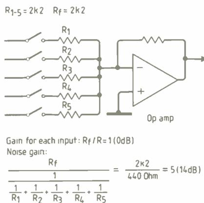
Fig.11. Noise performance of the inverting summing amplifier with five inputs.
