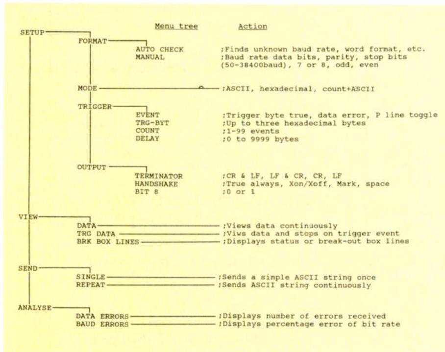
Menu options for the DA100 are displayed on the oscilloscope screen.
