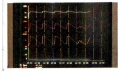
Real-time telemetry is used to monitor racing-car performance. Cranfield's Microsystems Design Group has developed a telemetry link in the form of a UHF transmitter that sends data from sensors within the car to a PC.
