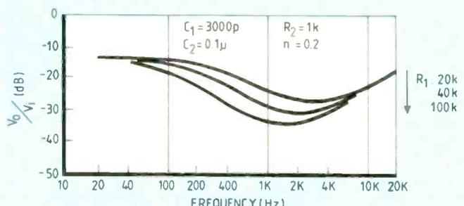
e.  $V_o/V_i$  - f curves for different values of  $R_1$
