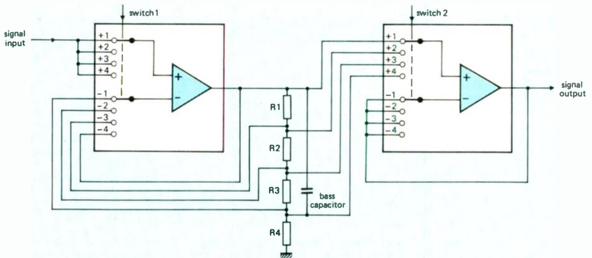
Fig.3. Inserting a single capacitor in the feedback loop of the left-hand op-amp stage makes it possible to control the low-frequencies. Low-frequency gain is determined by the resistors and the effective frequency range by the resistor and capacitor values.
