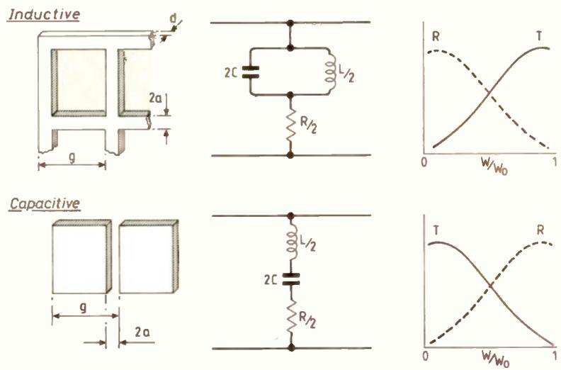
**Fig.6:** Inductive and capacitive meshes for use as quasi-optical filters or filter elements. Also shown are their lumped element equivalent circuits and their normalized filter transmission curves. (Adapted from C. Cunningham, Ph.D. thesis, University of London, 1982).
