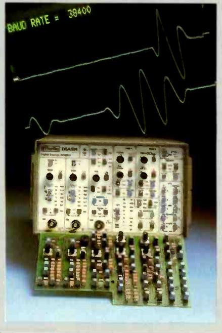
○ Increasingly complicated nature of multiprocessor systems makes analysis by conventional logic analysers extremely difficult, if not impossible, according to Dolch Logic Instruments. Their latest model M128 incorporates a twin-slot capability that allows two cards to be linked together and analyse data on two independently clocked and synchronized processors.
