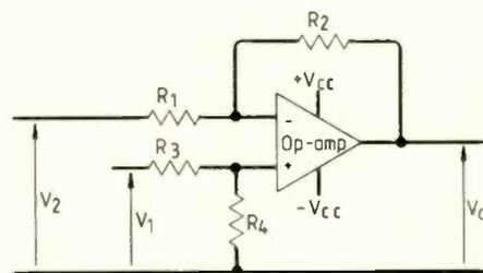
Fig.1. Standard differential amplifier, in which common-mode rejection is heavily dependent on resistor matching.
