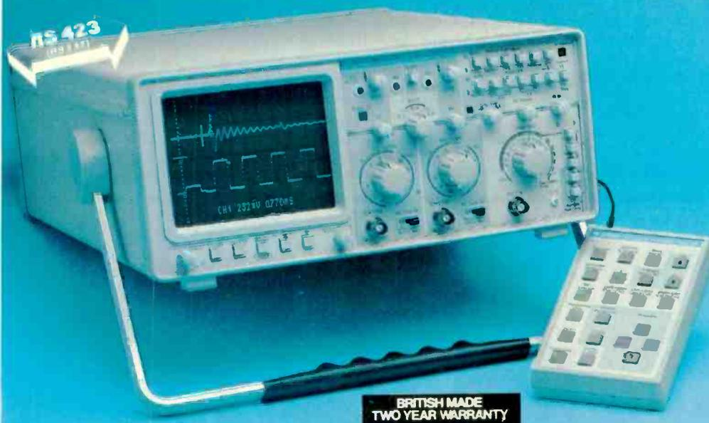
The Gould 1425 Digitising Storage Oscilloscope allows detailed comparison of active with stored waveforms, up to a frequency of 20MHz. Five reference waveforms can be held in the non-voltage memory.
