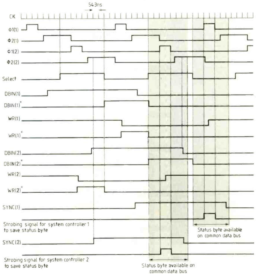
memory and i/o control signals. The multiprocessor system controller combines these control signals to produce common bus-control signals. Overlapping of combined signals can cause disturbed system operation. To prevent this, signals from each system controller are activated only during
