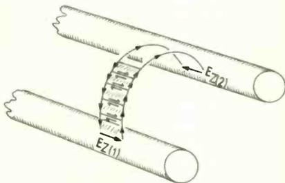
Fig. 7. This illustrates that if there is a longitudinal component of E field, the only place where it is significant is on the conductors.
