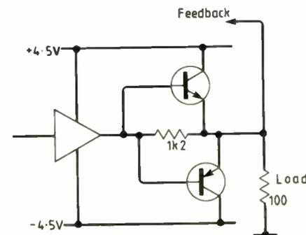
**Fig.3. Final version of the combiner. The op-amp alone supplies the load current for outputs of less than 700mV.**
