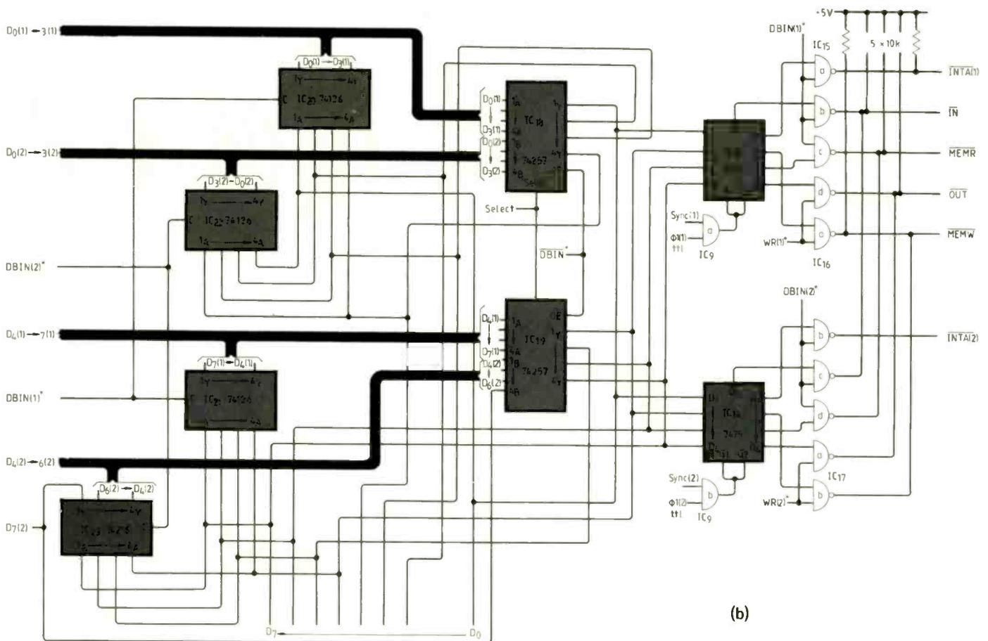
**Fig.1. Processor control signals modified to allow two processors to operate together. In this synchronous system,  $\phi 1$  and  $\phi 2$  clocks of each microprocessor are shifted in relation to each other so that the processors access the bus alternately.**
