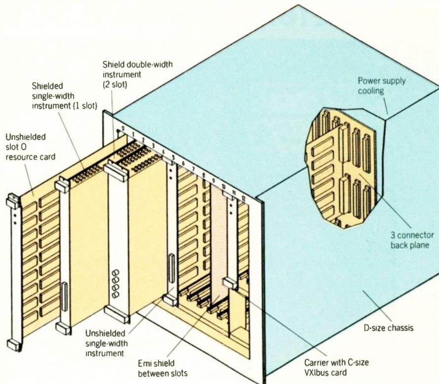
*Shown here is a VXIbus mainframe used for internal product development at Hewlett Packard Co. Also shown is a prototype instrument module and a carrier assembly that allows standard B size VME modules to be integrated into C size mainframes.*
