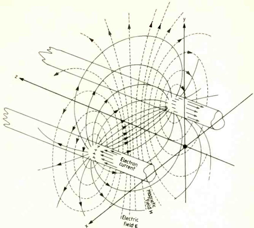
Fig. 2. The fields, currents and coordinate system for the parallel line shown in detail.
