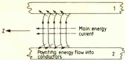
Fig. 8. The losses in the conductors 'distort' field direction, so that there is a net movement of energy current into the conductors from the field (seen by the direction of the Poynting vector).
