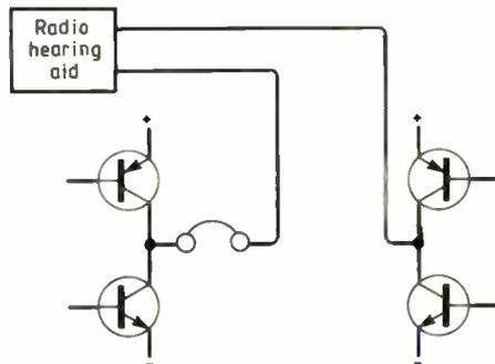
**Fig.2. Modifying a radio hearing aid using a full bridge transposer output stage.**
