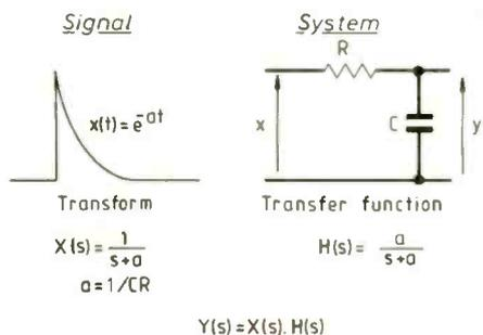
Fig.2. The signal and system are matched in the sense that the system impulse response is identical to the characteristics of the signal.
