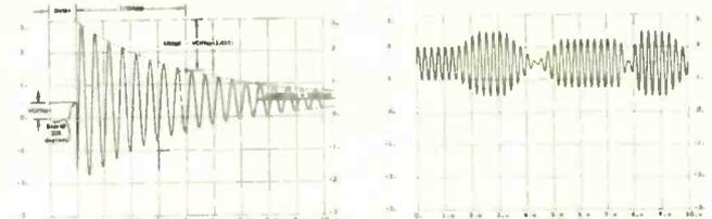
Internal generator programmed to produce sine wave with exponential amplitude decay
