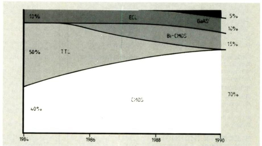
NEC's asic production output trends show c-mos replacing t.t.l. by 1990.
