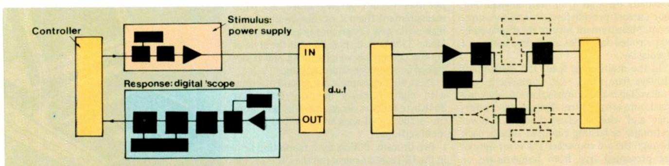
Simple stimulus response test using standard instrumentation (left) has limited adaptability and an excess of features. In the 6954A setup (right) the relationship between cards is not fixed and is determined by the test designer. Features can be adapted by 'rewiring' the blocks, and as the selection of i/o cards is determined by the test designer unnecessary functions can be omitted.
