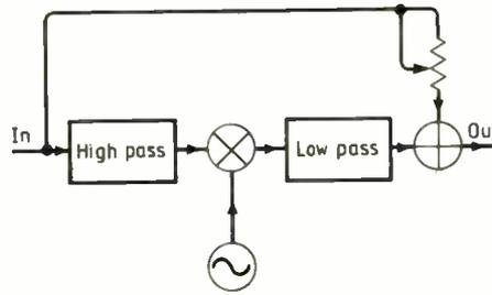
**Fig.1. Transposer-type hearing aid. Sound components above 4kHz are superimposed on the 0-4kHz components. This treatment improves intelligibility by adding emphasis to speech consonants and other sounds.**
