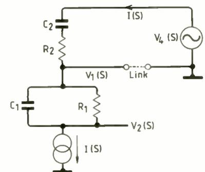
Fig.2. Equivalent circuit of the sine-wave oscillator of Fig.1. With the link closed, the circuit assumes inverters having infinite gain; practical devices have a finite gain (link open).
