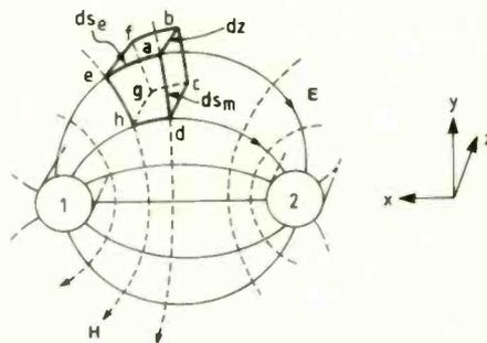
Fig. 3. The key to handling the field approach to lines means constructing a small volume in the space around the line, bounded by the E field lines, the H field lines and direction of propagation, z.
