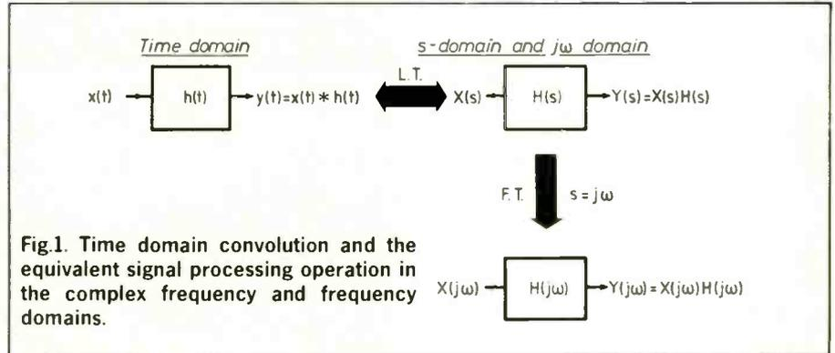
Fig.1. Time domain convolution and the equivalent signal processing operation in the complex frequency and frequency domains.
