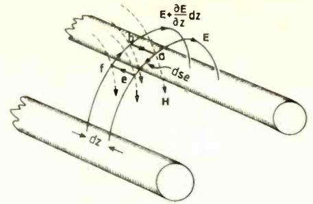
Fig. 6. Illustrated is the similar  $\mathbf{E}$  field curl loop. The result this time is the magnetic flux rate of change through the loop. This is used to derive the second Telegrapher's Equation.
