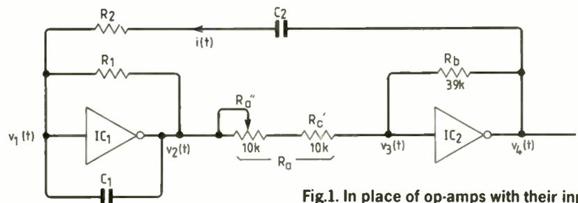
Fig.1. In place of op-amps with their inputs biased at half the supply voltage, the circuit uses c-mos inverters.
