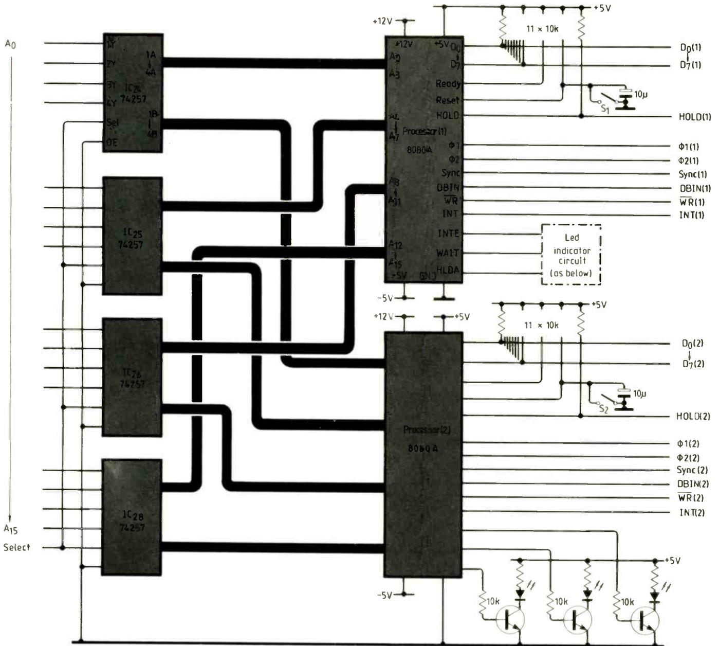
affects the duration of activation of the output signals from both system controllers. This is achieved in this design by control-signal alignment modules which act upon  $\overline{\text{DBIN}}$  and  $\overline{\text{WR}}$  signals of each processor, and product  $\overline{\text{DBIN}}^*$  and  $\overline{\text{WR}}^*$  modified signals. These signals are activated only during the bus time slot of their associated processor.
