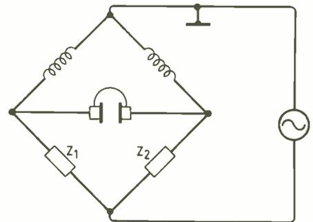
Tightly-coupled inductive ratio-arm bridge circuit, 1928: Blumlein's first invention. The coils were bifilar-wound.
