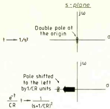
Fig.5 The Laplace transform of the ramp function  $t \rightarrow 1/s^2$  gives rise to a double pole at the origin of the  $s$  plane. The frequency shifting rule has the effect of moving the poles to the left by  $1/CR$  units.
