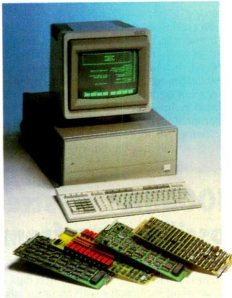
seventies, the 6954A has eight slots, expandable in 16-socket frames to 120, a 300 series computer, 1Mbyte of ram and a 20Mbyte disc, whilst running Basic 5.0 and maintaining compatibility with the previous series software. The computer, actually a 310 series with 68010 c.p.u., replaces the 68000 series 300, which in turn supersedes the series 200 introduced six years ago.
