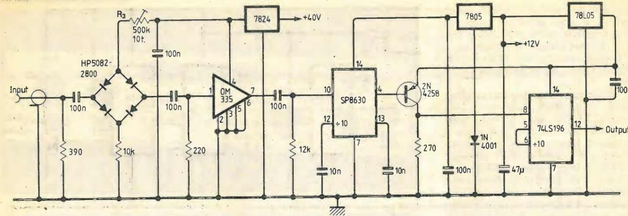
Fig. 9. 500MHz prescaler. R<sub>3</sub> should be adjusted for optimum sensitivity at 500MHz. To reduce stray capacitance it is important to use a ground plane on the circuit board and to use the i.c.s without sockets.
