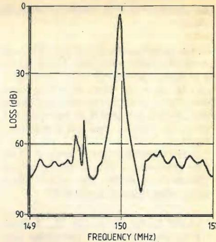
Fig. 5. Measured frequency response of 149.950MHz s.a.w. resonant filter with a bandwidth of 30kHz and insertion loss 3.5dB.
