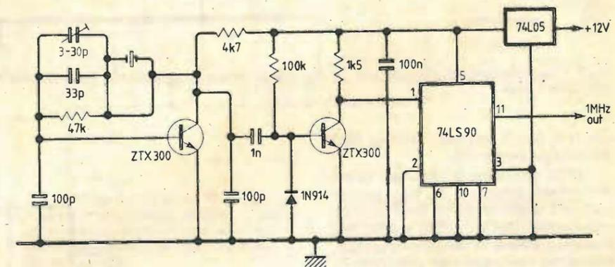
Fig. 4. External crystal oscillator.
