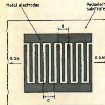
A: Uniform interdigital transducer used for launching surface acoustic waves on a piezoelectric substrate. This transducer has a  $\sin x/x$  frequency response
