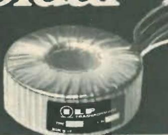
We use advanced winding technology to make our toroidal transformers. They have only half the weight and height of their laminated equivalents and are appreciably more efficient. Our toroidals cost virtually the same as the older types which they are rapidly replacing. Induced hum is reduced by a factor of ten. Supplied with rigid mounting kit with centre bolt, steel and neoprene washers.
