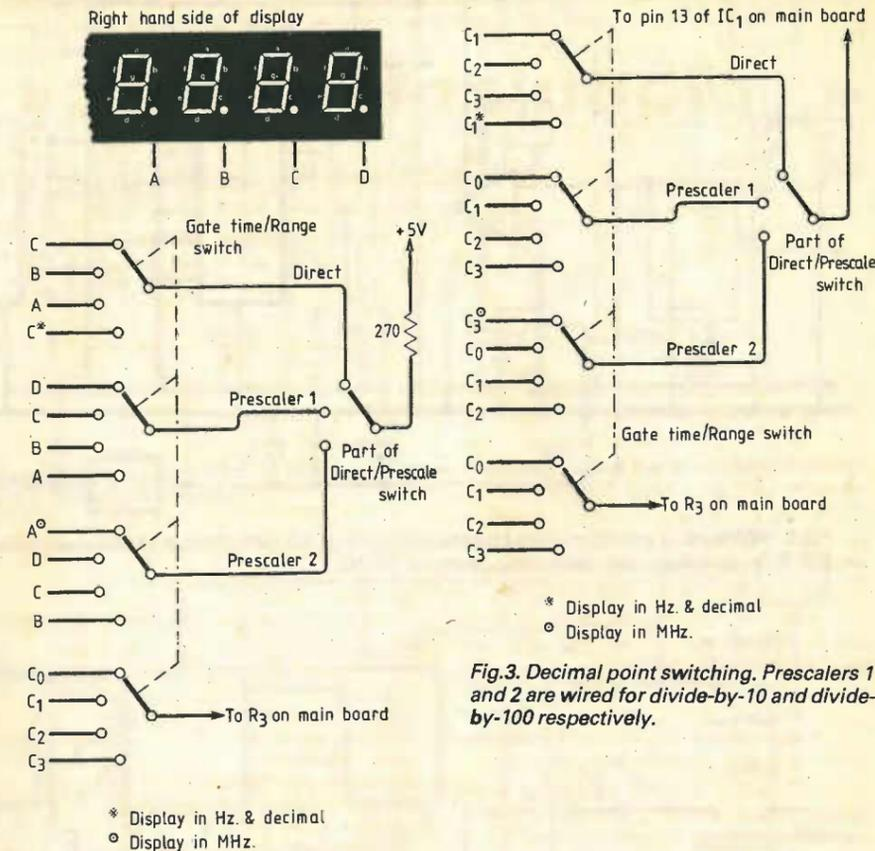
Fig. 3. Decimal point switching. Prescalers 1 and 2 are wired for divide-by-10 and divide-by-100 respectively.
