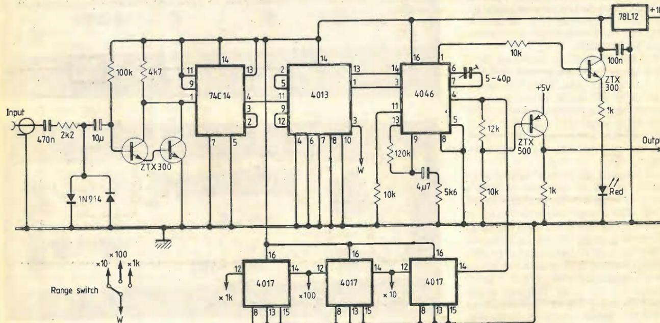
Fig. 10. Phase-locked loop frequency multiplier. A secondary winding of 15V at 200mA is needed for the 18V supply, but the 5V rail can be taken from the main counter module.
