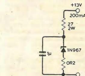
Fig. 3. (a) Test circuit to measure dynamic voltage and current,  $F = 18\text{kHz}$ , (b) Waveforms across 0.2Ω resistor, 3V (top) and pk-to-pk.
