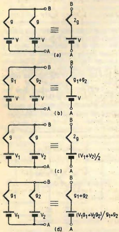
Fig. 5. Cells connected in parallel (a), (b) and (c) show that the voltage across the terminals is the mean of e.m.f. of the two cells (case d) is not so simple) In each case internal conductances are added to give total conductance.
