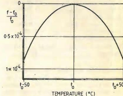
Fig. 6. Frequency of s.a.w. oscillator on quartz as a function of temperature variation about reference temperature ( $t_0$ ).
