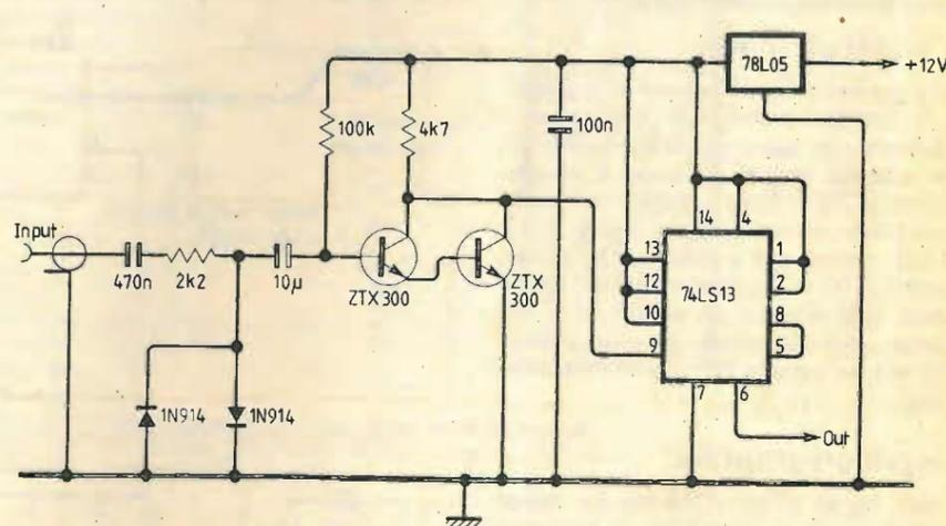
Fig. 7. Simple preamplifier for input B of the 7216.
