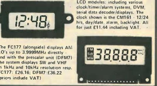
The FC177 (alongside) displays AM LO's up to 3.9999MHz directly - and with the prescaler unit (DFM7) the system displays SW and VHF in 1kHz and 10kHz resolution resp. FC177: £26.16; DFM7: £36.22 (prices include VAT)
