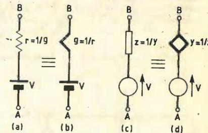
Fig. 3. Batteries of e.m.f. V in series with its internal resistance (a), internal conductance (b), and generators of e.m.f. V with internal impedance (c), and internal admittance (d). (Batteries and generators are equivalent).
