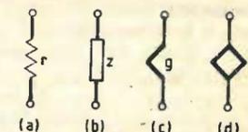
Fig. 2. Symbols used for resistor or resistance (a), impedor or impedance (b), conductor or conductance (c), admittor or admittance (d).
