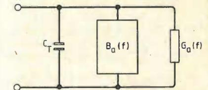
C: Lumped equivalent circuit of interdigital transducer.
