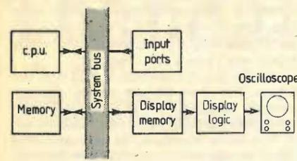
The system uses two standard DAC0800 converters to provide X and Y inputs to the oscilloscope and, as can be seen from careful examination of the display, these are just adequate. It was found that continuous intensity modulation is not necessary. A simple 16-input OR function detects the address 0,0 and blanks the display.
