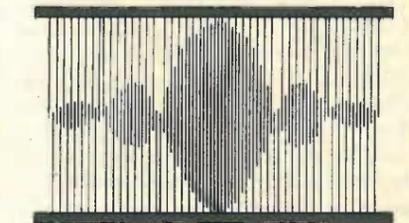
B: Overlap weighted interdigital transducer. The frequency response is determined by the weighting pattern.
