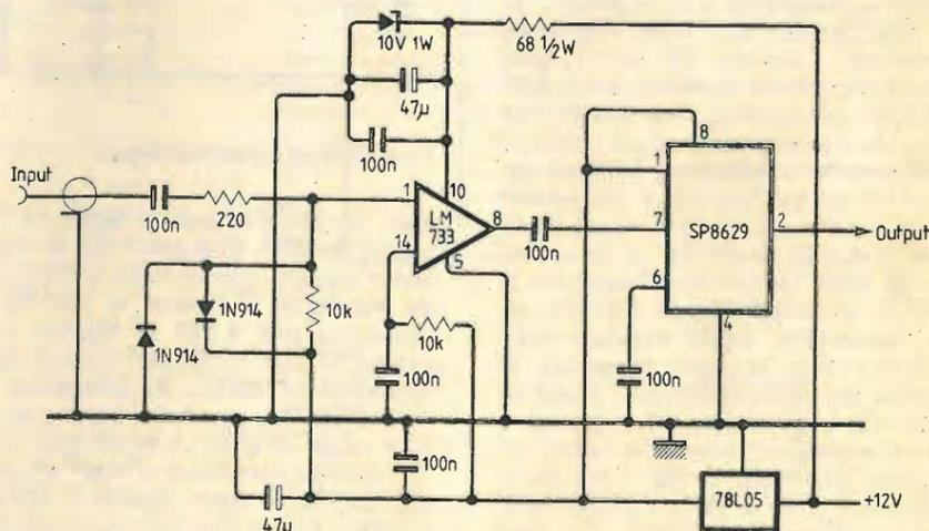
Fig. 8. 200MHz prescaler with an input impedance of about 2kΩ.
