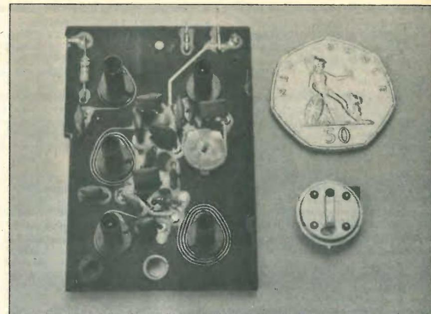
Fig. 2. Comparison of conventional LC (left) and surface acoustic wave (right) television i.f. filters showing the considerable size reduction.
