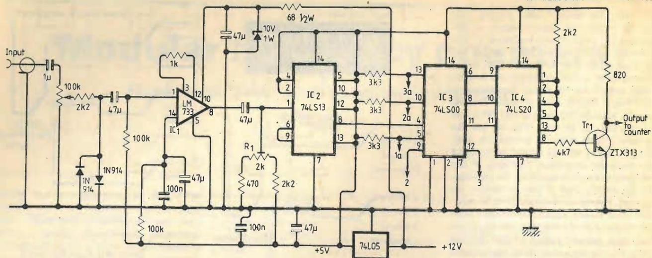
Fig. 5. 10MHz input amplifier. Note that the output must not be fed to the 7216 unless power is applied to the counter. R<sub>1</sub> is adjusted for optimum sensitivity and reliable triggering at 10MHz.
