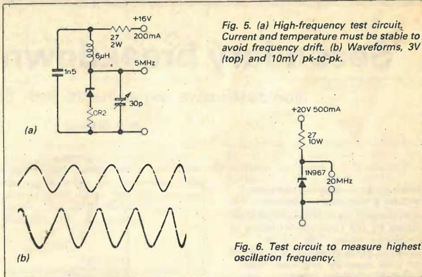
Fig. 5. (a) High-frequency test circuit. Current and temperature must be stable to avoid frequency drift. (b) Waveforms, 3V (top) and 10mV pk-to-pk.
