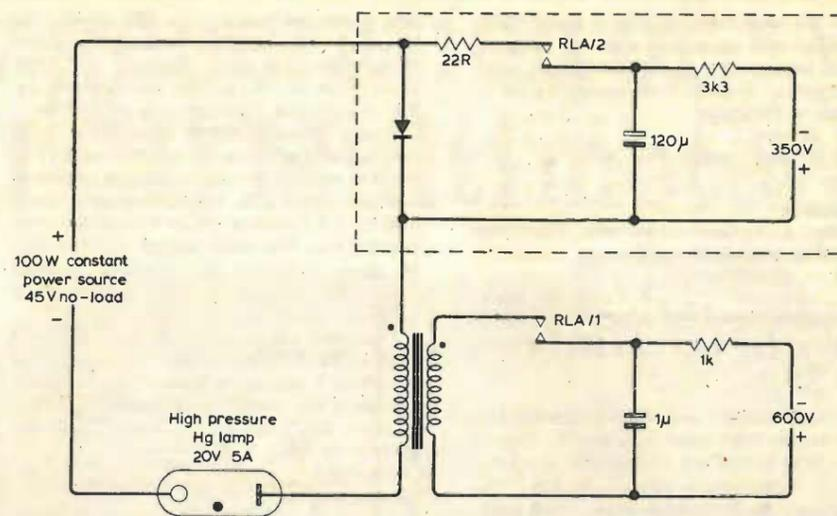
Basic e.h.t. ignition circuit for mercury lamp as used in u.v. oscillographs, with supplementary h.t. source (in broken-line box). All resistors serve as current limiters. RLA is designed to operate repeatedly until ignition is obtained.
