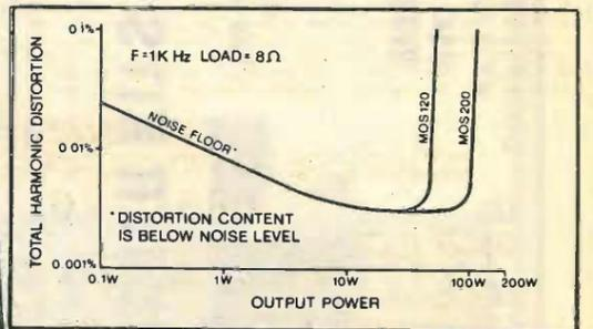
Load impedance both models 4Ω-∞ Input sensitivity both models 500mV Frequency response both models 15Hz-100KHz - 3dB
