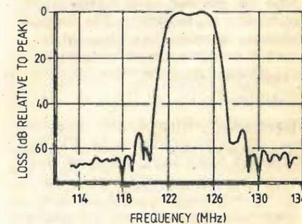
Fig. 3. Measured frequency response of 124MHz s.a.w. transversal filter showing low ripple and very steep sides. The bandwidth is 3.7MHz.
