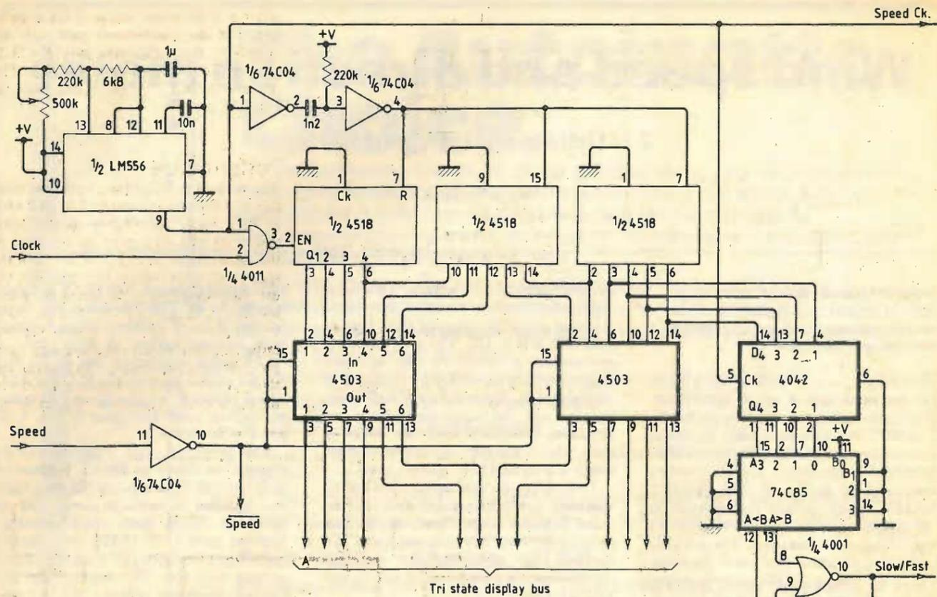
Fig. 10. Wind speed measuring circuit.
