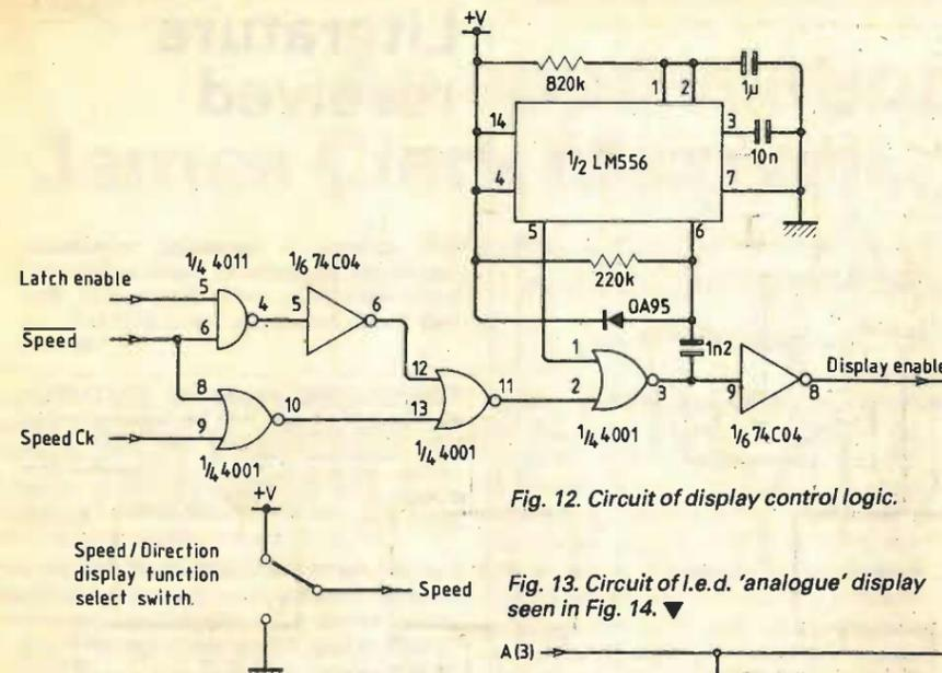
Fig. 12. Circuit of display control logic.
