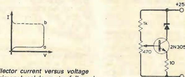
Fig. 1. Collector current versus voltage showing primary breakdown at a, followed by secondary breakdown at b. Region b exhibits negative resistance.
