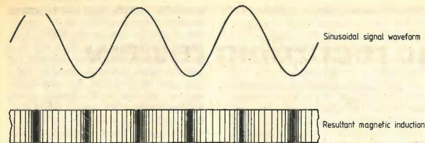
A sinusoidal signal produces a sinusoidal distribution of flux along the tape
