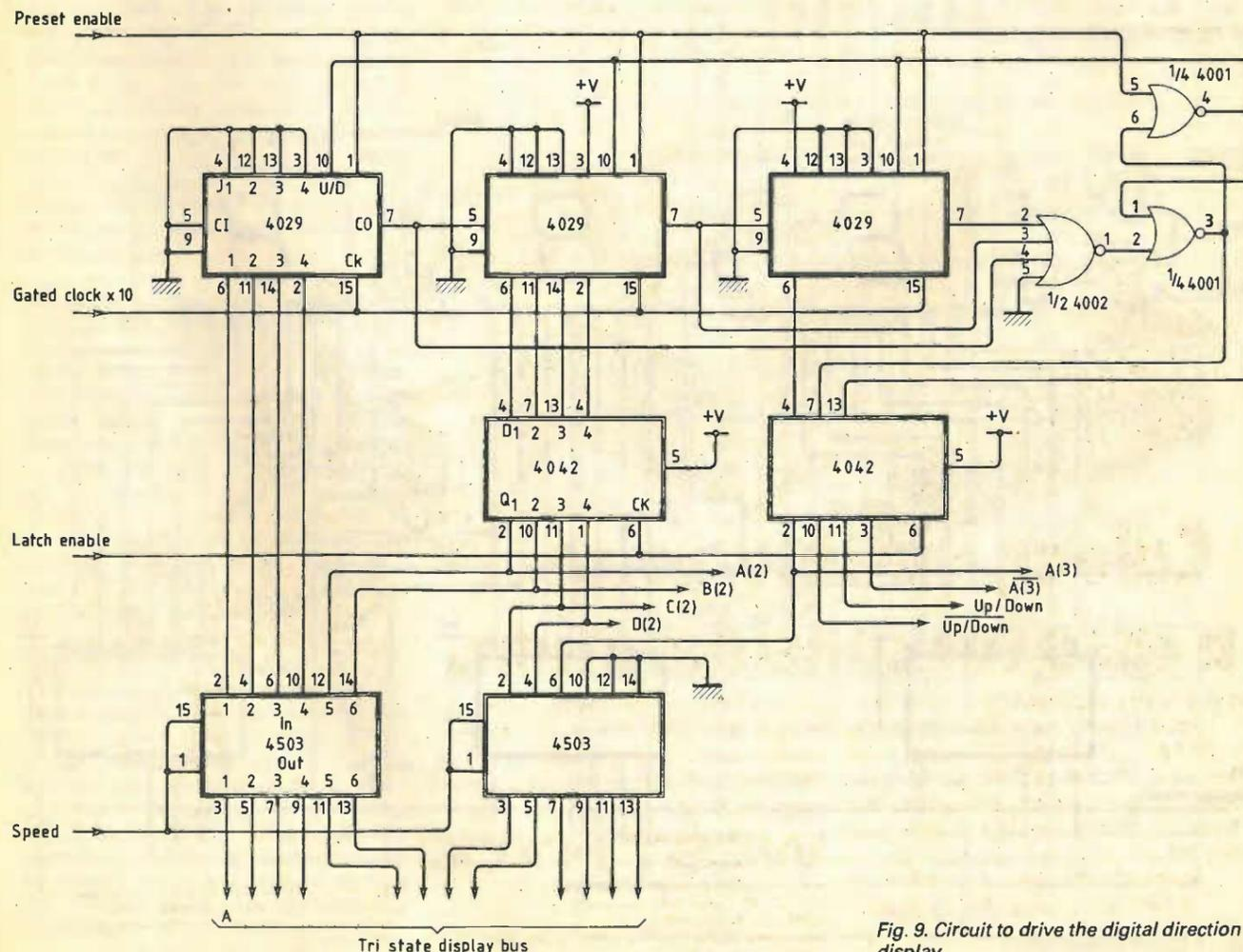
Fig. 9. Circuit to drive the digital direction display.
