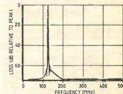
Fig. 4. Measured wideband frequency response of 124MHz s.a.w. transversal filter highlighting the excellent stopband properties of these filters.
