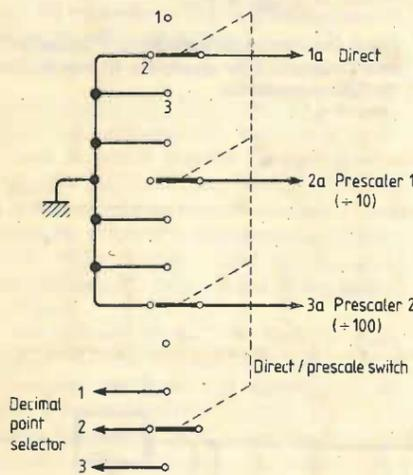
Fig. 6. Enable/disable switching for the prescaler signals.
