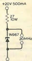
Fig. 6. Test circuit to measure highest oscillation frequency.
