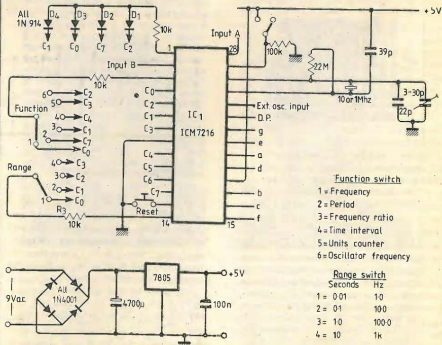
Fig. 2. Main counter module and internal oscillator connections. Pin 1, via D<sub>1</sub> to D<sub>4</sub>, selects display blanking, display test, external oscillator enable, and 1MHz external oscillator respectively. Break-before-make switches should be used for function and range, non-latching push-to-make for reset and display test, and single-pole toggle for hold and display blank. The voltage regulator must be insulated and mounted on the chassis.
