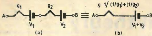
Fig. 4. Two cells represented by pure voltage sources in series, each with internal admittance (a). When the cells are connected in series, (b) + (a). Cell voltages add directly; the total admittance of the battery is the reciprocal of the sum of reciprocals of the separate internal admittances.
