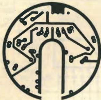
Fig. 15. Printed-board layout of mast-head unit.
