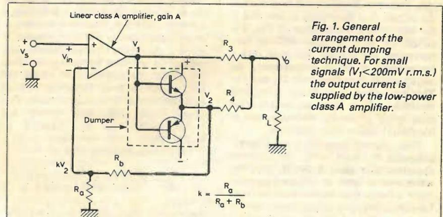
Fig. 1. General arrangement of the current dumping technique. For small signals ( $V_1 < 200\text{mV r.m.s.}$ ) the output current is supplied by the low-power class A amplifier.
