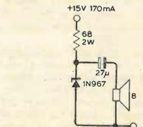
Fig. 4. Audio oscillator with an efficiency of 10% at 1kHz.
