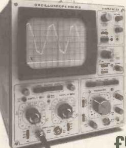
Trace Oscilloscope with delayed sweep. DC-50MHz Sensitivity 5mV-20V/cm Time base range 0.1uS-2.0S/cm with x5 horiz mag to 20nS/cm. Delay ranges 7 decade steps 100ns-1S with fine control CRT screen 8 x 10cm Full XY using ch II as x input, bandwidth 4° MHz. Z input. Delay line allows viewing of leading edge. Vertical overscan indicated by 2
