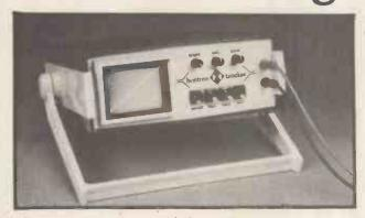
This easy to use test instrument displays shorts, opens, and leakage in solid state components. Check diodes, unijunctions, bipolars, Darlingtons, J-FET's, MOS FET's, LED's, electrolytics and IC's . . . IN CIRCUIT!
