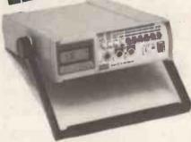
DMM with true RMS on AC volts and current DC volts 200mV-1KV,  $10\mu V$  resolution AC volts. 200mV-750V,  $10\mu V$  resolution. DC/AC current  $200\mu A-2A$ ,  $0.01\mu A$  resolution resistance  $200\Omega-20M\Omega$ ,  $0.01\Omega$  resolution. Also reads dB direct referenced to 16 stored impedances. Conductance ranges 2mS and 200nS. £199 mains model £239 mains battery.
