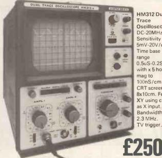
HM312 Dual Trace Oscilloscope. DC-20MHz. Sensitivity 5mV-20V/cm Time base range 0.5uS-0.2S/cm with x 5 horiz mag to 100nS/cm. CRT screen 8x10cm. Full XY using chll as X input. Bandwidth 2.3 MHz. TV trigger.
