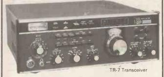
Ham Bands with 1.5-30 MHz receive with built-in 150 MHz frequency counter plus option of 0-1.5 MHz receive and/or any transceiving application 1.8-30 MHz.
