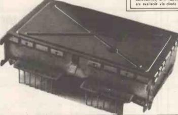
UM1181 VHF band 2 VARICAP TUNERHEAD
