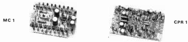
**CPR 1 — THE ADVANCED PRE-AMPLIFIER.** The best pre-amplifier in the U.K. The superiority of the CPR 1 is probably the disc stage. The overload margin is a superb 40dB, this together with the high slewing rate ensures clean top, even with high output cartridges tracking heavily modulated records. Common-mode distortion is eliminated by an unusual design. R.I.A.A. is accurate to 1dB, signal to noise ratio is 70dB relative to 3.5mV, distortion < 0.05% at 30dB overload 20kHz.
