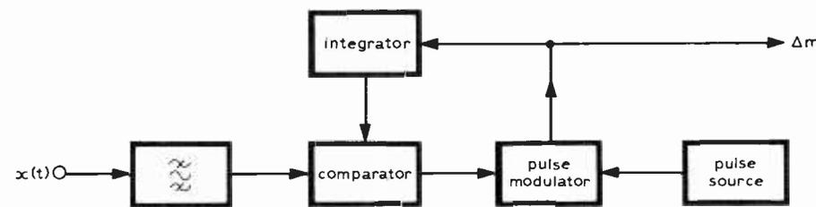
Fig. 13. The basic delta modulator.
