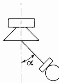
The effect of off-axis placement is to reduce the deviation of the h.f. carrier, and, as Mr Moir points out, this has no effect on the frequencies of the sidebands, although it reduces their apparent level. This indicates that the microphone should be placed on the axis of the loudspeaker unit radiating the modulating (l.f.) signal, if an unambiguous reading is to be obtained.
