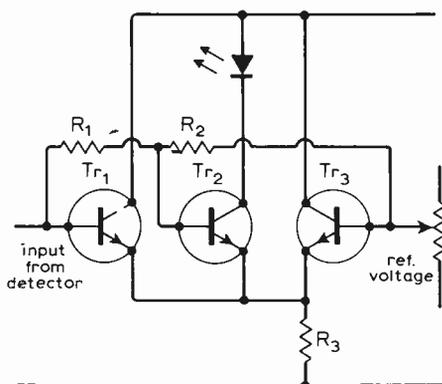
Fig. 2. New circuit permits tuning for maximum brightness of a single lamp by addition of a third transistor.
