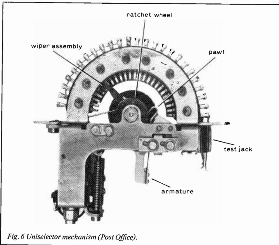
Fig. 6 Uni-selector mechanism (Post Office).
