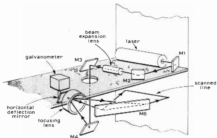
Fig. 1. Mechanical layout of the optical scanner.
