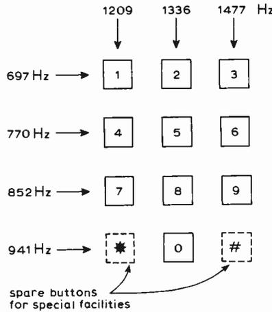
Fig. 2 Layout and frequency code for a push-button telephone.
