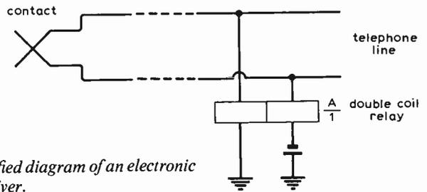
Fig. 12 Simplified diagram of an electronic dial pulse receiver.
