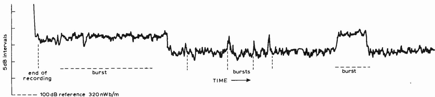
Fig. 2. Tone bursts revealed as the result of narrow band analysis.
