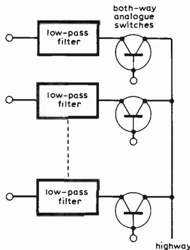
Fig. 11 Much simplified diagram of time division multiplex switch.
