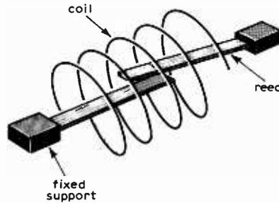
Fig. 10 Principle of operation of a reed relay.
