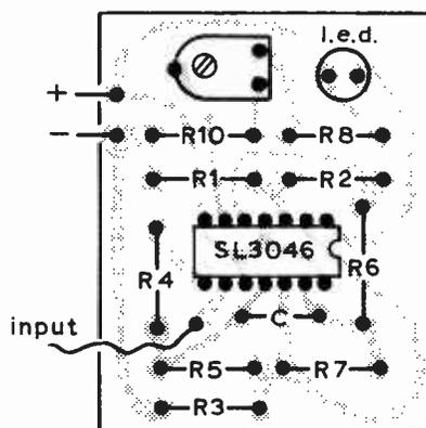
Actual-size printed board for circuit of Fig. 3, and pin connections for the i.c.
