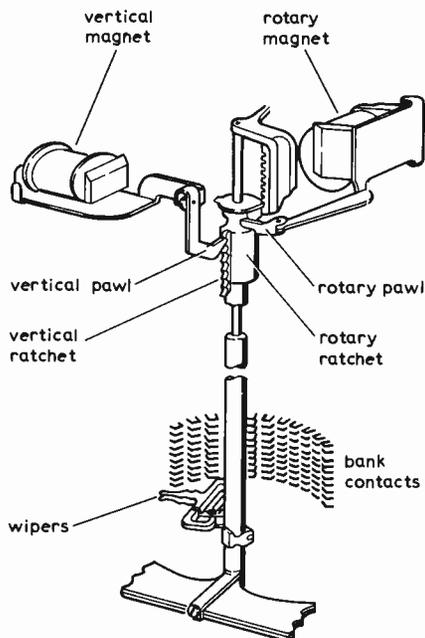
Fig. 5 Strowger two-motion selector mechanism.
