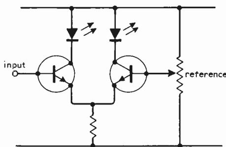
Fig. 1. Conventional two-lamp indicator requires adjustment of receiver tuning for equal brightness.
