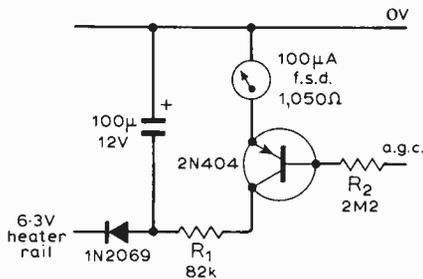
which supplies current to an S or tuning meter. The negative voltage required to power the emitter follower is obtained very simply by half-wave rectification of the 6.3V heater rail in the receiver. The circuit fits easily on a small piece of circuit board, which itself can be supported by the terminal posts on the back of the meter.
