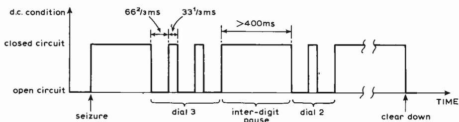
Fig. 1 Signalling conditions from a dial telephone.
