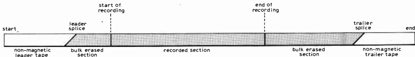
Fig. 1. Expected tape format for new tape on a battery recorder.
