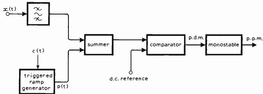
Fig. 8. The p.a.m. is dispensed with in this system.
