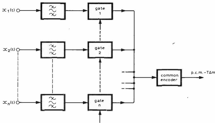
Fig. 12. Multi-channel operation in p.c.m. using time-division multiplex.
