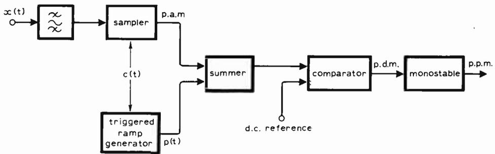
Fig. 7 (top). A pulse-position modulator.
