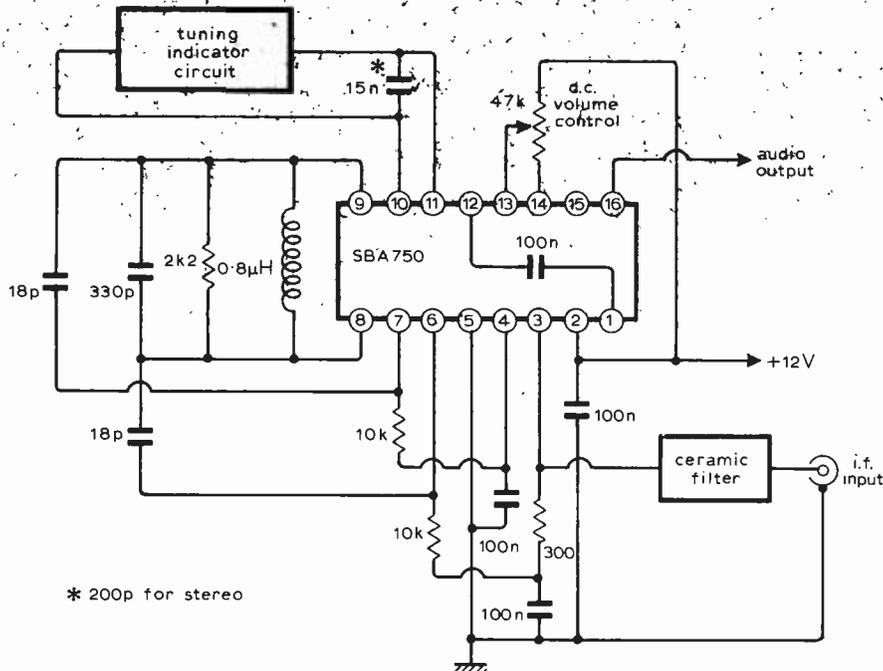
Fig. 4. Used with the SBA750 i.c., the reference can be dispensed with as the output is differential.
