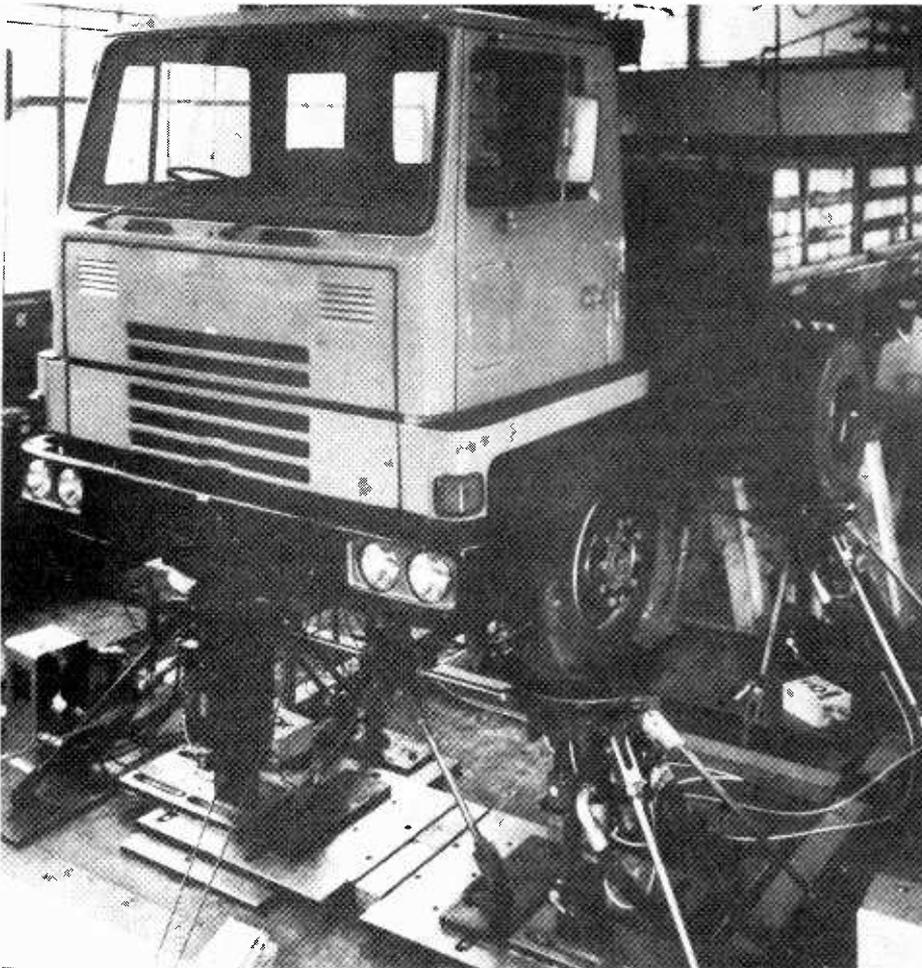
Prototype of the new Bedford heavy-truck range undergoing ride and vibration tests on the "road simulator" at the National Engineering Laboratory, Scotland. A computer is used to pin-point peak areas of vibration within the truck.
