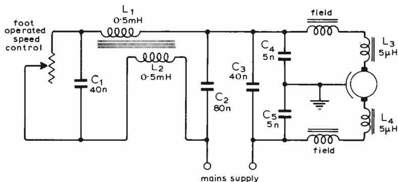
Fig. 3. Typical circuit for suppression of a sewing machine.
