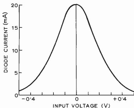
Fig. 5. Lamp current versus input voltage relative to reference voltage.
