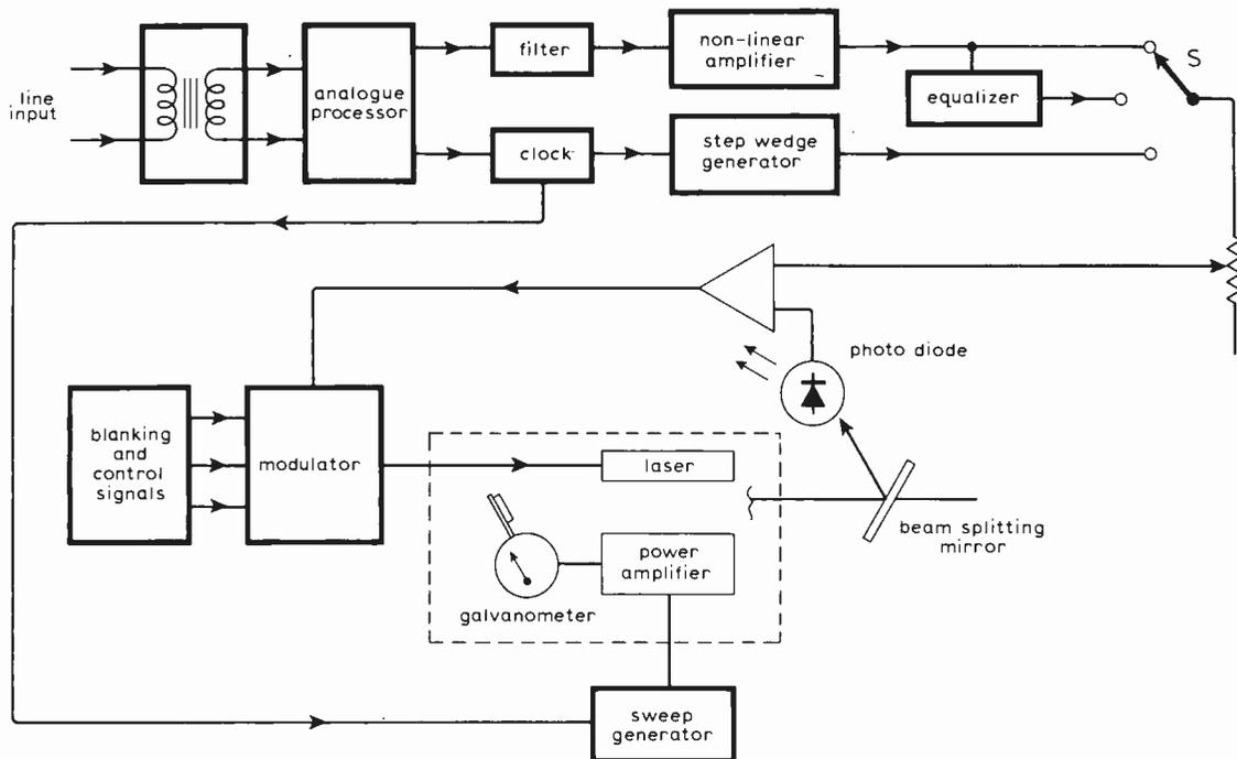
Fig. 2. Block diagram of the wirephoto receiver.
