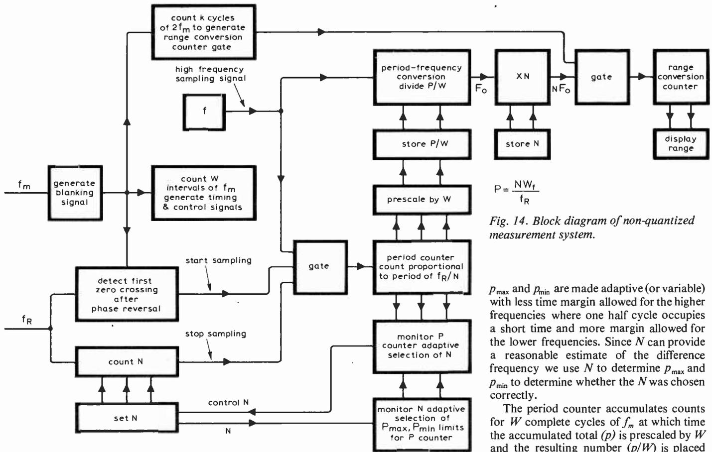
Fig. 14. Block diagram of non-quantized measurement system.
