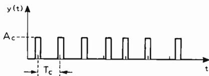
Fig. 6. Pulse-position modulation.
