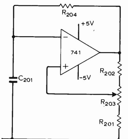
The problem can be minimized by a simple rearrangement of components as shown in the diagram. Any change in contact resistance is to be compared with the input resistance of the 741, not  $R_{204}$ . Since the input resistance of a 741 is typically  $1M\Omega$  an increase in stability greater than an order of magnitude can be expected.
