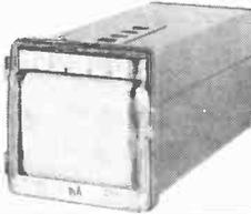
Provides permanent record of DC currents up to 1mA. Eminently suitable for use where space is limited. Separate time marker pen provided. Chart width 80mm. Chart length 40ft. Chart speeds: Slow 20-60-180 mm/hour. Fast 600-1800-5400 mm/hour. Dimensions 120x120x285mm. Weight 7.7 lbs. (3.5 Kg). Price complete with accessories
