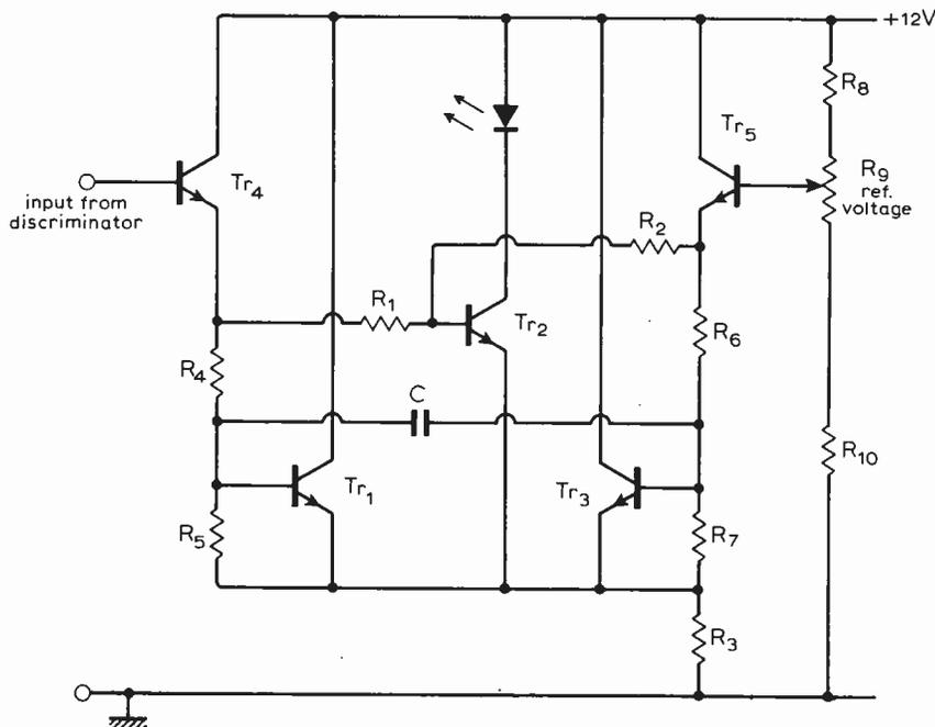
Fig. 3. Additional components reduce current drain of  $Tr_1$  and  $Tr_3$  by an order of magnitude and increase input impedance. (Transistors are integrated.)
