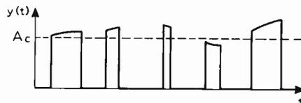
Fig. 9. Combined amplitude and width modulation for two information channels.
