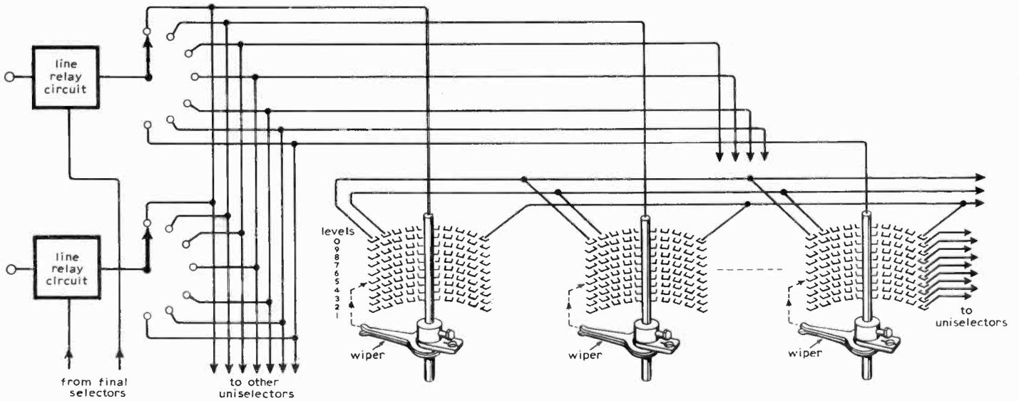
Fig. 7 Simplified diagram of a 100-line exchange.
