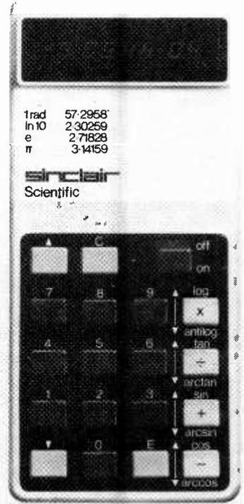
The Sinclair Scientific calculator. The four function keys each fulfil a dual function, selected by the keys at top left and bottom left.
