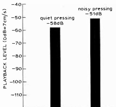
Comparison of surface noise on quiet and noisy vinyl pressings (RIAA playback, "A" weighted scale, unmodulated groove).
