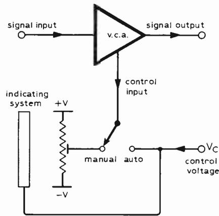
Simplified voltage controlled amplifier fader.
