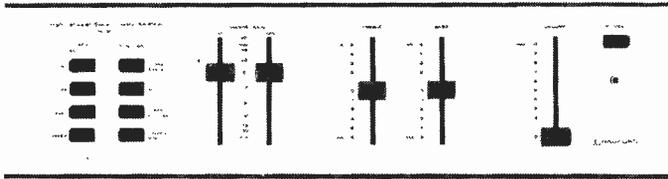
Designed for disc and tuner input and two tape machines, with complete recording and reproducing facilities.
