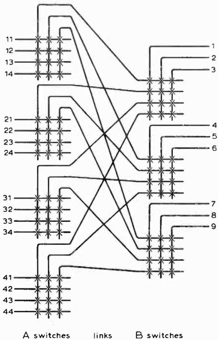
Fig. 9 Use of small co-ordinate arrays of switches to make larger switches.
