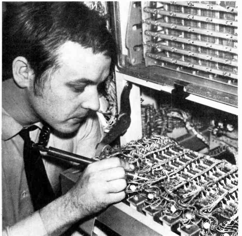
Fig. 8 Working on a cross-bar switch (GEC Telecommunications Ltd.).
