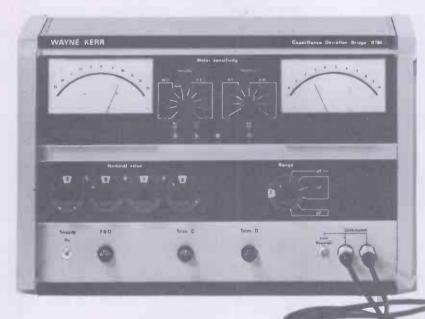
The B700 provides all the facilities required for checking capacitors during manufacture, quality control and batch selection to an accuracy of 0.1%. It can be adapted to control sorting, winding or cutting machines and is the latest in the WAYNE KERR series of transformer ratio-arm bridges.
