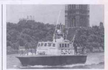
Prototype 52 ft. self-righting Lifeboat demonstrated recently on the Thames, with twin Bantex Aerials.
