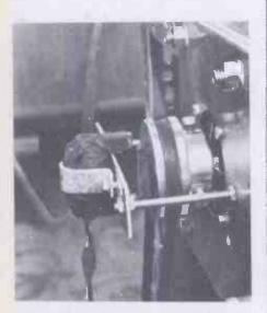
Synchronizing magnet and pick-up coil.
