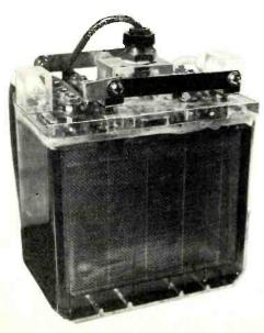
The top manifold, through which the hydrogen and oxygen gases are fed in, distinguishes the fuel cell from the otherwise conventional "battery" appearance.
