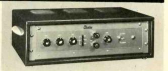
Integrated Mixer/Amplifiers Models A25–30 watts, and A80–60 watts, having inputs for two Microphone Channels balanced at 30 ohm, Auxiliary inputs for Microphone, Gramophone and Tape, each channel independently controlled. Overall Master Gain Control. Treble and Bass tone controls giving ± 12db lift and cut.
