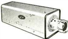
Totally enclosed dustproof unit only  $3\frac{3}{4} \times 4 \times 10\frac{1}{2}$  in., weighing 4 lb. Finished in two-tone blue/grey. Vidicon tube. Automatic sensitivity control enables the camera to maintain full picture quality over a brightness range of 60: 1. 625 line scanning standard 2: 1 interlaced, frame synchronised to mains supply. 600 lines horizontal picture definition with a bandwidth of 8 Mc/s. All supplies are obtained from the control monitor (consumption 5 watts).
