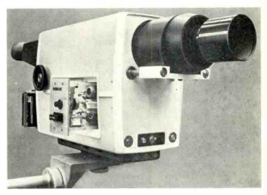
The high-speed camera showing the shuttering sine-wave oscillator module on the left.
