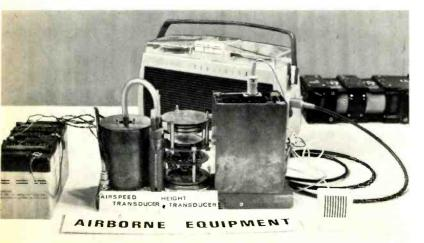
capacitor and thermistor. All the transducers were adjusted to a frequency range of 4-10kHz to suit the recorder. Although the calibration curves of these transducers are not quite linear, it was said that this could easily be corrected by the computer.
