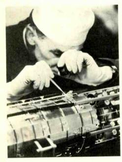
This month's cover. In clinically clean conditions at S.T.C's North Woolwich factory a submarine repeater undergoes one of many rigorous inspections. These repeaters, now being laid on the new £22 million Lisbon-Cape Town project, are required to go on working faultlessly for periods exceeding 20 years and so have to be manufactured to ultra-high standards. Undersea cable and repeaters are now an important British export—S.T.C. has about 50% of the current world market.
