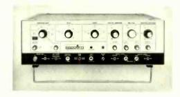
trigger output is supplied for all modes of operation. Pulse delay is variable from 15 ns advance to 50 ms delay, pulse width is variable from 10 ns to 5ms. Repetition rate, delay and width jitter errors are less than 0.05%, while overshoot, undershoot, ringing and top slope aberrations are less than  $\pm 3\%$  at amplitudes of 300 mV and higher. Output stages cannot be damaged by any combination of panel-control settings, open or short circuits or back voltages of up to 10 V.
