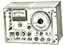
20 c/s to 20 Kc/s in a Single Sweep Logarithmic Scale Calibration. Accuracy ±1% ±1 c/s. Power supply 110 v. and 200-250 v. Dimensions: 19×12×13 ins. Supplied Brand New with Instruction Manual. Less than half Maker's Price. £125, ex Warehouse. Send 6d. Stamp for Data
