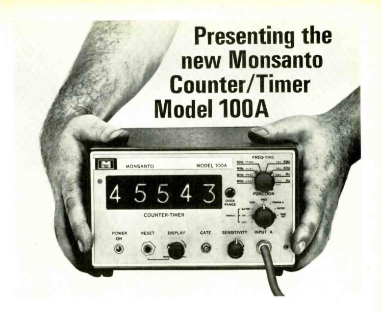
Integrated circuit construction plus completely original design concepts, result in high-quality 12.5 MHz counter/timer performance at remarkably low cost
