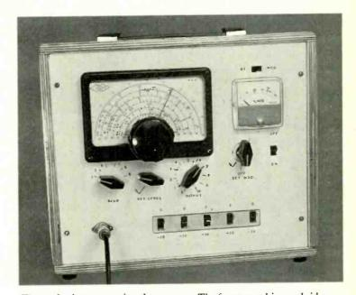
The author's protype signal generator. The front panel is overlaid with Perspex lettered on the reverse side.
