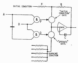
Fig. 5. Simplified schematic of electronic mode controlled integrator.
