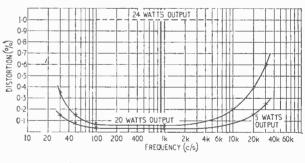
Below :—Fig. 8. Distortion characteristics of cascaded amplifier and preamplifier, 16  $\Omega$  resistive load.
