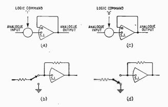
Fig. 3. Digital-analogue switch: (a) conducting state with (b) equivalent circuit; (c) non-conducting state with (d) equivalent circuit.
