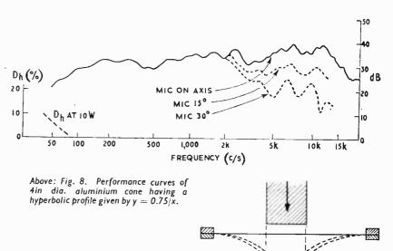
Right: Fig. 9. Showing the formation of a hyperbolic form by displacement at the centre of a stretched membrane.
