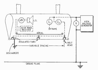
Fig. 7. Block diagram of test and measuring apparatus mounted inside simulated aircraft wing section.
