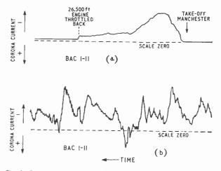
Fig. 1. Corona current measured during flights of BAC 1-II aircraft: (a) following take-off in clear air; (b) level flight in conditions of ice precipitation.
