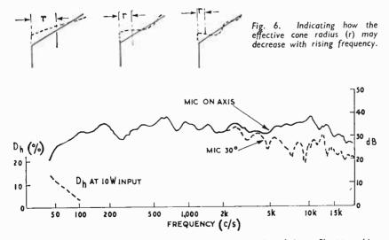
Fig. 7. Performance curves of 4 in dia. aluminium cone having a hyperbolic profile approaching a radius.
