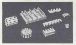
Refractories for high-temperature insulation.
