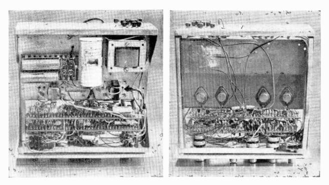
Top and underside views of the complete chassis. Note the heat sink for the output transistors.
