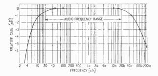
shown plotted in Fig. 8, where it is seen that full power output is obtainable up to over 40 kc/s. The distortion over the range of 20 c/s to 20 kc/s is very low compared with normal valve and transistor amplifiers which generally have rapidly rising distortion characteristics at the extremes of the audio range. Indeed quite a few amplifiers are unable to deliver full power output at 20 kc/s.
