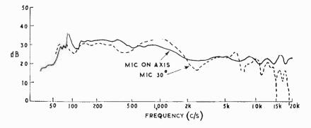
Fig. 5. Performance curves of full range electrostatic loudspeaker.
