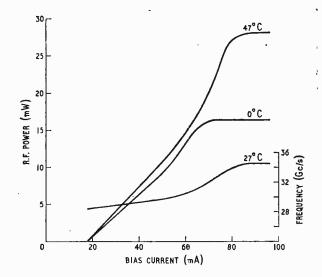
Fig. 2. Power output and frequency performance of a commercial GaAs avalanche diode at different bias currents. (Power measured at  $0^{\circ}C$  and  $47^{\circ}C$ ; frequency at  $27^{\circ}C$ .)
