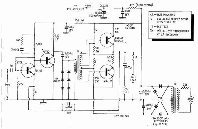
Fig. 1. Circuit of complete power amplifier.
