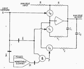
Fig. 7. Simplified schematic of track/store unit.
