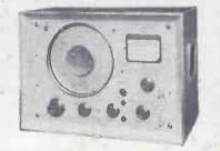
MF Transmission Measuring Set TF 2333 Signal Source 30 Hz to 560 kHz, Attenuator 70 dB in 1 dB steps, Level Meter -70 dBm to +25 dBm. Price: £335
