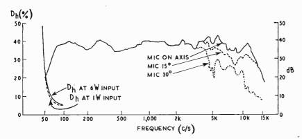
Fig. 3. Performance curves of 8 in hyperbolic paper cone m.c. loudspeaker.
