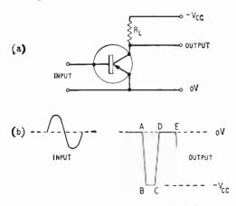
Fig. 65. Overdriven amplifier as amplified clipper.
