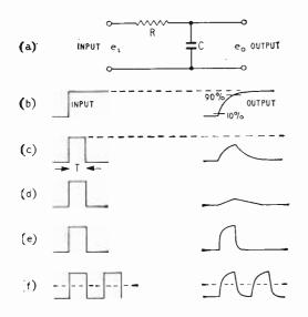
Fig. 59. Low-pass RC filter (integrator): (a) basic circuit, (b) step input, (c) pulse input (RC = T), (d) pulse input ( $RC \gg T$ ), (e) pulse input ( $RC \ll T$ ), (f) pulse train.
