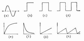
Fig. 56. Waveshapes commonly met with in pulse circuits: (a) sine wave, (b) step, (c) pulse, (d) square wave, (e) exponential, rising, (f) exponential, falling, (g) ramp. (h) sawtooth.
