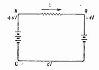
Fig. 4. Unlike the p.d. across a resistance, the p.d. across a source of e.m.f. does not reverse with direction of current.
