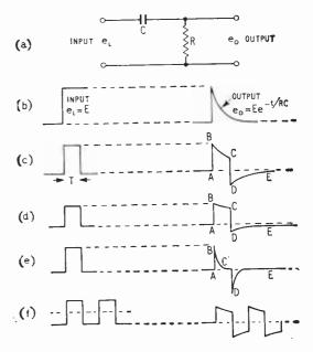
Fig. 57. High-pass RC filter (differentiator): (a) basic circuit, (b) step input, (c) single pulse ( $RC \Rightarrow T$ ), (d) single pulse ( $RC \gg T$ ), (e) single pulse ( $RC \ll T$ ), (f) pulse train.
