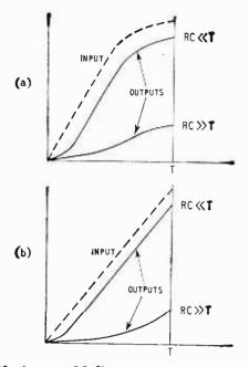
Fig. 60. Low-pass RC filter response to rising ramp; (a) panential, (b) linear.
