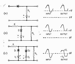
Fig. 63. Diode clippers (or limiters): (a) series, (b) parallel (shunt), (c) double parallel clipper (slicer).
