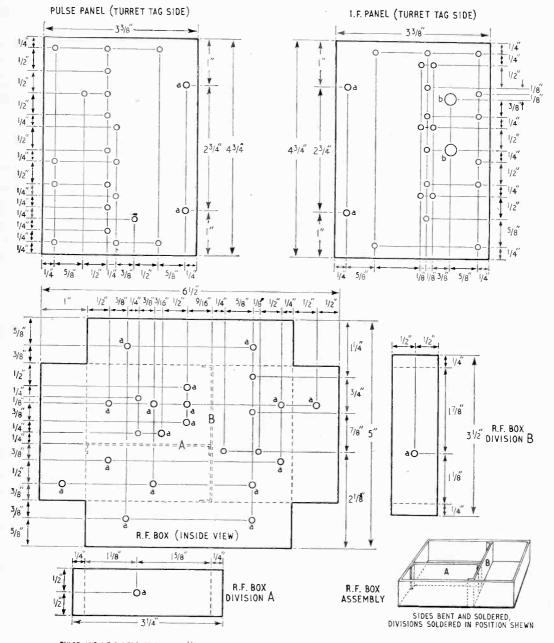
PULSE AND I.F. PANELS MADE FROM <sup>1</sup>/16in PAXOLIN R.F. BOX AND DIVISIONS MADE FROM THIN TINPLATE HOLES MARKED **a**, DRILLED <sup>1</sup>/8 in DIA, HOLES MARKED **b**, DRILLED <sup>1</sup>/4 in DIA, REMAINDER DRILLED <sup>3</sup>/32 in DIA.
