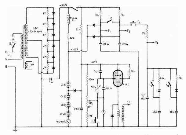
Fig. 4. Complete circuits of the power supply, trigger-pulse generator and stroboscope capacitor.  $VR_1$  is a pre-set control of trigger sensitivity and  $VR_2$  is a switched potential divider (200k $\Omega$  to 20M $\Omega$ ) for control of strobe rate. All semiconductor diodes are OY241.
