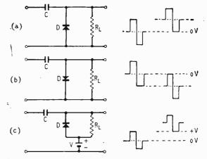
Fig. 64. Diode clampers (unbiased): (a) clamping -ve peak to OV, (b) clamping +ve peak to OV, (c) clamping -ve peak to +V.
