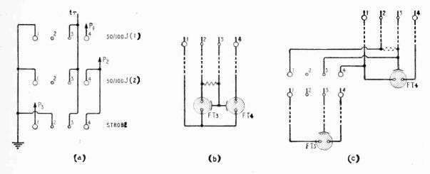
Fig. 5. Diagrams of the output and flash-head wiring. (a) The three UX4 output sockets. (b) A strobe-head consisting of two FA27 tubes on a single base. (c) Two separate heads, one of which bears an accessory UX4 socket for strobe use.
