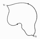
Fig. 2. Derivation of the fact that the net work done in taking any elecric charge around any closed path in any electric field is zero.
