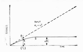
Fig. 58. Response of high-pass RC filter to rising ramp input.
