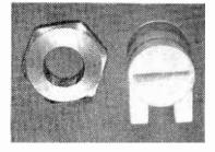
Steatite trimmer capacitors with 4 B.A. nut for size comparison.
