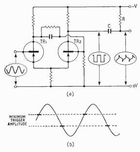
Fig. 4. Schmitt trigger circuit. At (b) is shown the reason for the minimum amplitude of input required.
