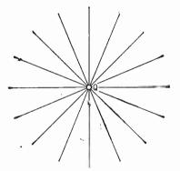
Fig. 1. Conventional representation of an electric field by lines of force takes this form around a concentrated charge in space.
