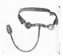
Amplivox throat microphone Type X.13761.
