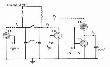
Fig. 1. Basic circuits for single, double or stroboscopic flashes. The points  $P_1$ ,  $P_2$  and  $P_3$  refer to the corresponding points in Figs. 4 and 5.
