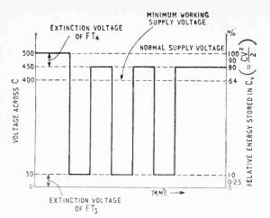
Fig. 2. Voltage and energy changes for the stroboscope capacitor C, initially charged to the full supply voltage and used for a sequence of six flashes. The extinction voltage has been exaggerated to 50 V for clarity.
