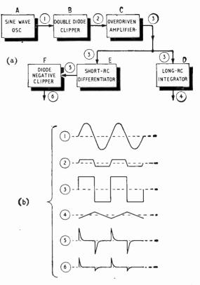
Fig. 66. Typical example of waveshaping of pulse train is cor. puter.
