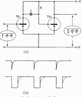
Fig. 5. Monostable flip-flop.
