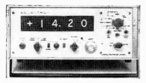
Right: Hewlett-Packard true r.m.s. voltmeter 3400A. Crest factors up to 100:1 can be tolerated.
