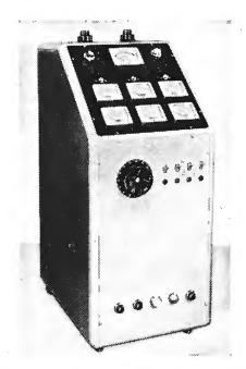
Control unit of G.V. Planer electron beam heating equipment for vacuum coating.
