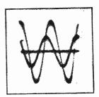
Fig. 4. Superimposition of two sine waves to show phase difference.
