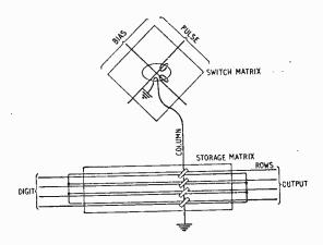
Fig. 7. Word address system with switch matrix.
