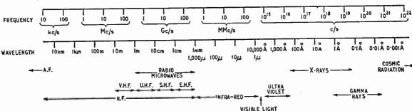
Fig. 1. Outline of a universal spectrum diagram showing the frequencies and wavelengths of the main varieties of electromagnetic radiation. The symbol " $\mu$ " stands for "micron", which is 0.001 mm; and " $\lambda$ " for "angstrom", which is 0.0001 $\mu$ .
