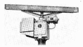
Aerial system of "Escort" radar. No parts other than turning gear and echo box are mounted with the aerial, so easing servicing problems.
