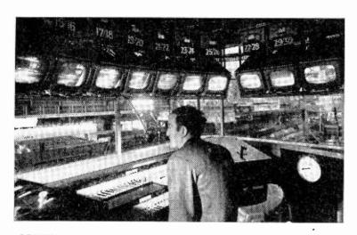
FIFTEEN closed-circuit television channels in the new rolling mill of the Steel Company of Wales at Port Talbot provide a composite view of about 700ft of railway track. This installation by Marconi's is for the remote observation of the conveyance of red-hot steel ingots from the soaking pits to the rolling mill.
