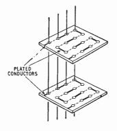
Fig. 8. Matrix store made up of perforated ferrite plates.
