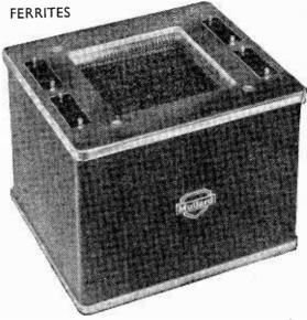
A stack of 20 matrix storage planes in practical form for use in a computer. The capacity is 81920 digits.
