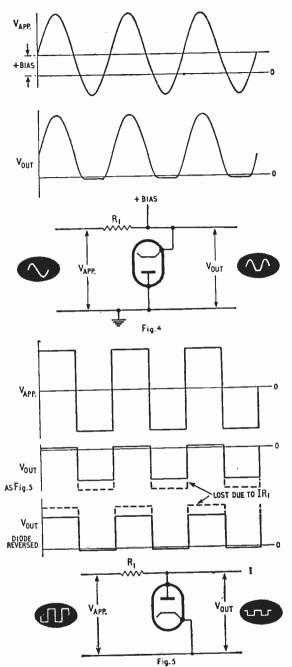
in limiting the CR coupling circuit time constant must be chosen so that no slide-back occurs.
