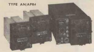
This Receiver is designed to determine the presence and measure the frequency of any radar or radio signals within the range of 38 to 2,000 Mc/s. To determine what modulation may be present on these signals giving an identification of relative strength of these signals.
