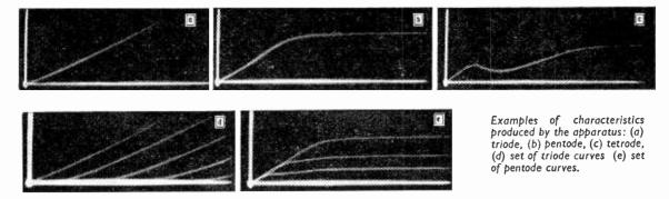
if the effect of supplying the screen grid with halfwave pulses is considered, since the resulting variation in screen-grid potential would follow that in anode potential and a triode characteristic would result.
