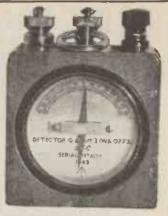
NEW GALVANOMETERS, solid brass, 3ln. dial, in polished wooden case. 70 degree scale, 35 mA either side. 100 ohm coil. Price: 12/6 each. P. & P. 1/6.
