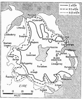
I.T.A. IN N. IRELAND.—Estimated service area of the new I.T.A. transmitter on Black Mountain, near Belfast. The station will radiate in channel 9 using horizontal polarization. The directional aerial atop the 700-ft mast, giving a height of nearly 1,700-ft above sea level, will have an e.r.p. varying from 20kW to 100kW. Full-power test transmissions are planned to begin in August.
