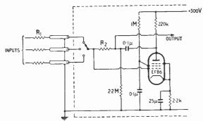
Improved input selector. The grid resistor of the following stage should be  $IM\Omega$ .
