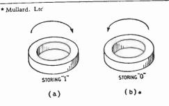
Fig. 1. Method of storing information by remanent magnetism in ferrite rings, (a) clockwise magnet zation and (b) anticlockwise magnetization.
