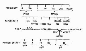
Fig. 2. Enlarged view of the part of Fig. 1 concerned with the infra-red band and its neighbours.
