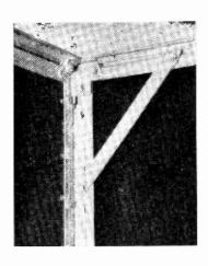
Left: View from inside of cabinet of new system. Note that it is necessary to drill holes in the front member only where they are required.
