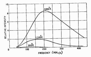
Fig. 3. Distribution of heat radiation as regards frequency, from a perfectly aperiodic radiator ("black body"), at three different temperatures.
