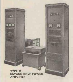
The SAVAGE 10KW AMPLIFIER is designed to meet the high power drive requirements of large vibrators. It has an output of 10 KW (continuous sine wave rating) over the frequency band 40 c/s. to 10 Kc/s. The output has eight secondary sections of 41½ V. each which may be cross connected to give a range of output voltages from 41½ V. to 330 V. Accessibility of components and ease of installation are features of this very compact 10 KW amplifier.
