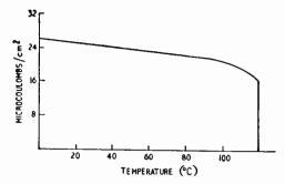
Fig. 3. Spontaneous polarization in a single domain of barium titanate, in microcoulombs per  $\rm cm^2$ .
