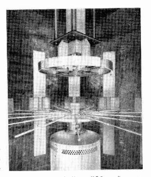
The aerial system of the Marconi V.O.R. installed in an aerial tower. Above is the omni-directional radiator with the figure-of-eight exciter below it.
