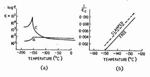
Fig. 4. Dielectric constants of potassium dihydrogen phosphate (divide e.s.u. by 900,000 to get  $\mu F \cdot cm^{-1}$ ). The c direction is the ferroelectric axis.
