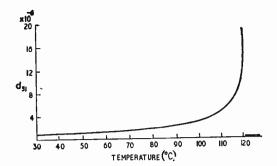
Fig. 5. One of the piezoelectric coefficients of a singledomain barium titanate crystal.
