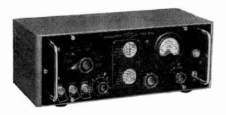
The Oscillator Type 858 is designed primarily for use as a calibrating Oscillator for the Wave Analyser Type 853, and as such provides fixed levels of output for setting up the instrument. It may however, be used separately as a c.w. oscillator of low harmonic distortion and stabilised output level.
