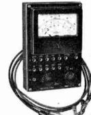
ranges a.c./d.c. 200 microamps — I,000 volts 5,000 ohms per volt
