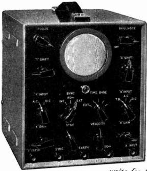
Model 1200B. For A.F. and low R.F. applications. Sensitivity 100mV/cm. B/W D.C. to 100Kc/s. C.R. Tube 3in. diam.
