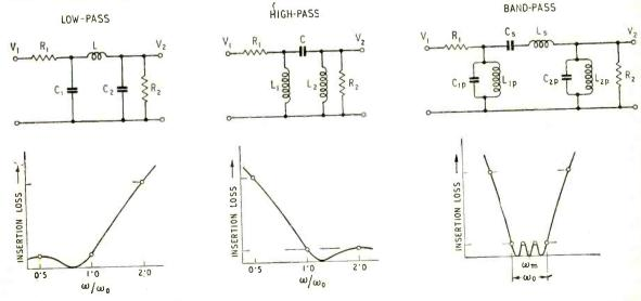
curve is used in the first case, the upper "db" curve in the second. When a value of t has been chosen the corresponding values of  $a_1$ ,  $a_2$  and  $a_3$  are read from their respective curves for the specified termination,  $R_2 = R_1$  or  $R_2 = \infty$ . The filter components are then calculated as follows: For a low-pass filter with cut off appulse for any second
