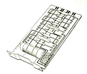
Fig. 3. Sub-unit using printed wiring and dip soldering, made from the master diagram of Fig. 2.
