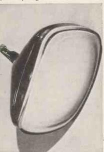
of the picture. Thirdly, in tubes with approximately flat faces, the deflected beam strikes the screen at increasingly acute angles, and the spot may be markedly defocused at the edges of the screen.
