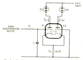
Fig. 1. Complete circuit diagram of neon tuning indicator. V3 and V4 are miniature uncapped neons (Hivac, type CCIIL). These are also available with M.E.S. cap and designated CCI0L.
