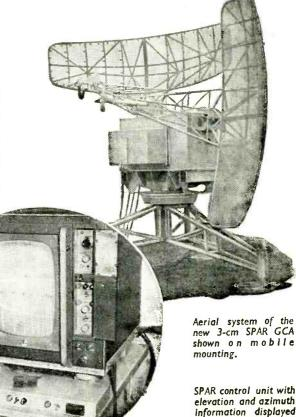
elevation and azimuth information displayed on a single extra-long persistence c.r. tube.
