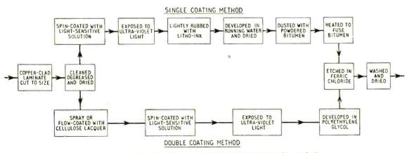
Fig. 4. Comparison of single- and double-coating photographic methods.
