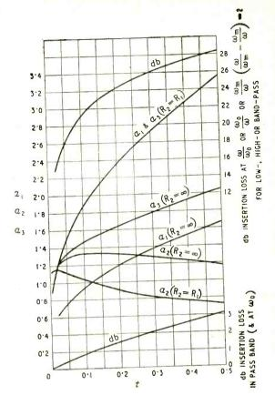
Fig. 1. Basic data for use in design formulæ.
