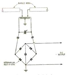
Fig. 2. Pick-up dipole head.
