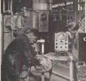
C The Cossor Model 1049 Double Beam Oscillograph displays the output of the twin inverters under test at the works of Sir W. G. Armstrong-Whitworth Aircraft Ltd. Photograph by courtesy of Sir W. G. Armstrong-Whitworth Aircraft Ltd.
