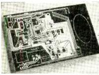
Printed circuit on De la Rue copper laminate.
