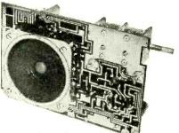
Four-valve portable embodying T.C.C. printed-circuit element.
