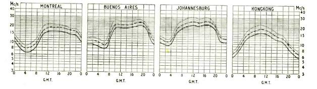
THE full-line curves given here indicate the highest frequencies likely to be usable at any time of the day or night for reliable communications over four long-distance paths from this country during September. Broken-line curves give the highest frequencies that
