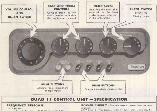
Cancel position. Radio & Tape inputs: 20-20,000 c/s within 0.3db. Microphone input: 20-18,000 c/s within 1db. Pickup Input (R.2): Within 0.5db of stated characteristics. Other plugs, no significant change. Bass and Treble controls: Within 1db of published curves. Filter frequencies (ff): SKc/s, TKc/s 10Kc/s ± 250 c/s. Filter slope: Level to 50 db/Octave.
