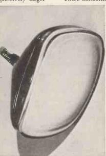
of the picture. Thirdly, in tubes with approximately flat faces, the deflected beam strikes the screen at increasingly acute angles, and the spot may be markedly defocused at the edges of the screen.
