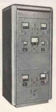
**Abbreviated Specification** Frequency range 60-216 mc/s Transmitter output Power 10 watts, or with Amplifier Unit-50 watts Maximum Deviation 50 kc/s **Overall Transmitter-Receiver Performance** Frequency Response 300 c/s-6 kc/s+3 db 6 kc/s - 36 kc/s + 1 dbIntermodulation Level At least-55 dbm for 2 tones applied each at 0 dbm Receiver Bandwidth 6 db down + 120 kc/s
