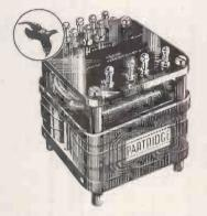
Optimum conditions are obtained in the form of output stage used in this amplifier when about 40% of the primary winding of the output transformer is common to anode and screen grid circuits. The Partridge Type P.3878 is of C-core design with tappings of 43% of primary turns, and is specified by the designer for this amplifier.
