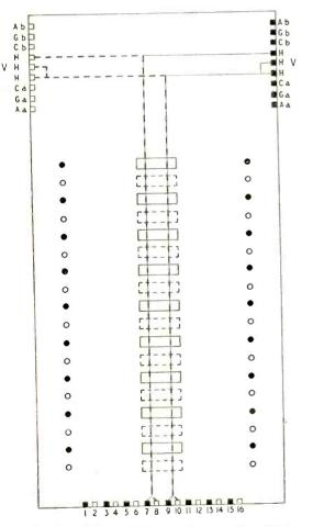
Fig. 1. Typical foundation pattern for use with white-onblack laminated paper for producing master circuits by engraving.
