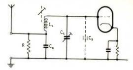
Fig. 5. Permeability-tuned aerial circuit.
