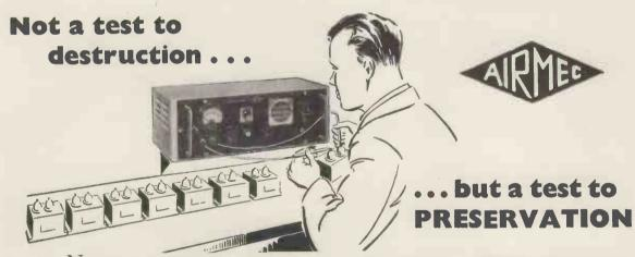
Normal testing of capacitors by the application of a voltage greatly in excess of their working voltage as a safety precaution is unnecessarily ruthless. Some components apparently withstanding the test may be damaged by it and subsequently fail in service, whilst others break down immediately under the increased stress, to which they would never be subjected in normal service, and are destroyed.
