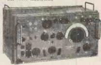
9 valves, R.F. amp. osc. Frequency Changer, 2 1.F.'s. (465 kc.), 2nd Detector, A.V.C. Af. amp. B.F.O. A.C. nains, 100-250 v. or 12 v. accum. Frequency range 17.5 to 7 Mc/s, 7.35 Mc/s to 2.9 Mc/s, 3.0 to 1.2 Mc/s. Monitor L.S. bulltin. Complete. Write for full details Price £12/12/-, plus 21/- carriage and packing.
