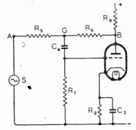
Fig. 1. The see-saw circuit in its - simplest form.
