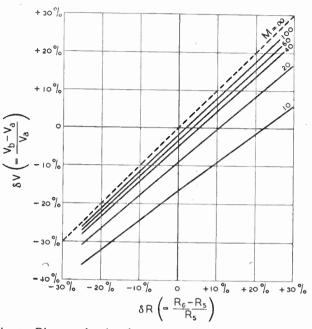
Fig. 5. Diagram showing the percentage departure from voltage balance ( $\delta V$ ) in terms of the percentage difference between  $R_{\delta}$  and  $R_{\delta}$  ( $\delta R$ ), for several values of amplification, M.
