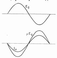
Fig. 1. Grid-voltage anode-current relationship.
