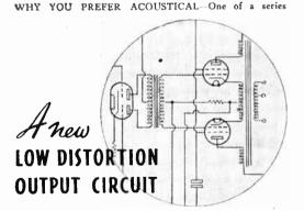
The new low distortion output circuit (an Acoustical Provisional Patent) incorporated in the M31 Amplifier provides a very high standard of reproduction-The output valves operate partly as triodes with cathode follower output and partly as tetrodes with negative feedback, thus giving considerable cancellation of generated harmonics and a high damping factor. Just one reason why you prefer Acoustical.
