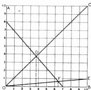
OE at F. Dropping vertically from F to OB we find that the reading is a little under 650 ohms—say 645. Work it out and you will find that the graphical solution is not so very far wrong.
