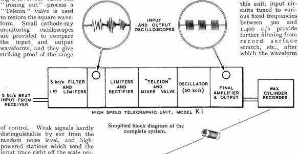
of control. Weak signals hardly distinguishable by ear from the random noise level, and highpowered stations which send the input trace right off the scale produce the same perfectly regular square-wave signal of constant amplitude on the output CR tube.
