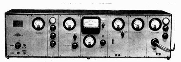
Romac Radio Corporation's Model K I High-speed Telegraphic Unit. At the head of the page is shown a specimen of receiver tape, and, below it, a section of the transmitter tape which actuates the electronic keying apparatus.
