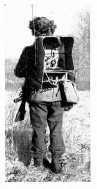
SUCCESSOR of the well-known infantry set No. 18. This shortrange transmitter-receiver, the 68P, operates in the 1.75 to 2.9 Mc/s band with crystal control for sending. It has facilities for 'phone and CW operation.
