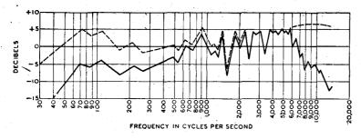
Fig. 1. The heavy line shows the response curve of the writer's loud speaker before correction, and the dotted line the approximate curve after correction. The decibel scale has been opened out to give a clearer effect of the result obtained.
