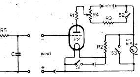
Fig. 3. Final circuit arrangement of the valve voltmeter described.
