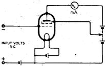
Fig. 1. Basic circuit diagram of a valve voltmeter of which the range of anode current proved too wide.
