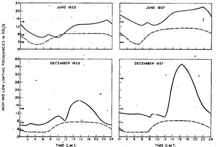
Fig. 3. High and low limiting frequencies for the summer and winter of years at the sunspot minimum and maximum for the transmission path to the U.S.A. by two hops of 3,500 km, each,
