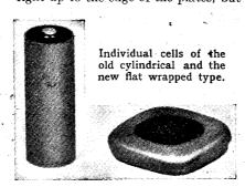
retains the electrolyte without additional sealing at the edges. Also, the resilient nature of the wrapping permits expansion due to chemical action during discharge, and the edge of each cell is chamfered slightly to allow just the excess volume required and no more.
