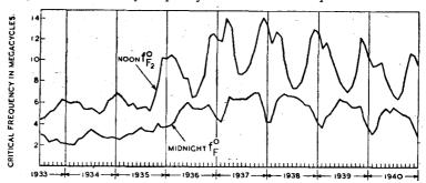
Fig. 2. Monthly average of noon  $(f_{F^0}^0)$  and midnight  $(f_F^0)$  critical frequencies at Washington.
