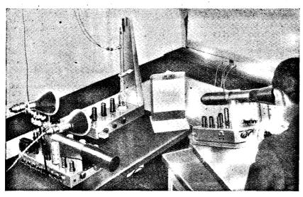
General view of a complete amateur television transmitting station: The operator on the right is viewing the test image on the combined iconoscope and monitoring tube. In the centre is seen the 2½ metre transmitter while on the left immediately below the two spot light lamps is the receiver.
