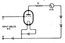
Fig. 2. Triode voltmeter with limiting resistance.
