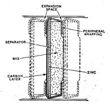
Inter-cell leakage is prevented and expansion permitted by the flexible wrapping of the latest flat-type dry
