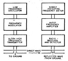
Circuit arrangement for altimeter.
