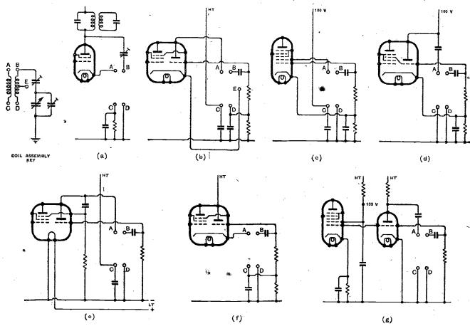
Fig. 1. Circuits employing the two-coil oscillator group. (a) autodyne; (b) triode-pentode; (c) heptode; (d) triode-hexode; (e) battery triode-pentode (note condenser coupling to pentode suppressor grid); (f) another mains-fed triode-pentode arrangement; (g) heptode with separate oscillator. Battery-fed single-valve mixers use similar coils, but battery autodyne and triode-pentode frequency-changers usually employ a third low-resistance dual winding carrying the filament current, as in Fig. 2.
