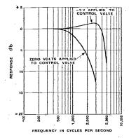
Fig. 4. Response of valve-controlled filter.
