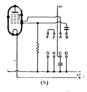
may be of service if the experimenter is lucky enough to have a choice of replacement valves: (a) The "autodyne" (Fig. 1) is now little used because it is not so easy to maintain oscillation at the higher frequencies, and because a good deal of the oscillator output is conveyed to the signal circuits through valve capacities. It works best at broadcast frequencies. (b) The triode-pentode, which is really
