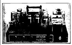
A pair of matches GLd's with 1-1 per cent, negative feed-back is fitted in the output stage, and the separate HT supplies to the anode and screen have better than 4 per cent, regulation, while a separate rectifier provides bias.
