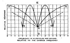
Fig. 7. Showing cancellation of frequencies near the carrier frequency for large and small assumed differences in path length. Difference of 75 kilometres gives BCB; 18.75 km. gives ACA.
