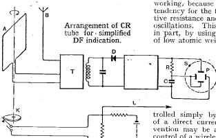
The output from the latter is then rectified at D and applied, through a phase-splitting circuit R, C, to the deflecting plates of a cathode-ray tube P. In the ordinary way, this would cause the electron beam to trace out the circular path shown in dotted lines on the fluorescent screen, the trace being continuously visible.
