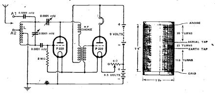
Fig. 2. Complete circuit diagram of the lightweight receiver discussed in the text. Inset is shown winding details of the tuning coil (inductance approximately 800  $\mu$ H). The wire is No. 36 SWG, enamel covered.
