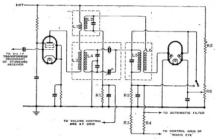
Fig. 1. Carrier boosting circuit. Values of components: L1, small 8-turn coupling coil; L2, 90 µH, shunted by 1350 µµF; L3, L4, L5, L6, 860 µH; R1, 0.2 megohm; R2, 0.5 megohm; R3, R4, 2 megohms; R5, 50,000 ohms; R6, 10,000 ohms.
