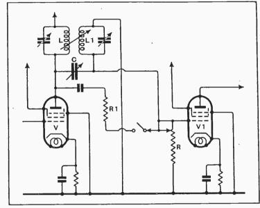
Circuit arrangement for control of selectivity in IF amplifier.
