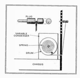
Operation of the Gody tuning system. Note the cord round the condenser drum, which is rotated against the tension of a return spring.
