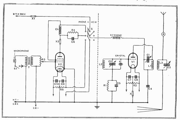
Fig. 1.—Circuit diagram for the transmitter, showing change-over switching for morse or 'phone. With centretap keying as shown (key at X), separate LT windings are necessary for V1 and V2. With certain valves, conditions may arise where it is better to connect the screen of V2 to the anode side of the choke.
