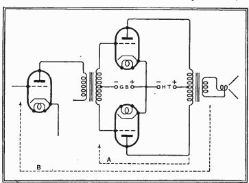
Fig. 1.—Negative feed-back may be applied across the output valves only, as indicated diagrammatically by A. But by extending its scope in both directions, as shown by B, its benefits are applied to the whole amplifier, provided that proper precautions are taken.
