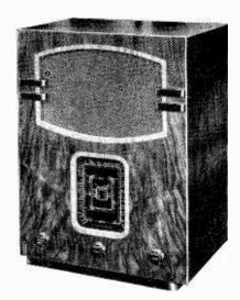
McMICHAEL MODEL 371. Coloured light bands are used as tuning pointers for the three wavebands in this new 10½ guinea McMichael AC superhet. The slow motion drive incorporates a flywheel for quick tuning, and the station names are printed in colour on a black background. Three valves and a rectifier are employed in the circuit of the set, which is available also as an AC/DC model at 11 gns.
