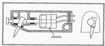
Diagrammatic section and end view of Shure pick-up showing tilt of needle in two planes.
