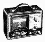
Simpson multi-range Roto-Ranger measuring instrument.
