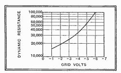
Fig. 1.-Specimen calibration curve: AC/SG valve with 90V on anode and 30V on screen.
