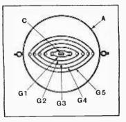
Electrode assembly for a frequency-changing valve.
