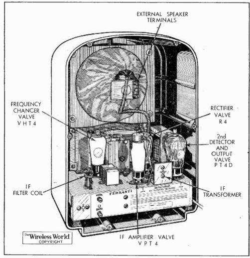
By careful disposition of the components above and below the chassis it has been found possible to dispense with screening cans for all coils, with a consequent increase in efficiency.
