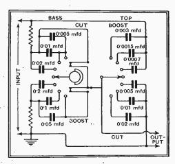
Fig. 3.—A composite circuit providing control of both bass and treble.
