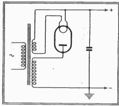
Fig. 34.—The same half-wave rectifier with negative HT earthed. This increases the voltage between the transformer windings.
