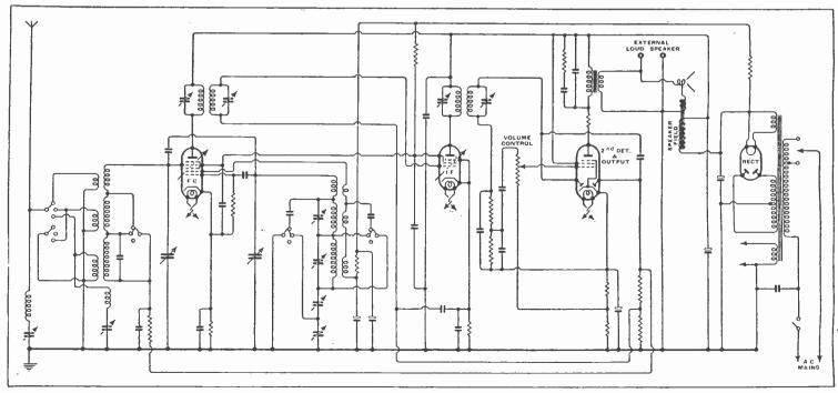
Although the superheterodyne circuit makes use of only three valves it has a remarkably efficient performance, particularly on long waves.
