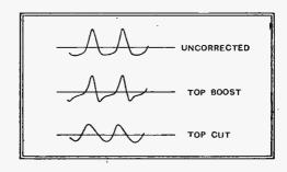
Fig. 7.—Effect of over-biasing one of the amplifier valves.
