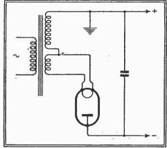
Fig. 33.—A simple half-wave rectifier circuit with the positive HT lead earthed.
