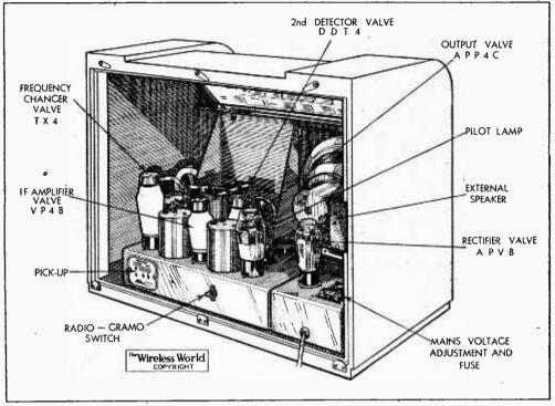
A single high-voltage pilot lamp mounted in the centre of the receiver chassis provides uniform illumination for the large rectangular tuning scale.
