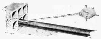
A socket wrench with a universal joint to reach normally inaccessible points has been produced by the Bell Telephone
