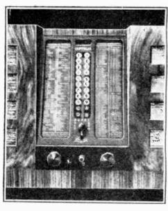
Keyboard and station index of the Elcosa automatic tuning system.
