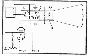
Combining electrostatic and magnetic control of the beam in a cathode-ray tube.
