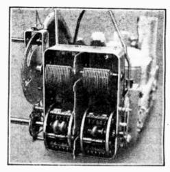
The Ondia tuning unit comprises a switchcoil "ensemble."
