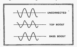
Fig. 6.—Top boost makes evident the harmonic content of the uncorrected waveform; bass boost has the opposite effect.
