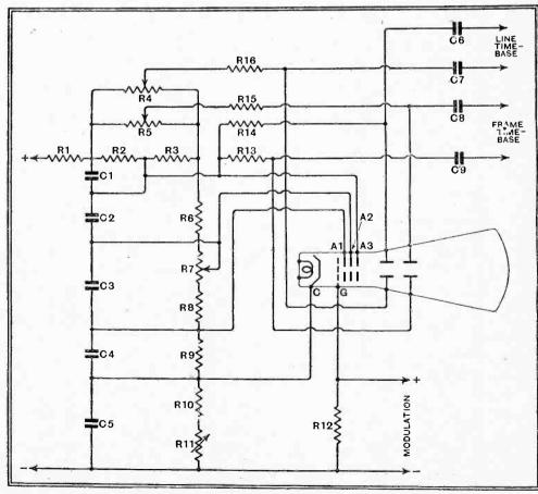
Fig. 36.—The smoothing equipment for the high-voltage supply and the potential divider for obtaining the various anode voltages are shown here.
