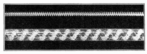
A length of the flexible Styroflex insulating material, and (below) method of winding it round a conductor in such a way as to provide insulation consisting mainly of air.
