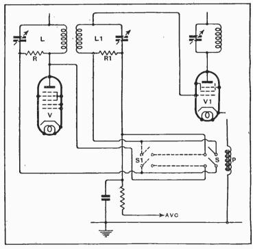
IF amplifier circuit for automatic and manual control of selectivity.
