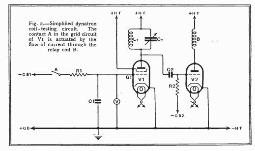
detected in a nearby oscillating receiver), then from the value of this critical bias voltage the value of the RF resistance may be found directly from the curve, oscillations ceasing when the negative resistance becomes equal to the dynamic resistance of the tuned circuit.
