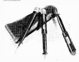
Forbat Pressler neon test prods.
