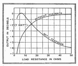
Fig. 6.—The effect of negative feed-back on the output/load resistance characteristic of the amplifier described. These curves do not take account of distortion, which is excluded by running well within the rated output.
