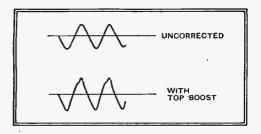
Fig. 5. — How top boost accentuates the harmonic distortion of the uncorrected waveform
