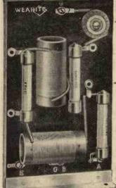
The complete Wearite Aerial Filter Panel. Ready for mounting in your "Single-Span Four."
