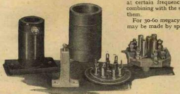
This group includes the Kinva and Goltone short-wave HF chokes, Bulgin 5-pin valveholder on steatite base and standinsulator, also lystone 7 - pin Eddystone 7 - pin chassis valveholder on base of new DL-9 insulating material.
