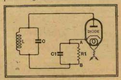
Fig. 1.—The fundamental diode detector circuit.
