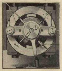
Enlarged view of pivot of milliammeter. The coil can be seen here; it moves at right-angles to the pointer. Note balancing weight on the latter.
