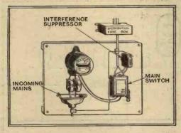
Fitting a Belling-Lee interference suppressor to incoming mains.
