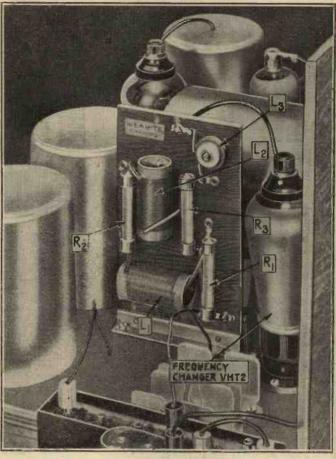
The position of the aerial filter in relation to the components is clear from this photograph.
