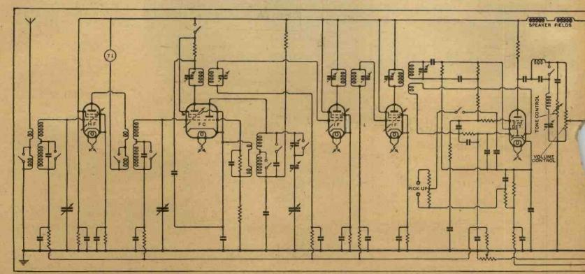
A signal-frequency amplifier and two IF stages provide a high degree of range and selectivity. The coupling of the IF circuits is adjustable, as is the
