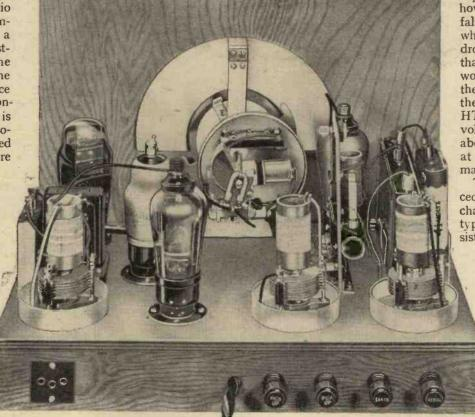
basic winding is the tuned secondary. Since the IF valve is of fairly high AC resistance a I-I ratio between primary and secondary gives the best amplification and is satisfactory from the selectivity viewpoint. A I-I ratio between the secondary
