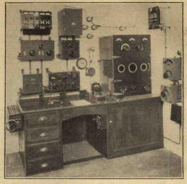
A standard 1.5-kilowatt Marconi installation for passenger ships.
