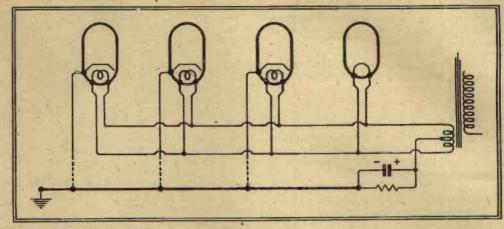
Fig. 4.—Automatic grid bias for a directly heated valve can be provided without needing a separate LT winding.
