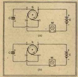
Fig. 21.—Condenser and battery, with rotating reversing switch. The behaviour of this circuit leads directly to the properties of capacity in an AC circuit.
