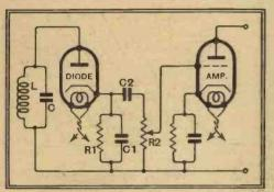
Fig. 4.—The usual coupling between a diode and an LF valve.
