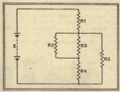
RI=100 ohms, R2=200 ohms, R3=500 ohms, R4=150 ohms, R5=1000 ohms, E=40 volts.
