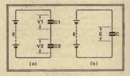
Fig. 13.—Condensers in Series. The voltage E is divided between the condensers; hence each takes less charging-current than if it were directly connected across E. For the same charging-current in the two circuits,  $\tau/C = \tau/C\tau + \tau/C2$ .
