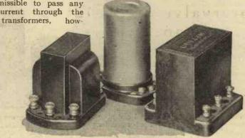
The Multitone Tone Control transformer is shown on the left, with the Benjamin Transfeeda in the centre and the Bulgin Transcoupler on the right.
