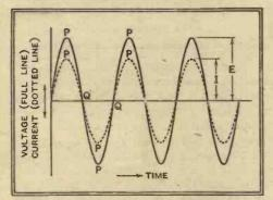
Fig. 20.—Voltage and current relationships in the circuit of Fig. 22. The average power over one complete cycle is  $\frac{EI}{2}$ , or half the power developed when E and I both have maximum values.
