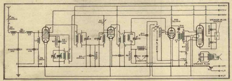
Fig. 1.—The complete circuit diagram of the new receiver shows that reaction is controlled by the variable resistance R7.
