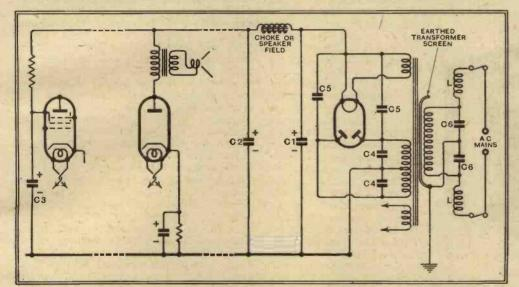
Fig. 2.—Circuit diagram of a typical power unit, showing positions of various condensers that may be used.
