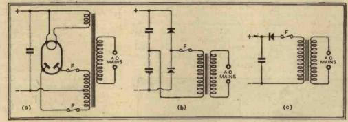
r.—F indicates fuse positions for protecting the H.T. circuit with (a) a full-wave valve rectifier, (b) a voltage-doubling metal rectifier, and (c) a half-wave rectifier of either sort.
