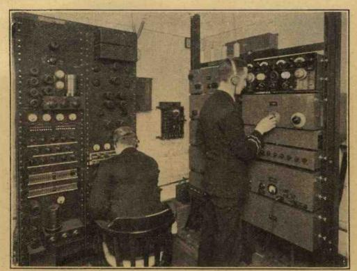
A Marccni short-wave wireless telephone receiver in operation on the "Empress of Britain."
