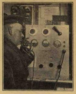
Trawlers are now fitted with fool-proof radio telephony sets. Here is a Siemens Co.'s installation in use.
