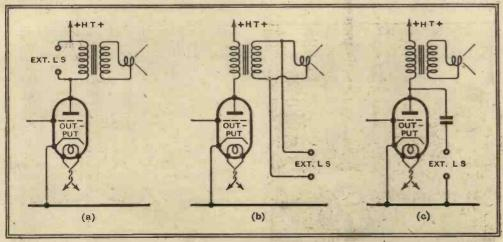
Various methods adopted by the leading set manufacturers for providing suitable terminals for extension loud speakers.
