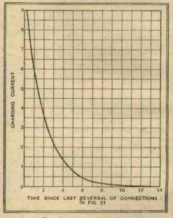
Fig. 22.—Showing the rapidity of the decay of the current after each reversal of direction.
