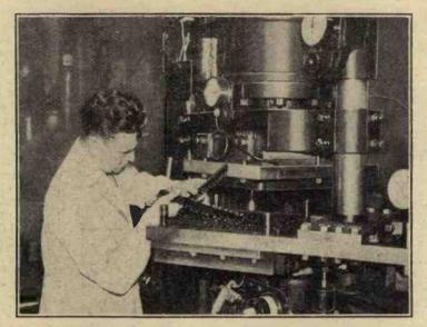
FIXED CONDENSERS BY THE BUNCH. A scene in the H.M.V. factory, Hayes, showing the 80-ton press which turns out 90 fixed condensers simultaneously.
