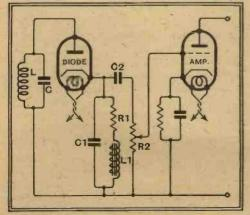
Fig. 5.-A modified coupling for distortionless detection. Lr has an inductance of 300 H.
