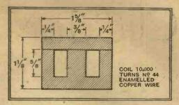
Fig. 7.—A suitable core for the 300 H. choke can be built from 25 pairs of varnished Laminic stampings, 0.015 in. thick.
