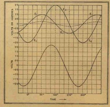
Fig. 30.—In the upper curve, Er represents voltage across the resistance, and Ec voltage across the condenser, of Fig. 29. The lower curve shows the resultant total voltage; that which the generator must have to drive 0.25 amp. through the circuit.
