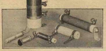
Types of wire-wound fixed resistances showing Bulgin mains, 40- and 10-watt; Dubilier 10-watt Spirohm; Watmel 3-watt and Amplion one-watt models.
