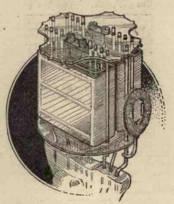
The QP21, a double pentode, which with proper precautions, can be used for the final stage as a class "B" output.
