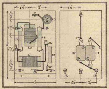
The construction and wiring of the aerial filter unit can clearly be seen in this drawing.
