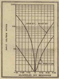
Fig. 4.—The selectivity, both with and without reaction, can be gauged from these curves.
