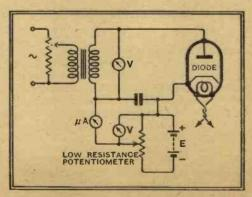
Fig. 2.—The circuit used for measuring the detector characteristics.
