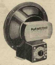
The principle of "impedence tuning" with a switched multi-ratio transformer is incorporated in the R. & A. "Multi-Mu" loud speaker.
