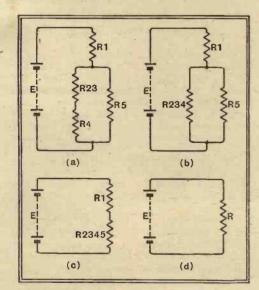
Fig. 11.—Successive stages in simplifying the circuit of Fig. 10. R23 stands for the single resistances equivalent to R2 and R3 R234 to that equivalent to R2, R3 and R4, and so on. R represents the whole system.
