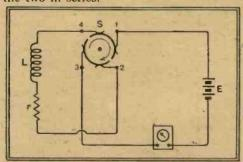
Fig. 24.—Inductance and resistance con-nected, through reversing switch, to a battery.
