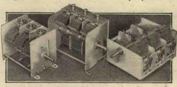
A group of three-gang condensers; the ones on the left and right are, respectively, Polar and J.B. straight condensers, while that in the centre is a Utility superheterodyne model.
