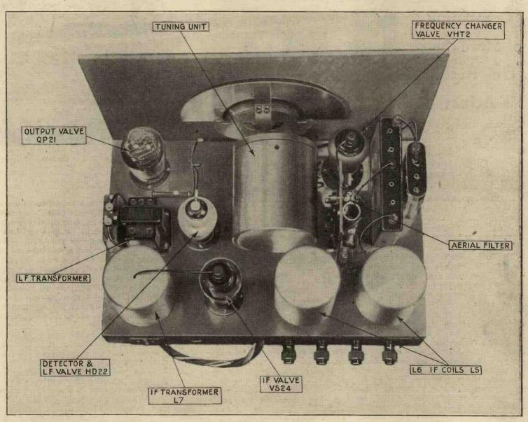
The positions of the chief components in the receiver can be clearly seen in this illustration.
