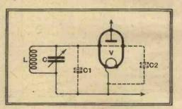
Fig. 3.—The total capacitance in a circuit comprises condenser C and small capacitances C1 and C2 representing wiring and grid/filament of valve.
