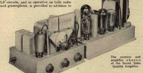
a control of the grid bias of the HF valve. These two volume controls, together with the waverange switch and tuning control, comprise all the panel controls. The apparatus is assembled on a grey finished metal chassis, and is so solidly constructed that it should give years of trouble-free operation.
