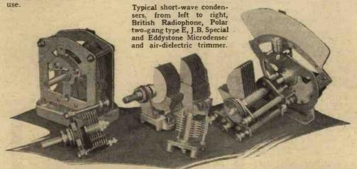
In a short-wave receiver the worst offender from the point of view of losses is the tuning condenser, which must have negligible resistance. Unless care is taken in the selection of this component, losses may be introduced, making it quite possible to obtain condensers which have a higher HF resistance than the coil associated with them. On this account it is obvious that air is the only suitable dielectric to use, tuning condensers with a bakelised-paper dielectric being entirely unsuitable.
