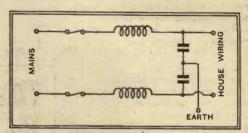
Fig. 2—Arrangement of a choke-condenser filter for suppressing mains - borne interference.
