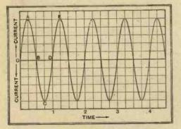
Fig. 18.—A curve showing the variation of the current in an oscillating circuit with time.
