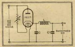
Fig. 1.—Usual connections of the rectifying valve in a universal receiver.
