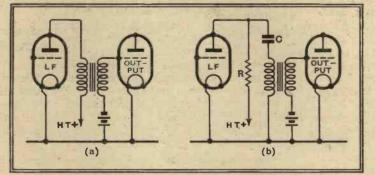
Fig. 1.—The direct coupling connections for an intervalve transformer are shown at (a) and the parallel-feed circuit at (b).
