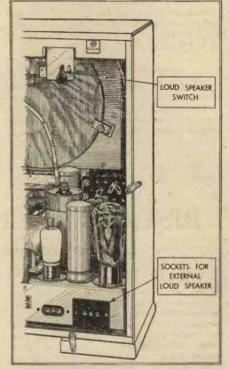
The addition of a switch to isolate the speaker on the set when the extension speaker only is required is provided on some of the Philips models.
