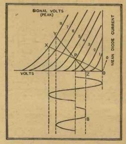
Fig. 3.—Typical diode curves are shown here with a DC load line XO and an AC load YZ of different values. The resulting distortion is shown at B.
