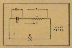
Fig. 29.—Condenser and resistance in series with an AC source. The generator-voltage E is equal to the total voltage due to the simultaneous presence of Ec and Er. See Fig. 30.
