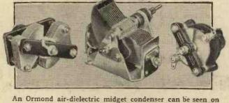
An Ormond air-dielectric midget condenser can be seen on the left, and a solid-dielectric differential reaction condenser of the same make on the right. In the centre is a Formo tuning condenser.
