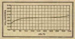
Fig. 5.—An appropriate barretter keeps the heater current for universal or DC valves at the correct value over a wide range of mains voltages.
