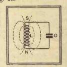
Fig. 17.—The discharge of C has driven a current through L, evoking a magnetic field opposite in polarity to that of Fig. 15.
