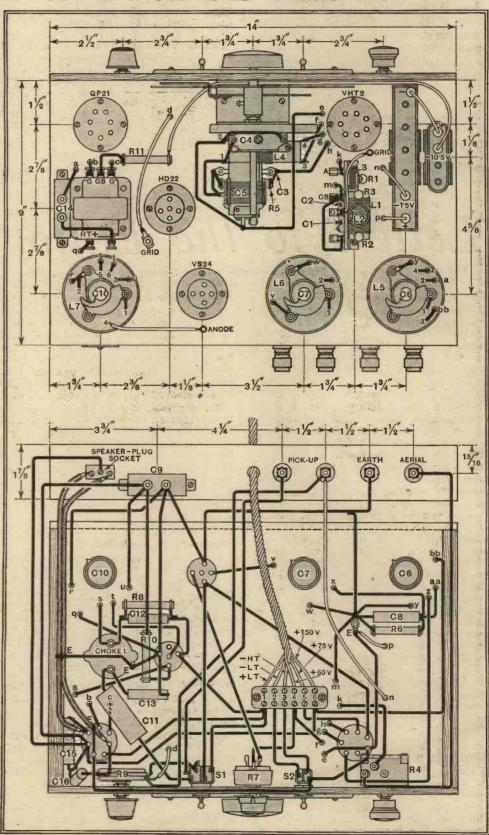
Full details of both the wiring and construction of the new receiver can be gleaned from the drawings.
