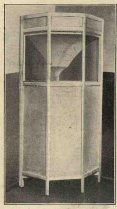
Designed to fit into a corner of the room, the latest Voigt domestic loud speaker retains the acoustic characteristics of its large-sized "straight" horn equivalent.
