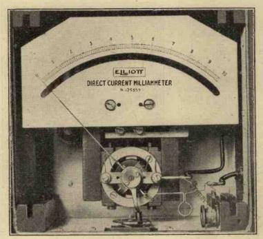
Milliammeter with front removed. The coil lies behind the pivot between the poles of the magnet. When moved by a current it sweeps the pointer over the scale.
