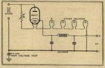
Fig. 2.—Wiring of the LT and HT supply circuits.
