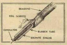
A method of providing air spacing (with consequent reduction in losses and self-capacity) for the conductor of screened aerial cable (Ward and Goldstone's "Metocel'').
