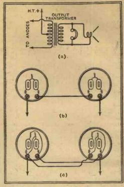
Fig. 2.—Connecting headphones to a QPP output stage, and (below) normal and suggested parallel connections of phone bobbins.
