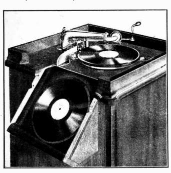
Produced at Hayes in 1920 and believed to be the first experimental automatic record changer. Five records could be handled.
