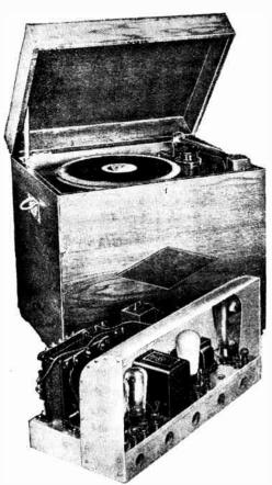
The amplifier shown separate from the The synchronous electric motor, pick-up and the two controls are attached to the motor board.
