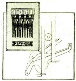
Zetavox automatic tuning mechanism, with tuning panel inset.
