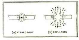
Fig 3.—(a) Attraction between dissimilar poles and (b) repulsion between similar poles.
