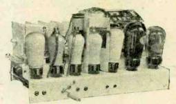
Columbia seven-valve A.C. superheterodyne chassis.
