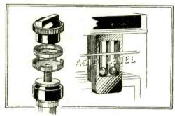
Terminal and charge-indicator of Fuller accumulator.
