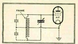
Fig. 2.—A centre-tapped frame, connected as Both ends now act as elevated aerials by their capacities to earth, but the resulting currents are in opposite directions and balance out.
