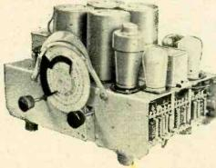
Philips 630A chassis showing micrometer dial.
