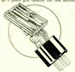
The record mutual conductance of 12.6 mA/volt is obtained in the Standard Micromesh PAI output valve. This illustration shows the cooling fins and the close-spaced electrodes.
