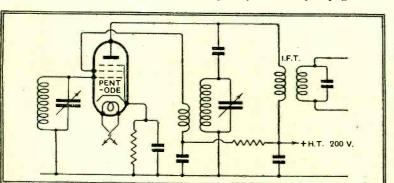
The final self-neutralised pentode frequency changer negligible circuit interaction, and is as efficient as a screen-grid type. The space-charge grid is operated with a very low positive potential.
