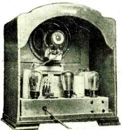
Yagerphone four-valve A.C. receiver.
