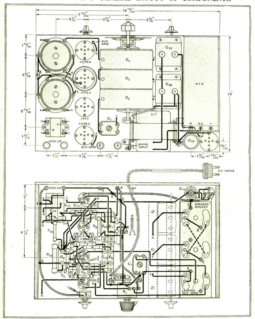
The clean layout ensures ease of wiring and the metal-covered baseboard assists in screening.
