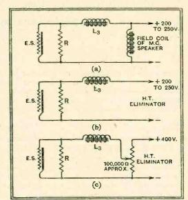
Fig. 3.—Various methods of obtaining the polarising voltage. The potentiometer in (c) should be adjusted so that the voltage applied to E.S. is about 220.
