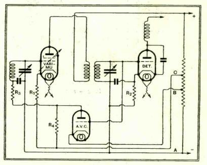
Fig. 1.—A popular American A.V.C. circuit in which an extra valve is used purely for control purposes.
