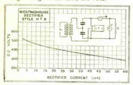
Fig. 1.—A basis for voltage calculations: output curve of a metal rectifier, showing the voltage corresponding to different loadings.
