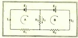
Fig. 3.—A more complex circuit the solution of which involves both the first and second laws. The circular arrows indicate directions taken as
