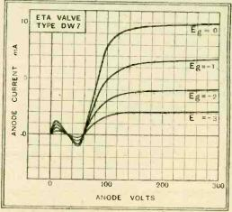
Anode current-anode voltage curves of "ETA"
