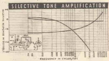
3/1 model. In radio apparatus which aims at the highest quality reproduction, it is desirable to control the response right up to a cut-off just below the heterodyne beat frequency between adjacent carriers. This aim, with the same principle of Tone Control, is realised in this model.
