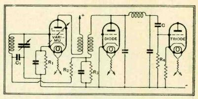
Fig. 2.—A circuit employing a diode for both detection and automatic volume control; an additional valve is usually needed as an amplifier to compensate for the low efficiency of the diode.
