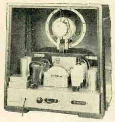
Chassis of the R.I. six-valve superheterodyne.
