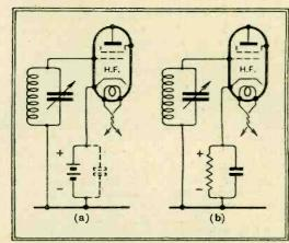
Fig. 2.—A bias battery, connected in the cathode lead, as shown in diagram (a), serves the same purpose as the usual bias resistance (diagram (b)).
