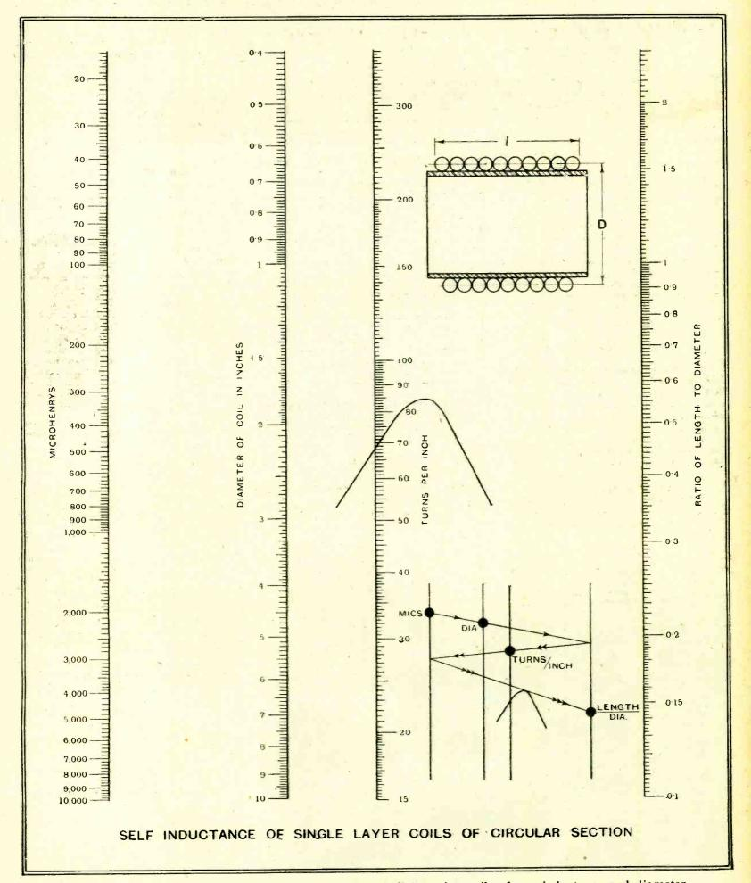
This time-saving abac gives the necessary data for winding tuning coils of any inductance and diameter having turns touching.
