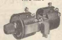
This component has been specially constructed in view of the tendency of modern design to reduce the number of controls. The Watmel Type M.S. 5 Dual Potentiometer is ganged with mains "on" and "off" switch, the one knob controlling mains switch, radio volume control and gramophone control. Price 13/6.
