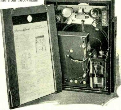
The back panel, which carries full operating instructions, is completely detachable, giving ready access to valves and batteries.
