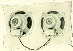
Magnavox dual compensated moving-coil units.
