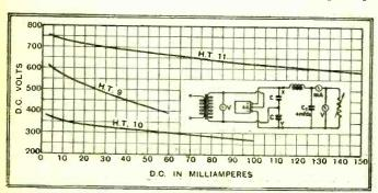
Regulation curves of new Westinghouse rectifiers, models H.T.9, H.T.10 and H.T.11, with constant input voltage and measured before smoothing.
