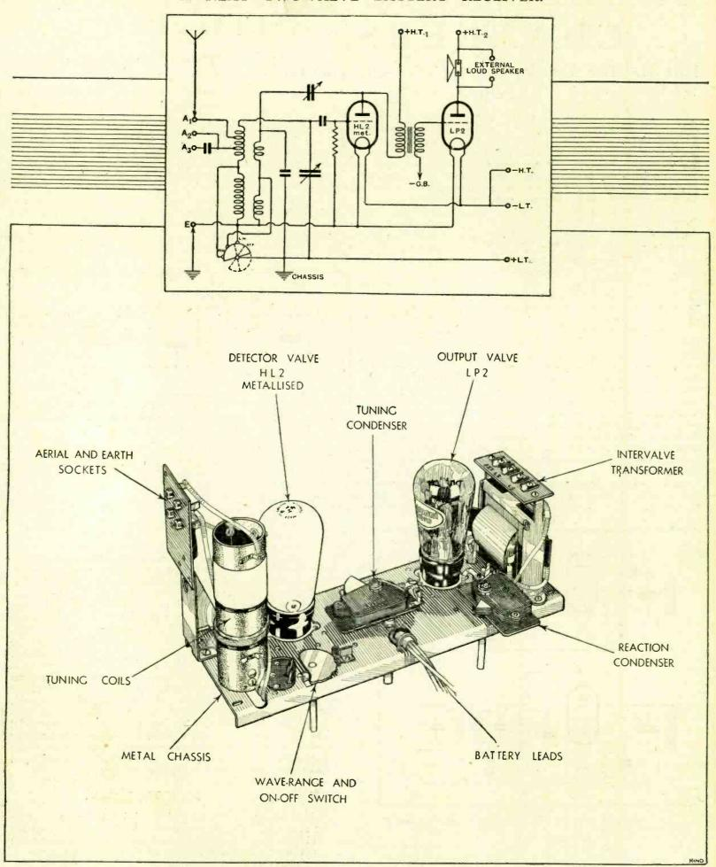
A high standard of workmanship and simplicity of design characterise the receiver chassis in the Marconiphone Type 248 set.
