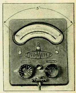
The scale length of a measuring instrument has an important bearing on the accuracy with which readings may be taken.
