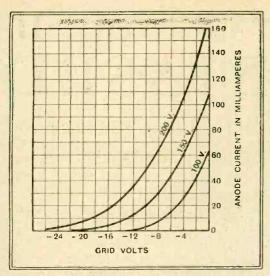
Anode current-grid voltage curves of "Micro-mesh" power valve, the PAI. power valve, the PAI.
