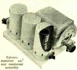
construction of a single-dial superhet.; the inductance on the two wavebands is 126.9 and 1,056 microhenrys when screened. The Link band-pass filter, with slight modification, is retained for the coming season. The properties of this component are now well known and provide a means of maintaining practically constant selectivity and sensitivity over the waveband by the judicious use of common capacity and negative mutual inductance coupling.
