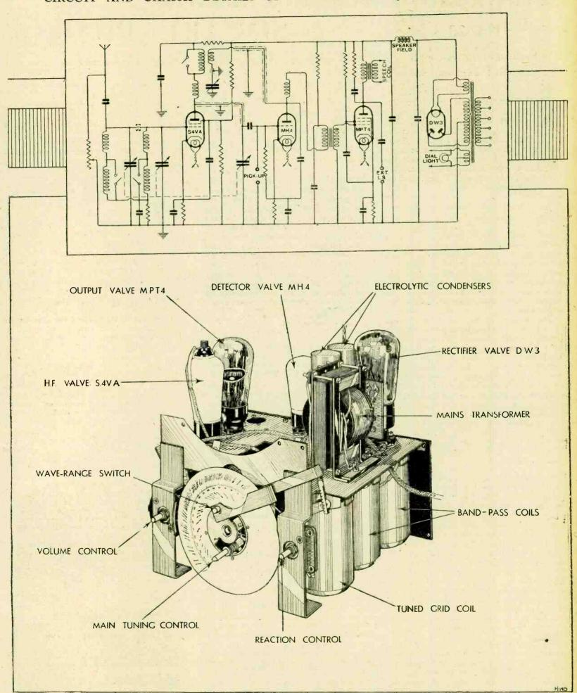
The complete receiver chassis, showing the principal components.
