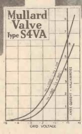
OPERATING DATA. Heater Voltage, 4-0 V; Heater Current, 1-0A; Max. Anode Voltage, 200V; Positive Screen Voltage, 110V. CHARACTERISTICS. (1) At Anode Volts 200; Screen Volts 110; Grid Volts zero.
