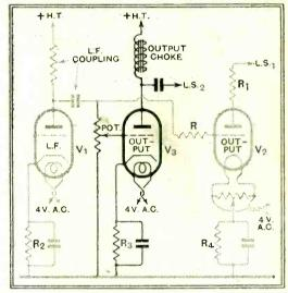
Fig. 2. - Connections of an extra output valve R<sub>2</sub>, R<sub>3</sub>, R<sub>4</sub>, bias resistors; V<sub>1</sub>, V<sub>2</sub>, original valves; V<sub>3</sub>, extra output valve.
