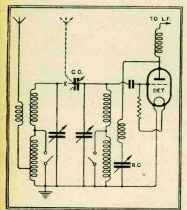
Stage-by-stage filter tests: the primary circuit is temporarily eliminated by interrupting the inter-circuit coupling at point X and transferring the aerial to the coupling condenser C.C.
