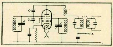
Fig. 6.—The bi-grid circuit re-drawn to show the valve capacities which account for the freedom from interaction.
