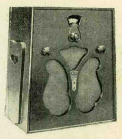
Self-contained three-valve battery receiver the Columbia Model 354.
