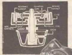
This new All-British resistance embodies many new and novel features which guarantee a higher degree of efficiency and a far steadier performance than resistances constructed on old and obsolete
