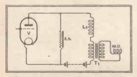
Fig. 1.—A suitable circuit where the transformation ratio of  $T_{\underline{i}}$  can be altered at will.
