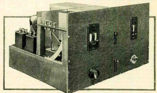
"The Wireless World" Band-pass Superheterodyne described in 1930. Terminals for the connection of a centre-tapped frame aerial can clearly be seen.
