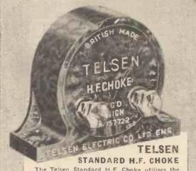
The Telsen Standard H.F. Choke utilises the minimum baseboard space. It is designed to cover the whole broadcast band, has very low self-capacity, and is highly suitable for reaction-circuits. The inductance is 150,000 microhenrys and the resistance 400 ohms. It has proved very popular and has been incorporated by set designers in many of the leading circuits.
