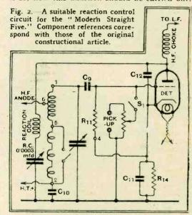
As this set has two H.F. stages, and a total of four tuned circuits, the additional complication of reaction should hardly be necessary, either as an aid to sensitivity or selectivity. Its use might, in exceptionally difficult receiving conditions, confer a slight benefit, but would tend to upset the overall frequency characteristics.
