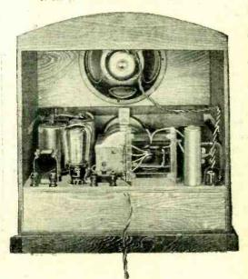
Rear view of the Baby Superhet. On the right can be seen the electrolytic condenser which greatly assists in smoothing.
