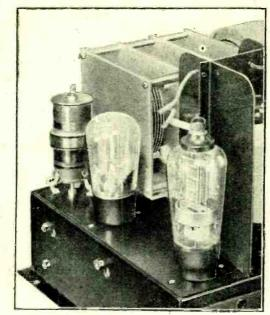
The essential components for the frequencychanging process in a typical modern superheterodyne.
