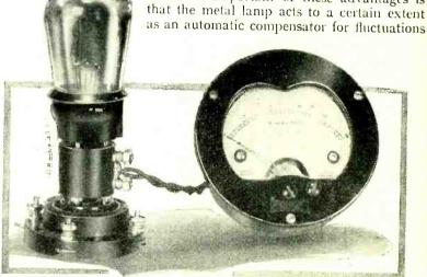
A convenient connection point for an anode milliameter: an adaptor interposed between a valve and its holder.
