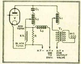
Fig. 5.—The complete schematic diagram. L<sub>1</sub>, I henry (tapped); L<sub>2</sub>, 0.2 henry (tapped); L<sub>3</sub>, 100 henrys; C<sub>1</sub>, I mfd.; R, 250,000 hms; T<sub>1</sub>, moving-coil output transformer; M.C. moving-coil loud speaker; E.S. "Primustatic" loud speaker; V, output valve. If the matching transformer T<sub>2</sub> of Fig. 4 is required, one winding replaces E.S. in the above diagram, and E.S., R and L<sub>3</sub> are connected to the other winding.
