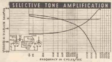
In radio sets and radiograms which aim at a definite 3.5/1 model. 5 kc. audio-frequency band, this model gives True Tone Control over a wide range.
