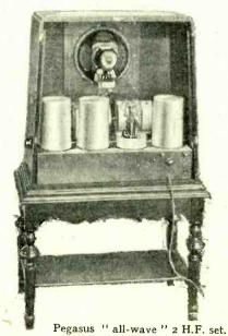
self-contained type, covers wave-ranges of 15-50, 200-600, and 750-2,000 metres, and embodies a Westinghouse rectifier and
