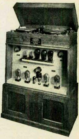
A 1-KILOWATT AMPLIFIER. The Tannoy battery - operated gramophone console and amplifying equipment installed in the "Daily Mirror" van now touring the health resorts.
