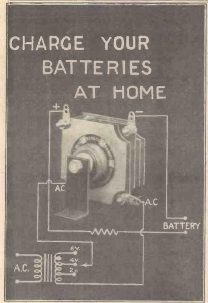
One of the greatest sources of inconvenience associated with wireless is undoubtedly the L.T. accumulator. Time after time a good programme is missed because the accumulator is discharged. BUT...now that the new L.T. Westinghouse Metal Rectifiers have been introduced, wireless enthusiasts with A.C. mains can always keep their accumulator "up to scratch" by trickle-charging it at home.
