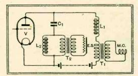
Fig. 4.—Where the impedance of E.S. is either too high or too low to act as an efficient load on the valve, the transformer T<sub>2</sub> is used to match the impedances at high frequencies.
