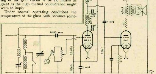
Fig. 1.—Suggested arrangement of detector and output stages using "Micromesh" HLA1 and PA1 valves
