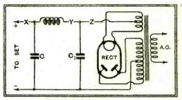
Fig. 2.—Testing for a partial short-circuit: positions in which a milliammeter may be connected.
