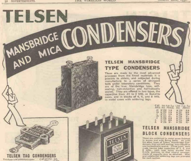
This type is of extremely compact and sturdy construction. It may be mounted on either insulated or metal panels by utilising the two baseboard screw holes in the neetly designed moulded casing. The tags enable the condenser to be connected to any other component, either directly or by soldering. H.F. losses are negligible. The capacity is stamped on the soldering tag.
