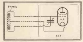
Fig. 4.—Correct connections. The connecting leads, as well as the frame, are now balanced, the tuning condenser being in the set. Short of taking laboratory precautions, this arrangement is the best possible for eliminating elevated aerial effect.
