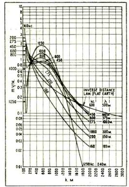
Fig. 5.—A series of international tests gives these mean peak values (m.v./M) of the down-coming ray at different distances from the transmitter. It will be seen that interference is not proportional to the distance (k.m.) that a receiver is located from the transmitter.
