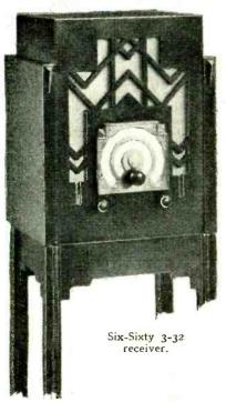
The volume control is unconventional and comprises a reaction condenser mechanically linked to a variable resistance connected between aerial and earth. The tuning dial is calibrated in stations, wavelengths, and kilocycles, and, instead of a pointer, a narrow beam of light indicates the resonance point.
