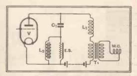
Fig. 2.—When the ratio of  $T_1$  cannot be altered, a resonant circuit  $L_2$  E.S. prevents the lower audio-frequencies from rattling the electrostatic loud speaker.
