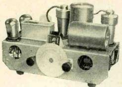
Philips 830A receiver chassis for A.C. mains.
