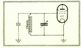
Fig. 1.—The usual method of connecting frame. By the capacity of the top end to earth (shown dotted) it acts also as an elevated aerial.
