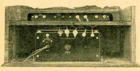
Back view of cabinet showing eliminator and H.T. and L.T. connections.
