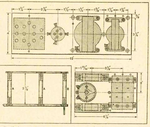
Fig. 12.—Layout of parts on the eliminator base and sub-stage showing method of mounting ebonite supports. The metal-cased 2 mfd. condensers on the sub-stage are held down by the moulded 1 mfd. condensers.
