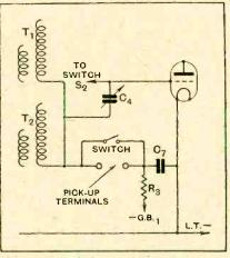
Fig. 1.— Modlfying the "S.G, Regional Receiver" for gramophone amplification. Reference lettering corresponds to the original diagram.
