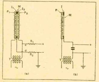
Fig. 1.—Diagrammatic cross-sections of the new differential and carlier single-acting Vogt electrostatic loud speakers. as simple as its external appearance would suggest. It consists, as shown diagrammatically in Fig. I (a), of the two plates  $P_1$  and  $P_2$ , both of which are perforated with large holes. Between them is stretched a very thin metal foil M, which serves as the diaphragm, and
