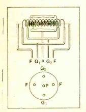
Fig. 1.—A double-grid valve and base. A straight filament is used around which there are two spiral grids and a cylindrical plate.
