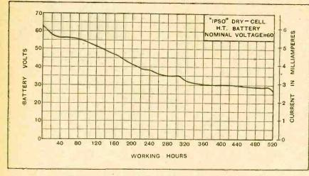
Discharge curve of the " Ipso " 60-volt dry-cell battery.
