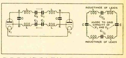
Fig. 20.—Circuit of Fig. 19 simplified by redrawing and omitting the connection from the junction of  $C_2C_2$  and of  $C_1C_1$  to the common filament lead. A B E D is an oscillatory circuit of supersonic (requency.
