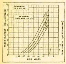
Average values under working conditions :— A.C. resistance, 11,700 ohms; amplification factor, 11; mutual conductance, 0.94 mA volt. amplification purposes a grid bias of -6 volts will be required under these conditions. The specimen tested exhibited slightly better characteristics than the maker's rating. Measured at 100 volts H.T. and zero grid bias, the A.C. resistance was found to be 10,000 ohms, the amplification factor 10, and the mutual conductance 1.0 mA. per volt.
