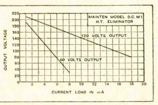
Voltage regulation curves of the D.C.M.1 model. Measurements were made of each output voltage under load separately.
