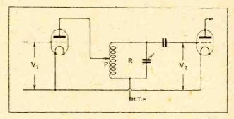
Fig. 5.—Here the amplification attained is variable within wide limits by changing the tapping point P. There is an optimum position for P.
