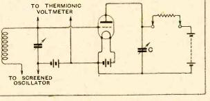
Fig. 1.-Connections for measuring the input load of the detector.
