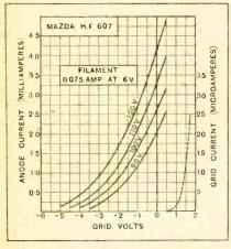
Average values under amplifying conditions: A.C. resistance, 19,000 ohms; amplification lactor, 18.2; mutual conductance, 0.96 mA. per volt.
