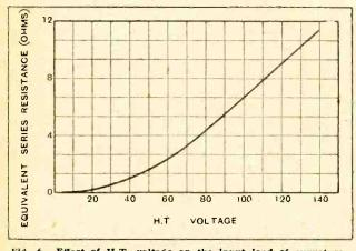
Fig. 6.—Effect of H.T. voltage on the input load of curvature detector. External anode resistance 60,000 ohms; added shunt capacity 135 micromicrofarads; wavelength 240 metres.
