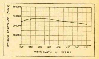
Fig. 3.—It will be seen from this curve that the dynamic resistance is approximately constant for the 200-550-metre waveband.
