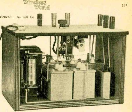
View of interior showing double-pole change-over switch.
