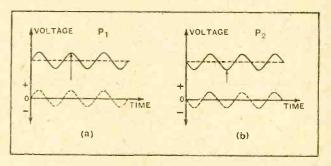
Fig. 2.—Curves representing the voltage conditions at the two outer plates of the Vogt differential loud speaker.
