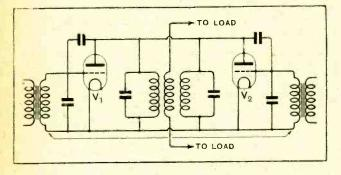
Fig. 23.—Showing that back-to-back valve circuits are equivalent to two paralleled tuned anodes.
