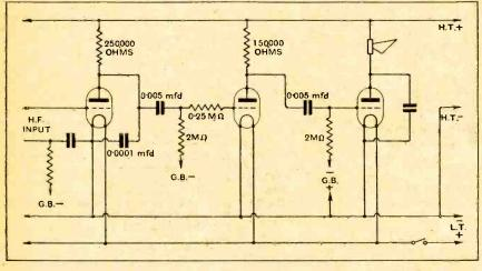
Fig. 2. Resistance-coupled L.F. amplifier for a portable receiver.
