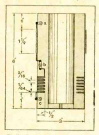
Fig. 6.—Sectional drawing of grid circuit coils. The short-wave winding consists of a single layer of 60 turns of 9/40 Litz and each slot of the longwave coil contains 35 turns of No. 32 D.S.C.
