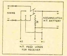
Fig. 1.—Switching scheme for connecting mains in series with H.T. accumulators for output valves.
