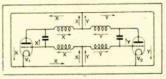
Fig. 24.-Showing "parallel" parasitic circuits in back-to-back amplifier.
