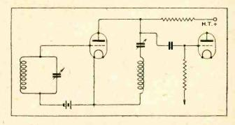
Fig. 13.—Series tuned circuit across external anode load to short-circuit virtually the H.F. component so that feed-back is eliminated. The low potential end of the coil can either be connected to L.T. negative (as shown) or to H.T. positive.
