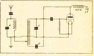
Fig. 4.—The same method of coupling applied to a "singlecoil Reinartz" circuit.
