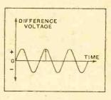
Fig. 3.—Resultant force on the diaphragm due to the alternating voltage applied to the two plates of the differential loud speaker.
