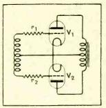
Fig. 25.—Diagram showing method of curbing parasitic oscillations in pushpull circuit.  $r_1 r_2$  are resistances to damp out parasitic oscillations of the twotypes described in the text.
