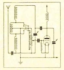
Fig. 1. H.F. potentiometer connected in a modified Hartley circuit.
