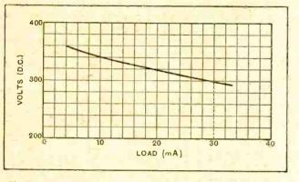
Fig. 5.-Regulation curve of Met-Vick combined "A" and "B" transformer and S.P. 42/U valve.
