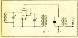
Fig. 6 .- Triple-grid valve as frequency-changer.
