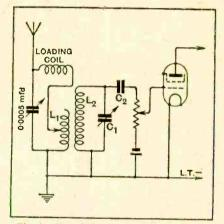
Fig. 1.—Tuned auto-coupled aerial circuit for the "Megavox" receiver.
