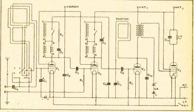
Portable receiver circuit with two screen grid stages and pentole. C<sub>1</sub>, C<sub>2</sub>, 0.0005 mfd.; C<sub>3</sub>, 0.0001 mfd.; C<sub>1</sub>, 0.0002 mfd.; C<sub>5</sub>, 0.0005 mfd.; C<sub>3</sub>, 0.0003 mfd.; C<sub>7</sub>, 0.0001 mfd.; C<sub>8</sub>, 0.003 m/d. or larger; C<sub>3</sub>, 2 mfls.; C<sub>10</sub>, G<sub>11</sub>, 0.002 mfd.
