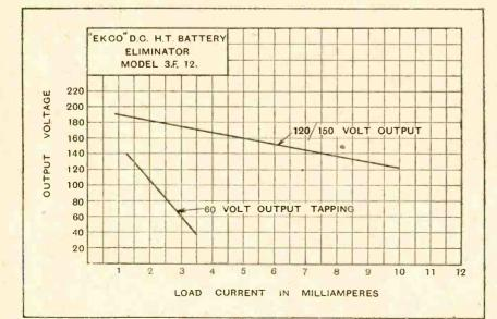
Voltage regulation curves for EKCO D.C. battery eliminator.
