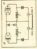
Fig. 15.—Diagram showing arrangement of output circuit when two magnetically separate but mechanically coupled high - resistance coils are used. teristics, each valve supplies one-half of the total electrical output to the loud speaker.
