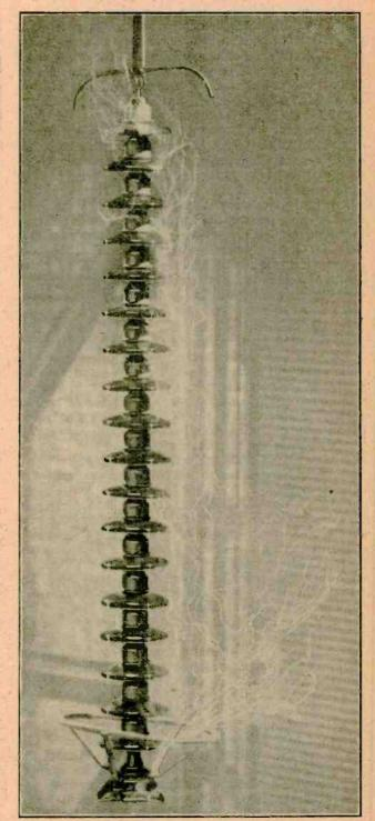
Fig. 3.—Photograph of an electrical discharge over a string of insulators about 7 feet long, with an applied pressure of about one million volts.
