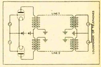
Fig. 12.—Diagram showing scheme of Fig. 11 applied to distant operation of reproducing apparatus.
