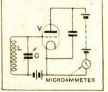
Fig. 3.—In this circuit a decapped valve V is used as an anode-bend detector. It had been calibrated as a voltmeter; the deflection of the instrument in the plate circuit for any H.F. voltage on the grid of the valve being known. The dynamic resistances given in the text apply to the above circuit as a whole.
