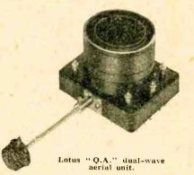
The device consists of two coils mounted concentrically, the inner being wound on a 2in. former and the outer on a 23in. former. For medium-wavelengths the two coils are connected in parallel, and for long-wave reception a series arrangement is adopted. These changes are made by a switch housed in the hollow base. The switch has an extension on the spindle to provide a means of "ganging" two or more units, so that one operation of the control knob will change over a number of units.
