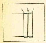
Fig. 13.—Diagram showing arrangement of mechanically coupled coils with small electromagnetic coupling.
