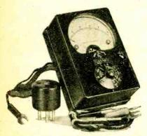
This Ferranti valve tester is actually reight instruments in one.
