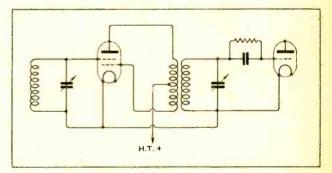
Fig. 3.-" Isodyne " circuit for high-frequency amplification.
