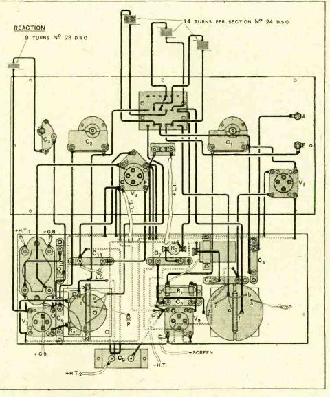
Practical wiring diagram. The leads are taken by the shortest path between the components on panel and baseboard. Leads beneath the baseboard are shown dotted and do not run by the paths indicated but by the shortest route from point to point.
