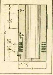
Fig. 10.—Sectional drawing of grid circuit coils. The short-wave winding consists of a single layer of 60 turns of 9/40 Litz and each slot of the long-wave coil contains 35 turns of No. 32 D.S.C.
