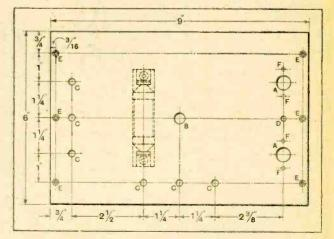
Fig. 2.—Layout of ebonite panel. Drilling sizes are as follows: A, in. diameter. B, in. diameter. C, in. diameter. D, in. diameter. E, in. diameter and countersunk for No. 4 wood screws. F, drilled and tapped 6 B.A. blind,
