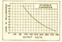
Voltage regulation curve from H.T. + 2 socket with vibrator adjusting lever at "maximum" setting.
