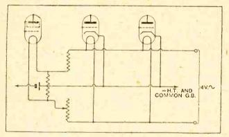
Schematic diagram of A.C. filament circuit.
