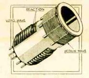
Fig. 2.—Construction of the anode coil assembly. The longwave section is cut away to show pile windings.
