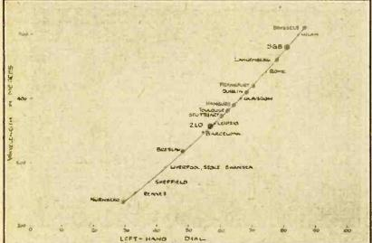
Fig. 15.—Calibration chart for the lower wave band made during a test at a place 20 miles north of London. Stations marked with one or more circles were enjoyed at full loud speaker strength withour interference.
