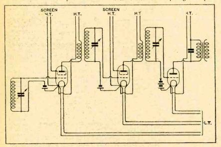
Fig. 2,—Individual feeds for each anode and screening-grid circuit, combined with non-inductive grid connections: scientific wiring as applied to a set with two screen-grid II.F. valves.
