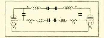
Fig. 26.—Showing circuital position of damping resistances  $r_1$ ,  $r_2$  of Fig. 25 for curbing parasitic mode of Fig. 20. Clearly resistances inserted at X and Y would also be effective. At high frequencies this is permissible since the resistance required is small, but at low frequencies it is large and would reduce the anothe feed.
