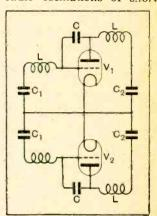
Fig. 19.—Circuit of Fig. 18 as it would appear so far as a parasitic oscillation of supersonic frequency is concerned. See Fig. 18 for meaning of symbols.
