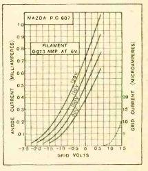
Average values under amplifying conditions; A.C. resistance, 75,000 obms; amplification factor, 40; mutual conductance, 0.53 mA. per volt.
