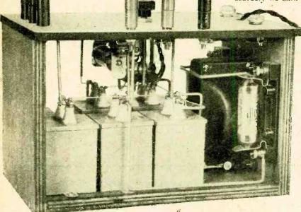
View of interior. The terminals at the left-hand side are for the connection of aerial, the aerial connection to set and the earth.
