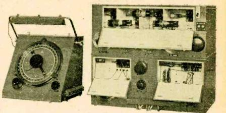
THE LATEST DIRECTION FINDER. New D.F. equipment specially designed for naval work by the Marconi Company's research department. On the left is the radio-goniometer. The amplifier and tuner are combined in a single unit.
