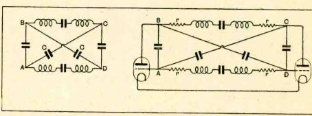
Fig. 28.—Showing additional circuits ABC, ACD, ABD, BCD introduced hy neutrodyne condensers CC of Fig. 27.
