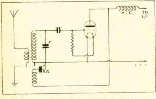
Fig. 1.- A conventional detector circuit with capacity-controlled reaction.
