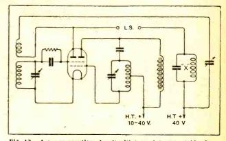
Fi 2. 12.—A super-reaction circuit with two-plate, two-The tuned circuit X is a trap circuit tuned to the frequency. -A super-reaction circuit with two-plate, two-grid valve,
