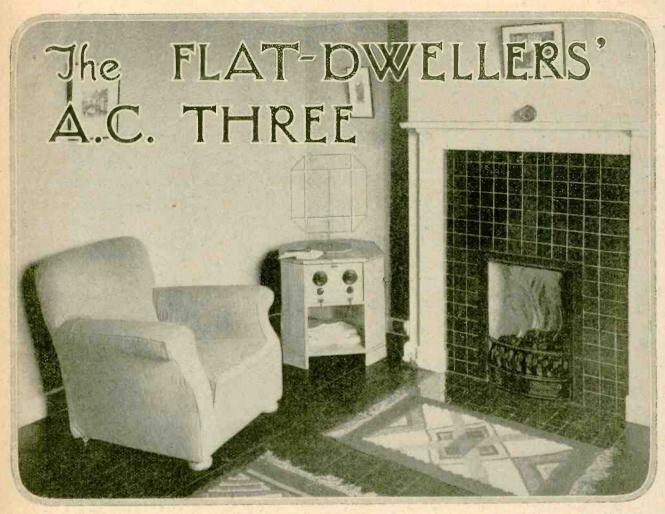
A Self=contained Frame Aerial Set Employing the New AC/S Screen=grid Valve. By F. L. DEVEREUX, B.Sc.
