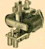
Baker's trigger release for use in building a picture receiver.
