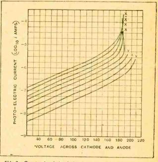
Fig. 2.—Curves showing relation between photo-electric current and anode-cathode voltage for various light intensities falling on the cell.
