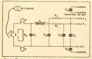
Fig. 1.—The theoretical circuit diagram. Values are as follows: C<sub>1</sub>, C<sub>2</sub>, C<sub>1</sub>, C<sub>4</sub> and C<sub>5</sub>, 4 mfds.; C<sub>5</sub>, 1 mfd.; L, 30 henrys: F, 3.5-volt flash-lamp bulb;  $R_1$ ,  $R_2$ , according to mains voltage and valves used;  $R_3$ , 40,000 ohms.
