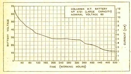
Discharge curve of the Columbia Type No. 4721 dry-cell H.T. battery.
