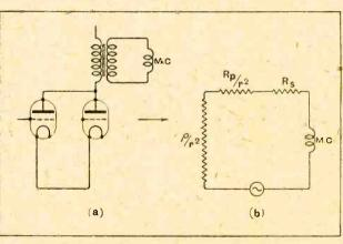
Fig. 1.—The output stage and its equivalent impedances.  $\rho =$  valve impedance, r = transformer ratio,  $\mathbf{R}_p =$  resistance of primary,  $\mathbf{R}_g =$  resistance of secondary.
