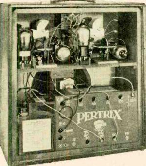
This view shows the arrangement of the batteries.
