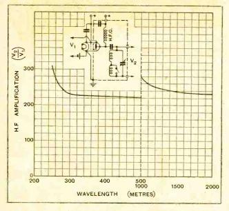
Fig. 2.—Amplification curves of the AC/S valve with parallel feed, tuned grid coupling; H.T.= 120 volts, screen-grid=48 volts, G.B.= — 1 $\frac{1}{2}$  volt. The measurements were made with a Lewcos H.F. choke, a 0.0002 mfd. coupling condenser and the coils shown in Fig. 6.
