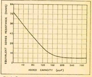
Fig. 4.—Gurve representing the effect of capacity across the primary of an L.F. transformer on the equivalent series input resistance of the detector. With 0.0001 mfd. across the transformer primary there is a load equivalent to about 30 ohms added to the tuning coil.
