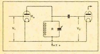
Fig. 4.—In this tuned anode circuit the overall amplification  $V_2/V_1 = \frac{\mu R}{R+R_0}$
