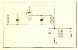
Fig. 2.—Standard frequency-changing circuit for double-grid valve.
