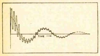
Fig. 10.—Diagram illustrating combination or superposition of the main diaphragm and reed oscillations of Figs. 8 and 9.
