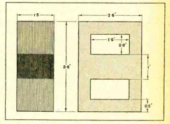
Fig.2.-Transformer section giving dimensions.
