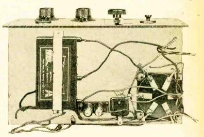
Components mounted on under-side of baseboard.
