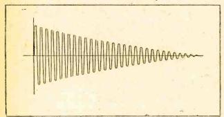
Fig. 9.—Showing higher frequency (damped) oscillation due to the reed plus part of the diaphragm.
