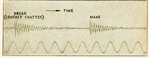
Fig. 16.—Acoustic output from desk type telephone with 2 inch stalloy diaphragm due to square-topped waveform. Break is marred for about three complete oscillations due to the relay contact chattering. Note that the oscillation persists practically the whole interval between make and break, i.e. 0.03 second. The frequency is about 1,000 cycles.
