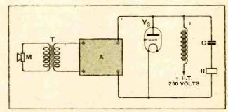
Fig. 12,—Diagram showing circuit arrangement of amplifier for Fig. 11.
