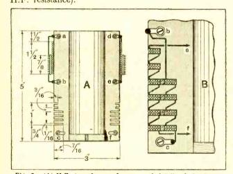
Fig. 3.—(A) H.F. transformer former and details of short-wave windings. (B) Enlarged section showing winding of long-wave transformer. Lettering of terminal points corresponds with that in other diagrams.
