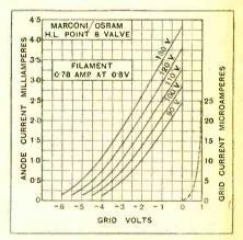
Average values under working conditions: A.C. resistance, 22,200 ohms; amplification factor, 16.6; mutual conductance, 0.75 mA./v.
