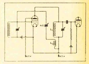
Fig. 2.—Here  $L_2$  is a two-turn coil coupled to  $L_1$ . The voltage induced in it is so small that neutralisation can be attained while still employing an ordinary neutrodyne condenser in the position N.C. Both here and in Fig. 1 the tuned-anode circuit is shown for the sake of simplicity; in practice an equivalent transformer could be used.
