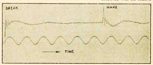
Fig. 19.—As in Fig. 15, but loud speaker in room without draping. The higher frequency components are now more prominent.
