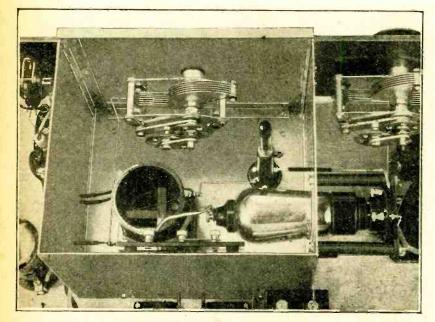
Interior of screening box showing the switch-over arrangement for using either screen-grid or triode vatve.
