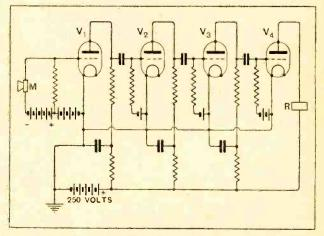
Fig. 6.—Circuital arrangement of microphone and its associated amplifier.  $V_1,\ V_2,\ V_3=LS5B$  valves,  $V_4=LS5A$  R - recorder, M= microphone.
