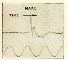
Fig. 13. — Acoustic output from transformer-coupled moving coil loud speaker with 55 turns 2 inches diameter. Diameter of cone 9½ inches. There is a low-frequency oscillation of 120 cycles due to the first "mode" of the diaphragm, and a high-frequency oscillation of 2,000 cycles. There is no oscillation of the diaphragm as a whole on its support.
