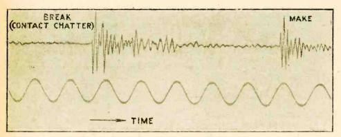
Fig. 18.—Acoustic output from experimental reed-orive with conical diaphragm 2 inches in diameter with flat circular paper surround 1½ inches wide. There appear to be two oscie ations superposed having frequencies of 1,000 and 500 cycles respectively. The damping is relatively small. The first three oscillations at break are marred by a chattering relay contact.
