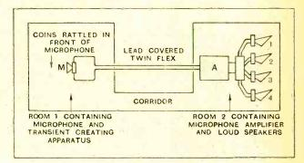
Fig. 3.—Diagram illustrating layout of apparatus for experiments on the reproduction of transients due to rattling of coins or ringing of electric bell.
