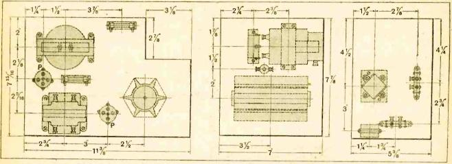
Fig. 7.—Disposition of components on baseboard and platform: under the latter are mounted condensers C<sub>1</sub>, C<sub>2</sub>, C<sub>3</sub>, C<sub>4</sub>, and decoupling resistance R<sub>2</sub>, in relative positions as shown in Fig. 8.
