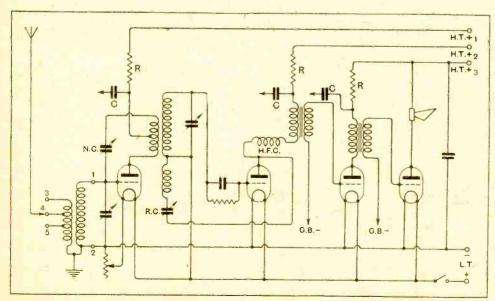
Fig. 1.—Theoretical circuit diagram, simplified by omission of waveband switch and output jack.
