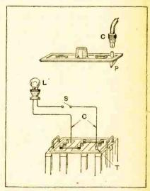
An acid-level indicator for accumulators with opaque containers.
