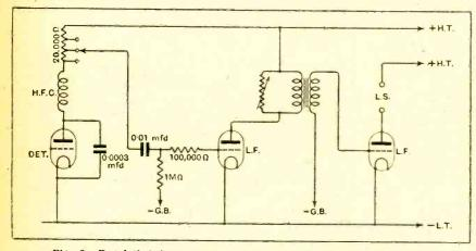
Fig. 2.—Regulating input to first and second L.F. amplifying valves.
