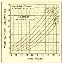
Average values under working conditions: A.C. resistance, 5,700 ohms; amplification factor, 6.6; mutual conductance, 1.15 mA./v.
