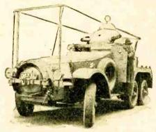
ARMOURED CAR WIRELESS. A new type of car designed for patrol work on rough roads in India. The wireless trans-mitter and receiver can be operated on the move.
