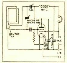
Fig. 1.—Circuit diagram of four-electrode valve portable set with semi-variable anode by-pass condenser.
