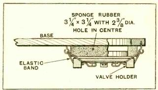
Fig. 5.—Sectional sketch showing shock-absorbing mounting for multiple valve holder.
