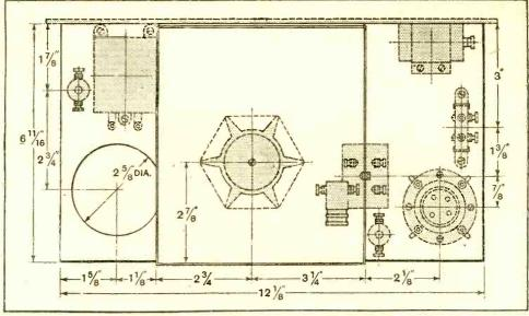
Fig. 4.-Layout of components on the baseboard, which is of plywood, in. thick.
