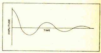
Fig. 8.—Diagram showing a damped sine wave. This corresponds roughly to the main lower frequency oscillation of the loud speaker.
