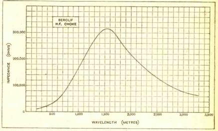
Impedance curve of Berclif H.F. choke; external capacity 8 mlcro-mfd.
