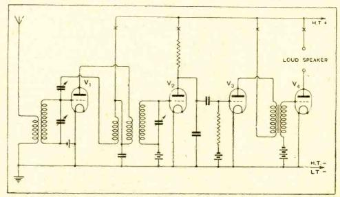
Fig. 1.—In a receiver such as this the plate currents might be as follows:  $V_1 = 3$  mA.;  $V_2 = \frac{1}{2}$  mA. or less, depending on signal strength;  $V_3 = 5$  mA., and  $V_4 = 18$  mA.
