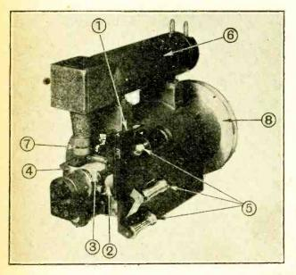
Fig. 4.—The sound projector. Reference numbers correspond with those in Fig. 3.
