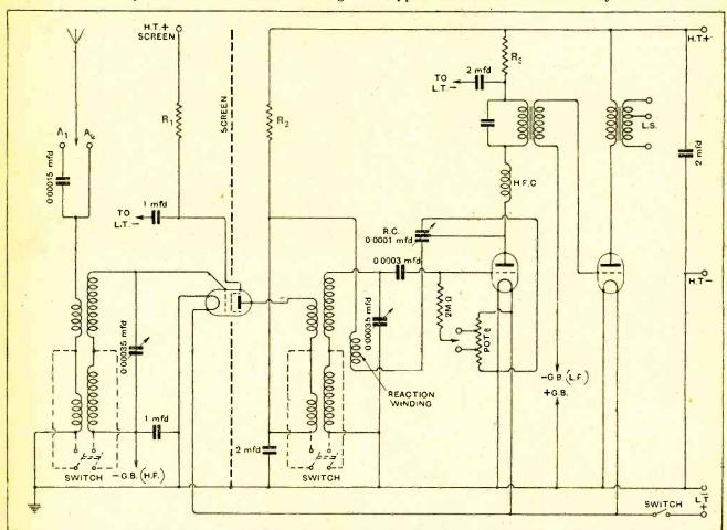
Fig. 2.—Complete circuit diagram. Wiring of wave-changing switches is shown in dotted lines. The by-pass condensers associated with grid and screen circuits of the H.F. valve are actually in the form of a single component with three terminals.
