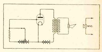
Fig. 14.—Arrangement of valve (L.S.5A.) and loud speaker for obtaining the record of Fig. 13.
