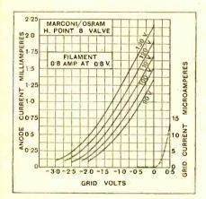
Average values under working conditions: A.C. resistance, 57,500 ohms; amplification factor, 44.5; mutual conductance,  $0_s/78$  mA./v.
