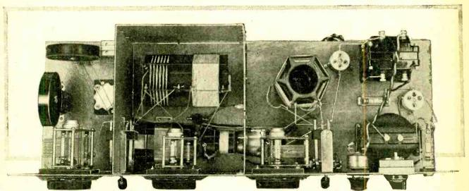
Plan view of receiver. Single bias cell for H.F. valve and by-pass condenser C, are secured to the baseboard by light metal clips.
