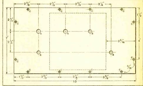
Fig. 2.—Drilling details of the front panel. Position of screening box, mounted behind it, is shown in dotted lines. A, i in. dia.; B, in. dia.; C, in. dia.; C,
