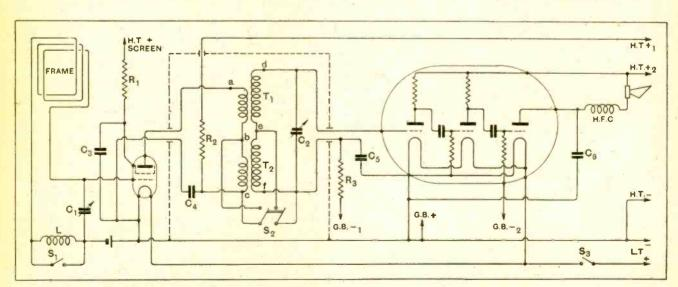
Fig. 1.—Circuit diagram.  $R_1$ ,  $R_2$ ,  $R_3$ , decoupling resistances, 600 ohms.;  $C_1$ ,  $C_2$ , tuning condensers, 0.0003 mfd.;  $C_3$ ,  $C_4$ ,  $C_5$ , hy-pass condensers, 0.1 mfd.;  $C_6$ , 0,002 mfd.;  $C_7$ , short-wave H.F. transformer;  $C_7$ , long-wave H.F. transformer;  $C_7$ , wave-changing switches;  $C_7$ , on-off switch;  $C_7$ , long-wave loading coil.
