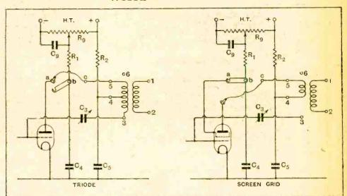
Simple switch-over scheme permitting the use of either triode or screen-grid valves. Should the same H.F. transformer be used with the screen-grid valve as with the triode, small yet probably adequate amplification will result. If a neutralising winding connects to pin 3 with the screen-grid valve then C<sub>3</sub> must be set to zero.
