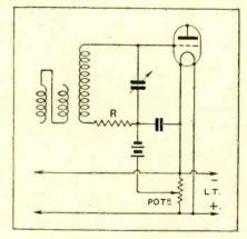
.—Position of artificial resistance (R) in an oscillatory circuit.
