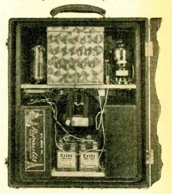
Rear view of receiver. The loud speaker is mounted above the L.T. battery.
