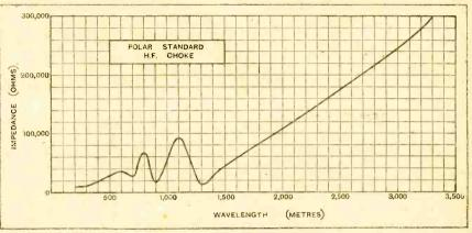
Impedance curve of Polar Standard H.F. choke; external capacity 8 micro-mfd.
