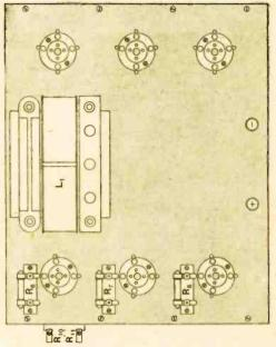
Plan view showing the location of components for assembly. By precisely tollowing this tayout the wiring up may be effected by short leads. The reference letters are those used in the circuit diagram.
