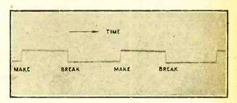
Fig. 4.—Diagram showing waveform of transient applied to loud speaker. Actually this is the waveform of the e.m.f. applied to the grid of the LS5A power valve in whose anode circuit the loud speaker was situated.
