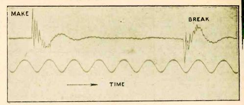
Fig. 17.—Acoustic output from experimental reed-driven loud speaker with large conical diaphragm. The main diaphragm oscillation persists for about two oscillations. Its frequency is about 100 cycles. The higher frequency is about 2,000 cyc.es.
