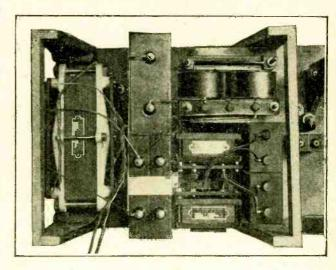
Fig. 3.—The eliminator wired ready for securing the valve platform.
