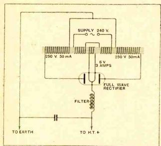
Fig. 4.—Transformer for supplying smoothed high-tension current. Note that the primary and secondary are split.
