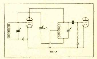
Fig. 1.—Neutralisation of a tuned-anode circuit in this or a similar manner is perfectly sultable for a three-electrode valve, with which it is shown, but not for a screen-grid valve. Neutralisation takes place when the balancing condenser N.C. is set to the same value as the interelectrode capacity of the valve, and this capacity, in the case of a screen-grid valve, is far below the minimum of any neutralising condenser.
