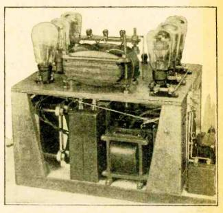
Fig. 5.—The eliminator section. For D.C. supply the three output valves together with the output choke and condenser are accommodated on the baseboard. High voltage D.C. is best obtained by means of an accumulator pattery connected in series with the maias.
