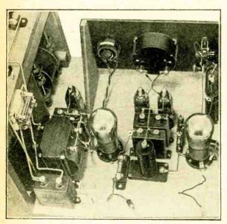
Fig. 2.—The arrangement of the components provides for easy wiring. This view shows the layout of the apparatus associated with the detector and first L.F. amplifier.
