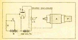
Fig. 5.—Diagram illustrating disposition of apparatus for applying equare topped transient to loud speaker, and obtaining a record of the resulting acoustic waveform on the axis of the speaker. R = non-inductive high resistance, B = grid bias battery. The blas voltage is reduced when the relay contacts C are closed. L.S. = speaker under examination, M = microphone, A = resistance-capacity microphone amplifier fed direct to P the recorder.
