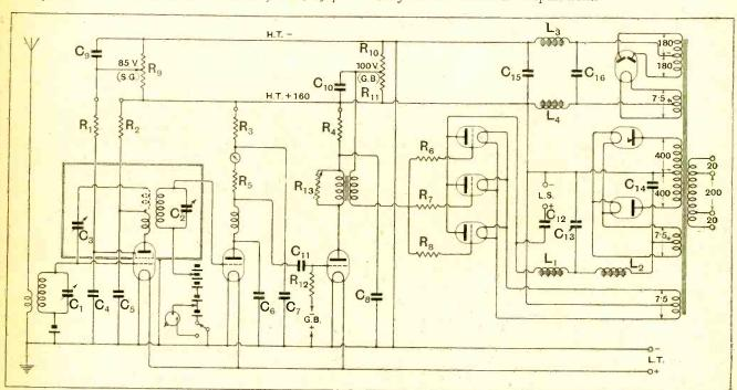
The complete circuit diagram showing the battery eliminator equipment for A.C. supply as well as the complete receiver.  $C_1$ ,  $C_2$ , 0.0003 mid.;  $C_3$ , neutralising condenser;  $C_4$ ,  $C_5$ , 0.01 mid.;  $C_6$ , 0.0002 mid.;  $C_7$ ,  $C_8$ ,  $C_{10}$
