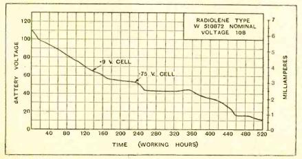
Discharge curve of Radiolene 108 volts dry-cell battery.
