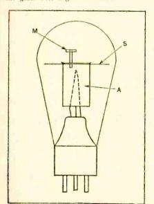
To facilitate free heat-radiation in a rectifying valve a mica screen S is inserted.
