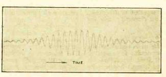
Fig. 1.—Diagram illustrating a simple transient. The frequency of the oscillation is 600 cycles for second. The waveform is that of the growth and decay of the natural oscillation of a simple tuned circuit consisting of an inductance, resistance and condenser as shown.
