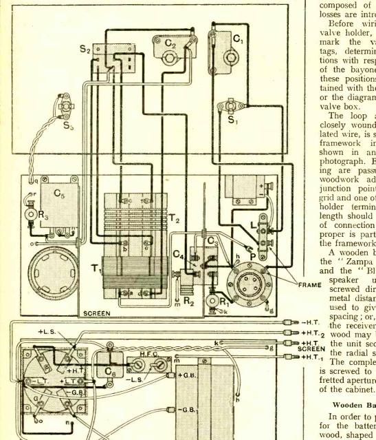
>+L.T. Fig. 6.—Practical wiring plan. Leads passing through baseboard may be traced by observing the corresponding lettering. Points of attachment for loud speaker and frame aerial are shown. Extra earthing leads are taken from rear lower edge of screening box and from metal loud speaker frame to L.T.—terminal.
