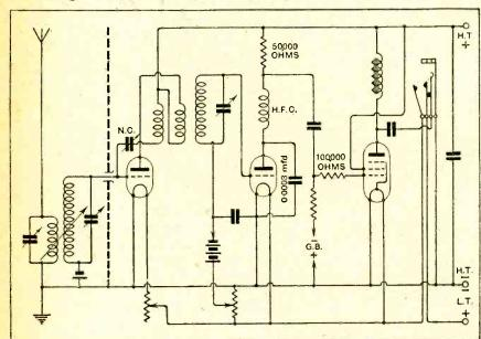
Fig. 2 .- "Regional Three" receiver with pentode output valve.
