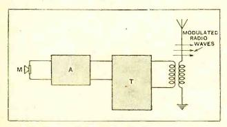
Fig. 2.—Diagram illustrating broadly how sound waves are ultimately converted into radio waves. M = microphone, A = microphone amplifier, T = radio-broadcasting transmitter.
