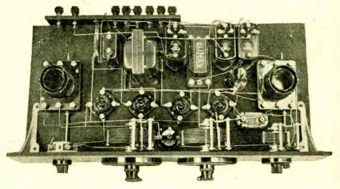
Plan view of the receiver. The neutralising condenser is mounted between the tuning condensers.
