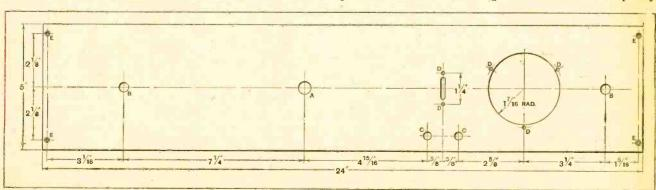
Fig. 1.—Drilling details of the panel. A, ½in.; B, ½in.; C, ½in.; D, ½in.; E, ½in., and countersunk for No. 4 wood screws. Thickness ½in.
