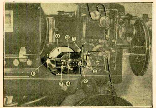
Fig. 3.—Cinema projector with sound-projecting apparatus fitted. Reference numbers are expl. in the text.
