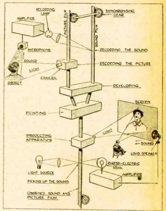
Fig. 2.—Simplified diagrammatic sketch, showing method of recording and projecting "Tobis" films.
