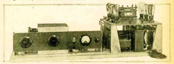
The complete receiver with eliminator for use on A.C. supply. A separate rectifier provides the anode voltage for the first three valves and this potential serves to bias the output stage.
