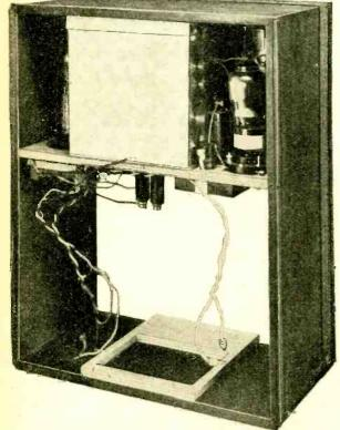
Another view showing framework removed from case. Note frame aerial winding and wooden block for retaining batteries in position.
