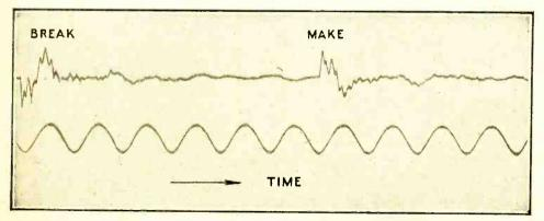
Fig. 7.—Acoustic output from "Kone" loud speaker when supplied with square-top input.
