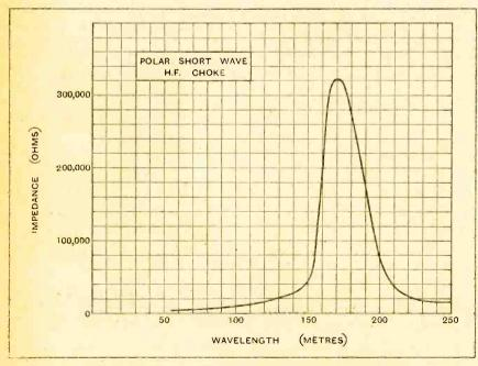
impedance curve of Polar Short Wave H.F. choke; external capacity 8 micro-mfd.
